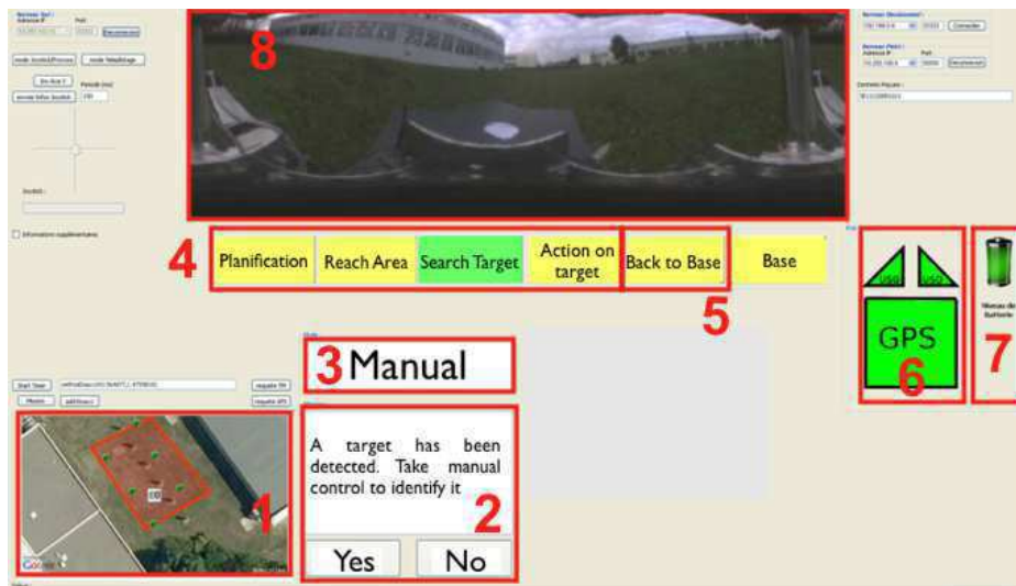
Figure 6.1: Eight Areas Of Interest (AOIs) are defined on the GUI as follows: 1) tactical map, 2) interactive panel, 3) piloting mode, 4) synoptic, 5) back to base, 6) GPS and ultrasound status, 7) battery status, and 8) panoramic video.
