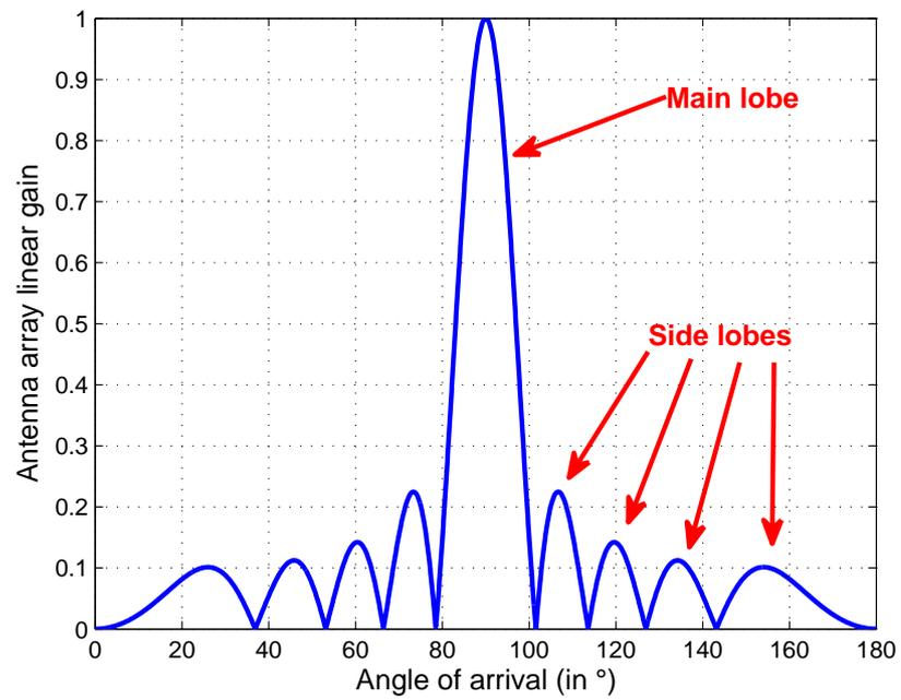
Figure 3.1: Directivity diagram of a 10-antenna Uniform Linear Array (ULA), with  $\frac{\lambda}{2}$  spacing, beamforming in the direction  $90^\circ$ . The main lobe is centered at  $90^\circ$  with unitary maximum gain.
