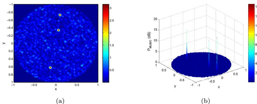
Figure 4.10: MULTIPLE SIGNAL CLASSIFICATION. Skymaps are given in dB. (a) Simulated skymap with three interferences impinging a 48-antenna array,  $\text{INR} = 0$  dB. (b) MUSIC spatial skymap (contrast function) showing three peaks corresponding to the three interference signals directions of arrival.
