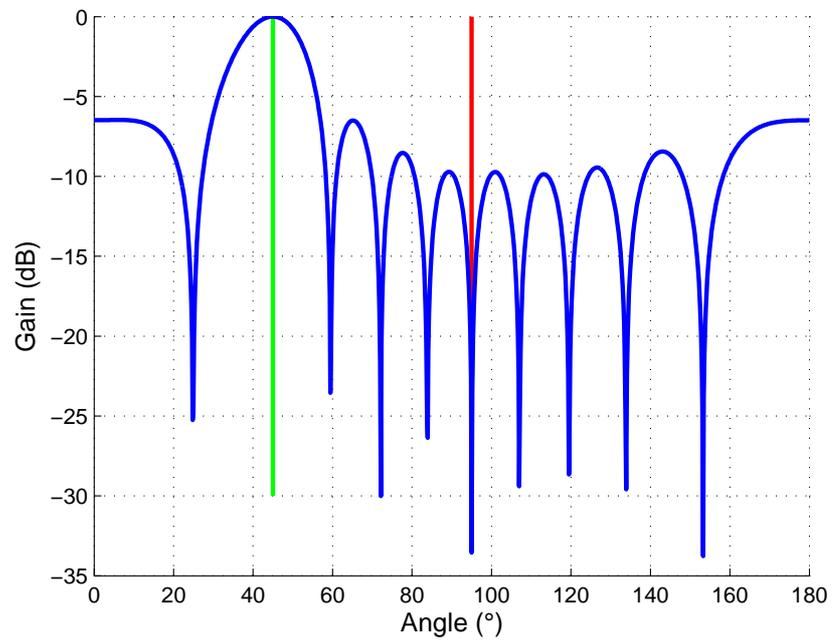
Figure 3.7: Directivity pattern obtained with a LCMV beamformer. Computed using a simulated uniform linear antenna array made of 10 antennas with  $\frac{\lambda}{2}$  spacing. One signal of interest, One interference, SNR = 0 dB, INR = 0 dB. The green line corresponds to the signal of interest direction, the red line is the RFI direction.
