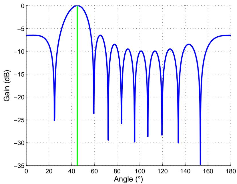
Figure 3.3: Directivity diagram obtained with a classical delay and sum beamformer. Computed using a simulated uniform linear antenna array made of 10 antennas with  $\frac{\lambda}{2}$  spacing. The green line corresponds to the signal of interest direction.
