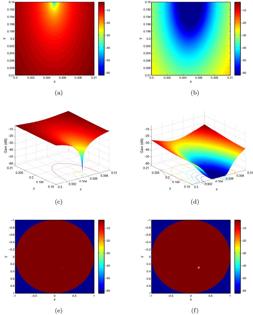
Figure 4.13: Multiple beam projection. Skymaps are given in dB. (a) Orthogonal projection based on a single steering vector. (b) Orthogonal projection based on the same steering vector as (a), by also rejecting 10 other directions of arrival located in a close neighborhood. (c) and (d) 3-dimensional representation of the map (a) and (b), respectively. (e) and (f) Global skymaps after the projection presented in (a) and (b), respectively.
