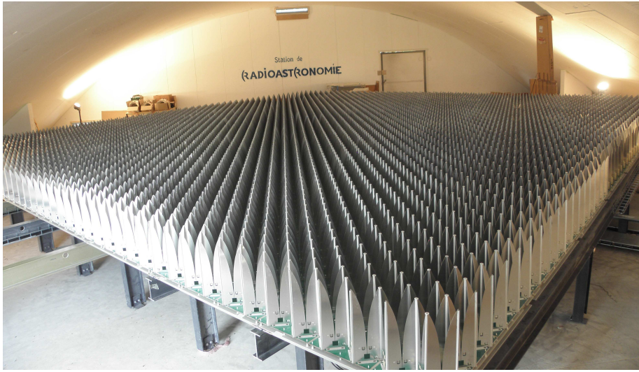
Figure 5.17: French EMBRACE station inside its radome, located at the Nançay observatory. Courtesy of Dr. Stephen Torchinsky.
