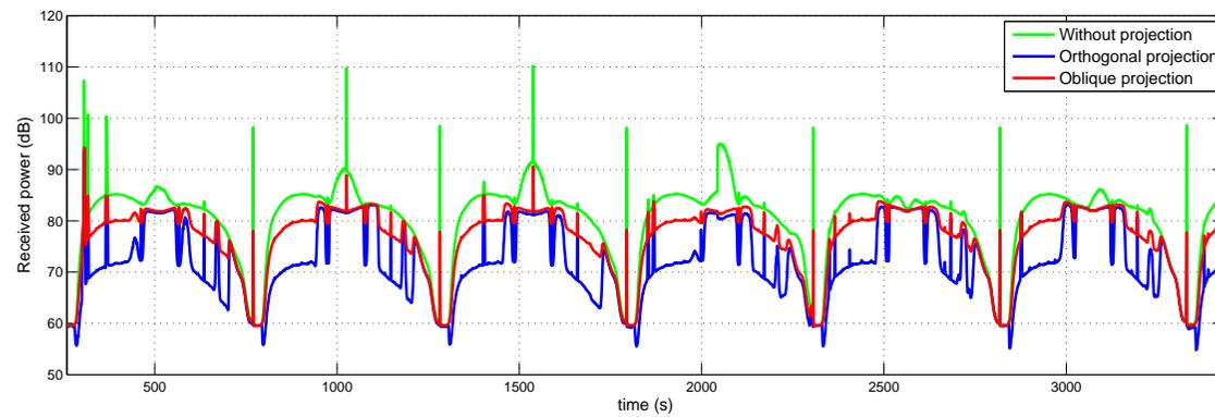
Figure 5.29: Orthogonal and oblique projections projecting a 1-dimensional RFI subspace. In green, the data recovered after beamforming in the direction of the center of the analog beam. In blue, the same results applying an orthogonal projection. In red, the same results applying an oblique projection. The interference subspace is estimated using the dominant singular vector of each crosslet.
