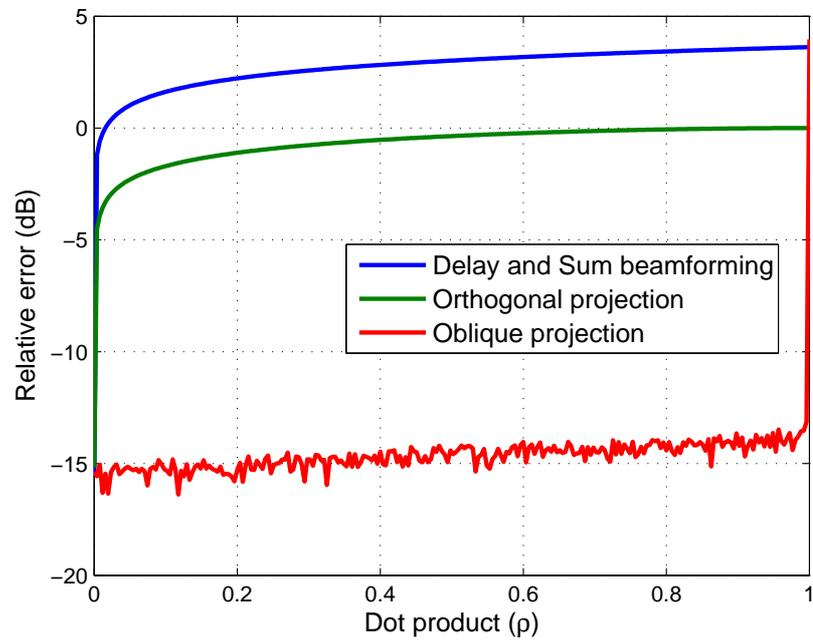
Figure 3.10: Relative error of the Delay and Sum beamforming, Orthogonal and Oblique projection beamforming techniques.  $M = 60$  randomly distributed antennas, noise-free model, one cosmic source (power =  $-5$  dB), one interference (Interference to Signal Ratio =  $+30$  dB), averaged over 512 trials.
