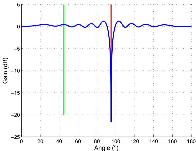
Figure 3.5: Directivity pattern obtained with a multiple sidelobe canceller beamformer. Computed using a simulated uniform linear antenna array made of 10 antennas with  $\frac{\lambda}{2}$  spacing. One antenna was used as a primary channel, the nine other antennas were used as the auxiliary sub-array. Covariance matrices calculated over 32768 samples. SNR = 0 dB. INR = 0 dB. The green line corresponds to the signal of interest direction, the red line is the RFI direction.
