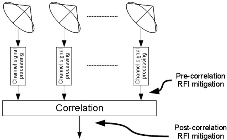
Figure 3.2: Antenna array radio telescope system. Signals acquired by antennas are pre-processed (subband filtering and frequency shifting), then correlated. Spatial RFI filtering can be applied either before or after the correlation process.
