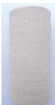
**Fig. II-3.** Cylindrical sample ( $\varnothing$  40 × 80 mm) of Richemont limestone.
