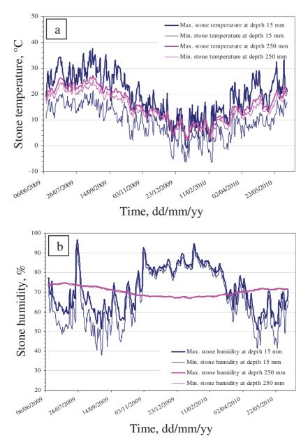
**Fig. II-23.** Daily maximum and minimum values of temperature (a) and relative humidity (b) at 15 and 250 mm depth, on the south wall for the period from June/2009 to June/2010.
