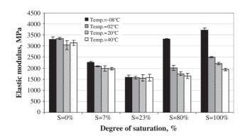
Fig. 5. Effect of water saturation on values of elastic modulus at different temperature.
