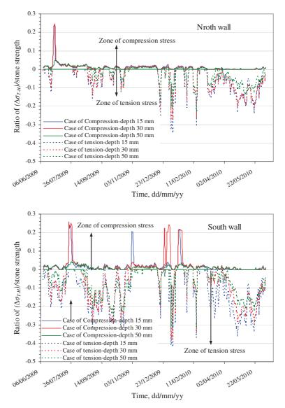
**Figure 12:** Proportion of compression, tension hygrothermal stresses to compressive, tensile stone strength at different depths inside the stone for the period from June 2009 to June 2010 on the north wall (left), and the south wall (right), **based on the adjusted stone humidity**
