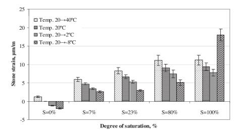
Fig. II-32. Effect of water saturation and temperature on stone strain values.
