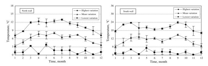
Fig. 5 Highest, mean and lowest daily variation in stone surface temperature for the period June 2009–June 2012
