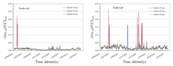
Figure 10: Proportion of daily variations in hygrothermal stresses to the minimum compression strength at different depths inside the stone for the period from June 2009 to June 2010 on both, north wall (left), and south wall (right), based on the adjusted stone humidity
