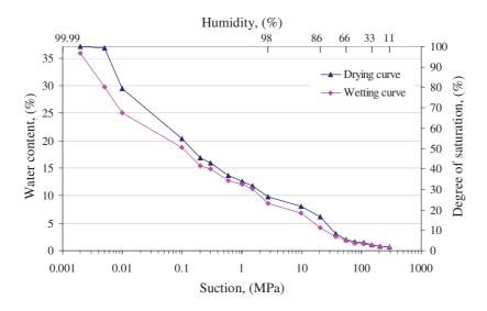
Fig. II-13. Water retention curve of tuffeau limestone (Beck, 2006).
