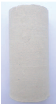
Fig. II-1. Cylindrical sample ( \text{Ø } 40 \times 80 \text{ mm} ) of tuffeau limestone.
