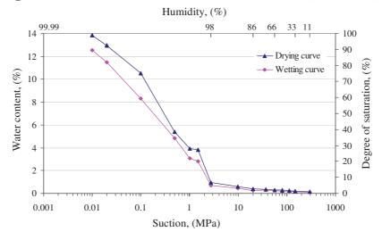
Fig. II-14. Water retention curve of Richemont stone.
