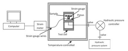
Fig. 2. Scheme of the layout of the experimental set-up.
