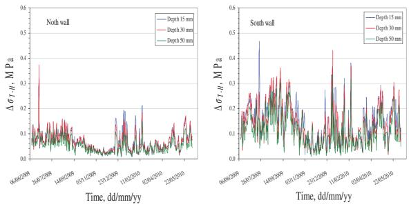
Figure 5: Daily variations in hygrothermal stresses at different depths inside the stone for the period from June 2009 to June 2010 on both, north wall (left), and south wall (right), based on the original stone humidity
