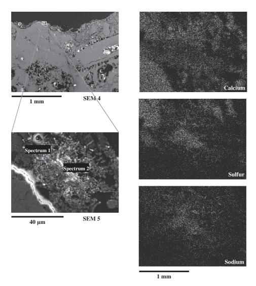
**Fig. III-20.** SEM images at different magnifications (SEM 4: ×50, SEM 5: ×1300) obtained from the sample BS-W (*left*); the elemental maps from the image SEM 5 (*right*).
