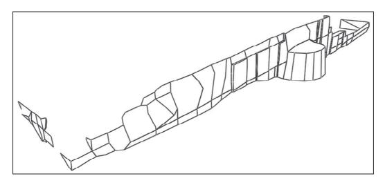
Fig. III-26. 3D wireframe model of Al-Ziggurat walls with its surfaces.
