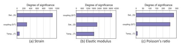
Fig. 8. Ranking the parameters in the form of the single or coupling effect on the measured response of (a) strain, (b) elastic modulus and (c) Poisson's ratio.
