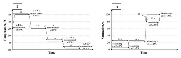
**Fig. 3.** Outline showing the stages followed in: (a) first experimental plan: strain, elastic modulus and Poisson's ratio measurements for the samples with different temperatures at constant water saturation, and (b) second experimental plan: strain measurements for the sample with different water saturation at constant temperature of 20 °C.
