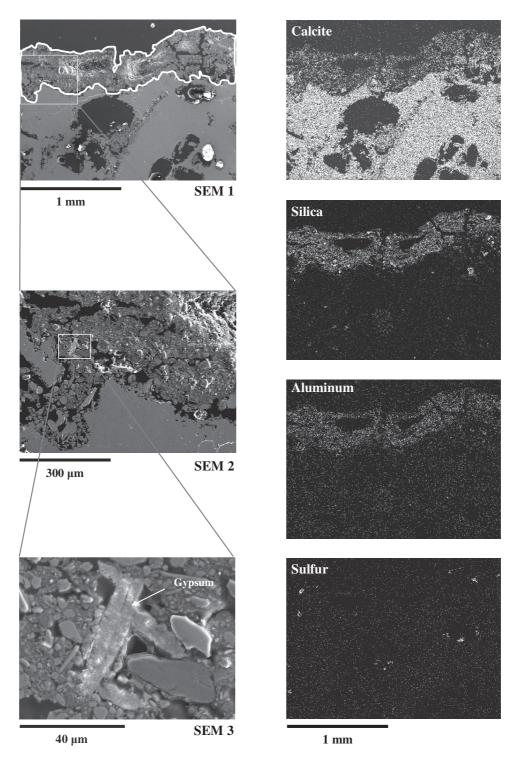
**Fig. III-19.** SEM images at different magnifications (SEM 1: ×50, SEM 2: ×150, SEM 3: ×1300) obtained from the sample BS-N (*left*); the elemental maps from the image SEM 1 (*right*).
