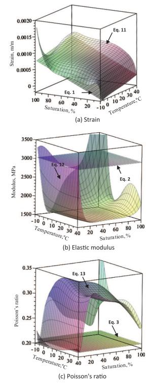
**Fig. 10.** 3D Graphical representation of the models of: (a) strain, (b) elastic modulus and (c) Poisson's ratio as a function of temperature and water saturation.
