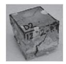
Fig. I-4. Different stone decay patterns due to salt weathering (sodium sulfate), fine crumbling at 5% salt concentration (*right*), coarse crumbling and contour scaling at 12% salt concentration (*left*).
