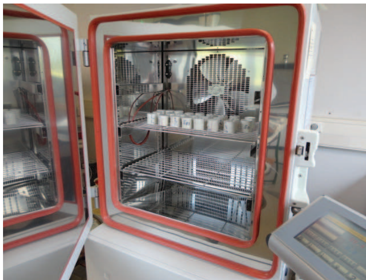
Fig. II-26. Schematic for one freezing-thawing cycle ( top ), general setting of the tested samples inside the freezing chamber ( bottom ).
