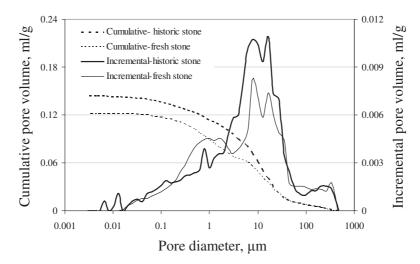
Fig. III-24. Analysis of mercury intrusion porosimetry test, pore size distribution for the two stones.
