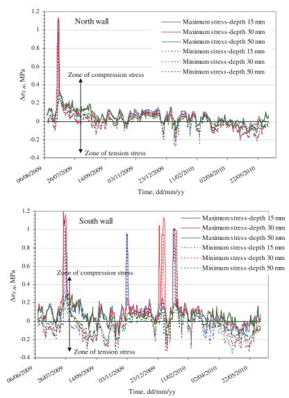
**Figure 8:** Maximum and minimum and tension hygrothermal stresses at different depths inside the stone for the period from June 2009 to June 2010 on the north wall (top) and the south wall (bottom), **based on the adjusted stone humidity**
