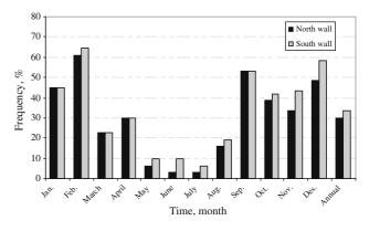
Fig. 6 Frequency of condensation events on stone surfaces of north and south walls
