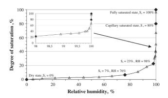
Fig. 1. Water retention curve of tuffeau [11,12].
