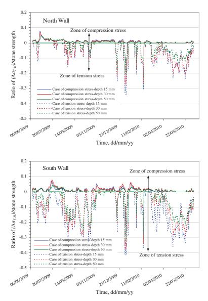
**Figure 11:** Proportion of compression, tension hygrothermal stresses to compressive, tensile stone strength at different depths inside the stone for the period from June 2009 to June 2010 on the north wall (top) and the south wall (bottom), **based on the original stone humidity**
