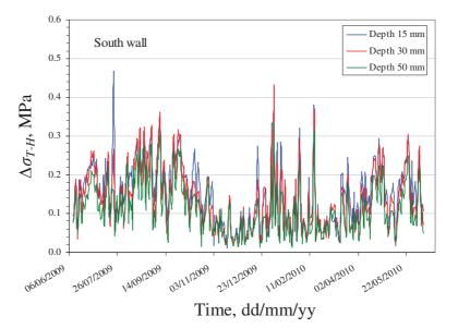
**Fig. II-36.** Daily variations in hygrothermal stresses at different depths inside the stone on the south wall for the period from June 2009 to June 2010.
