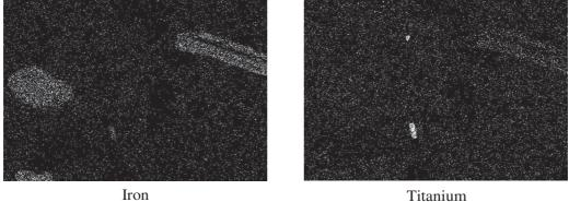
Fig. II-9. EDS maps showing the elemental compositions of Ca, Si, Al, Fe and Ti present in tuffeau limestone, (after Beck, 2006).
