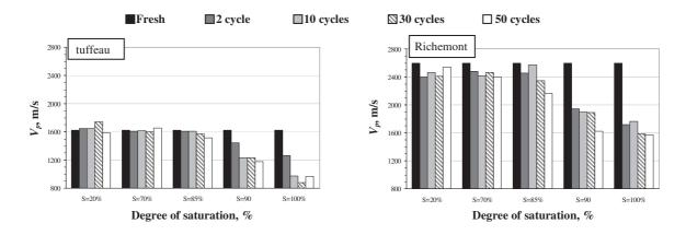
Fig. II-28. Ultrasonic pulse velocity for fresh and aged samples at different degrees of saturation, tuffeau and Richemont stone.
