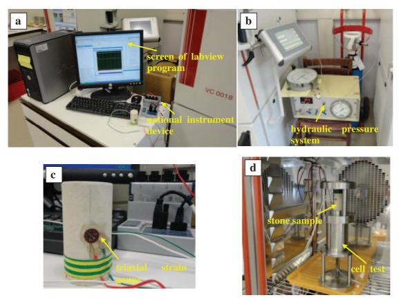
**Fig. II-30**. Photo showing the layout of the experimental set-up with the tools used: (a) data logger; (b) hydraulic pressure system; (c) strain gauge on the stone sample; (d) setting of the cell inside the climate chamber.
