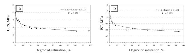
**Figure 4:** Correlation between degree of water saturation and Unconfined Compressive Strength, UCS (a), and Indirect Tensile strength, ITS (b), (Beck, 2006)
