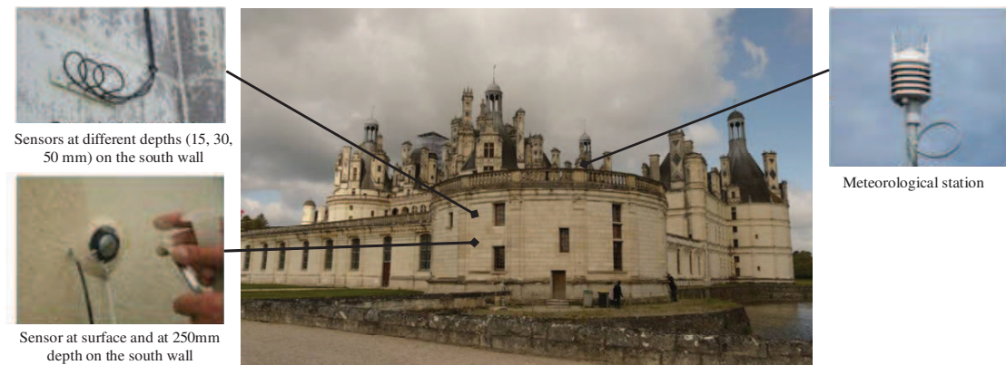
Fig. II-21. General view of the east tower of the castle of Chambord showing the thermal-humidity sensors ( left ), and the meteorological station ( right ).
