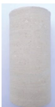
Fig. II-3. Cylindrical sample ( \varnothing 40 × 80 mm) of Richemont limestone.
