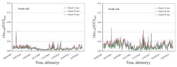
Figure 9: Proportion of daily variations in hygrothermal stresses to the minimum compression strength at different depths inside the stone for the period from June 2009 to June 2010 on both, north wall (left), and south wall (right), based on the original stone humidity
