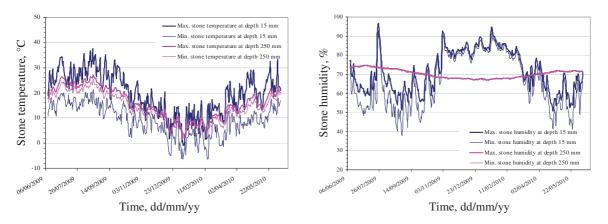
**Figure 2:** Daily maximum and minimum values of temperature (left) and relative humidity (right) at 15 and 250 mm depth, on the south wall for the period from June 2009June 2009 to June 2010
