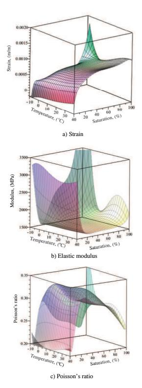
**Fig. II-35.** 3-D Graphical representations of the models of (a) strain; (b) elastic modulus; (c) Poisson's ratio as a function of water saturation and temperature.
