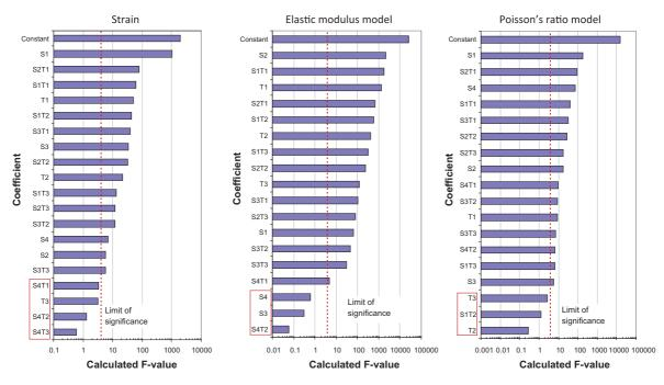
Fig. 7. Ranking the coefficients' significance for the three models.
