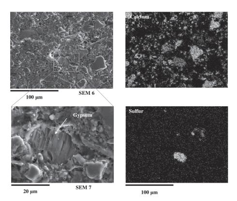
**Fig. III-21.** SEM images at different magnifications (SEM 6: ×500, SEM 7: ×2000) obtained from the soil sample (*left*); the elemental maps from the image SEM 6 (*right*).
