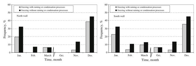
Fig. 9 Frequency of freezing events with or without effects of raining and condensation processes
