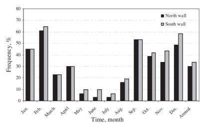
Fig. II-24. Frequency of condensation events on stone surfaces of the north and south walls.
