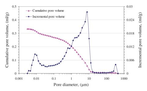
Fig. II-11. Pore size distribution of tuffeau limestone.
