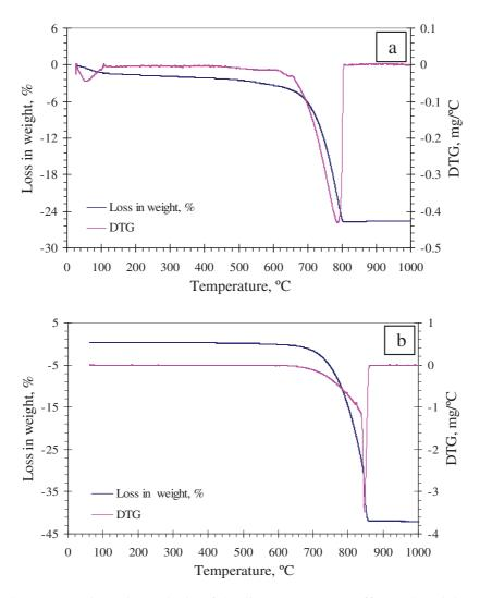
Fig. II-6. Thermo-gravimetric analysis of the limestones: (a) tuffeau; (b) Richemont stone.
