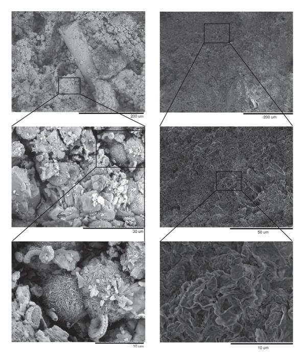
**Fig. II-7.** Rough surface SEM images showing the topography of the grains in the stones: (*left*) tuffeau: (*right*) Richemont stone.
