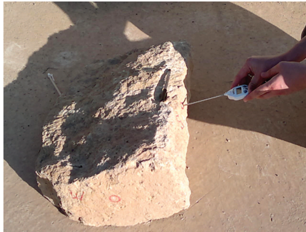
Fig. III-13. General setting showing the measurements of temperature for the large block of historic limestone for the period November/2012 - October/2013.
