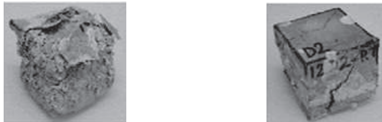
Fig. I-4. Different stone decay patterns due to salt weathering (sodium sulfate), fine crumbling at 5% salt concentration ( right ), coarse crumbling and contour scaling at 12% salt concentration ( left ).
