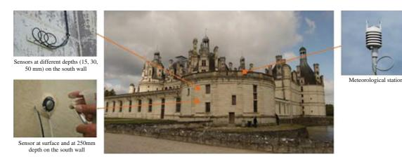
Fig. 3 The meteorological station above the east tower and the sensors positioned on the south wall
