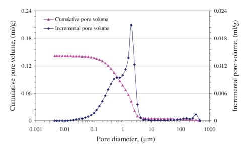
Fig. II-12. Pore size distribution of Richemont stone.
