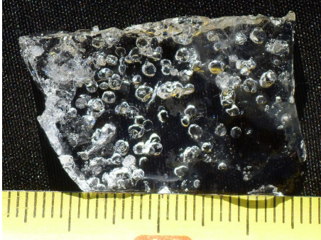
Fig. 10: Picture taken in the field during the CPH campaign showing air bubble inclusions in blue ice
