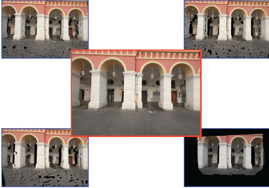
Figure 6.6: The four side images show the warped superpixels of 4 input images pre-selected to render the current novel view. The central image shows the blended result of the 4 warped images.
