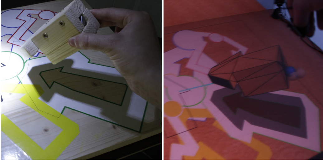
Figure 5.3: Target visibility. Left: in the physical setup, the contours of the targets are completed with dot lines. Right: in the virtual setup, the current target is displayed on top.
