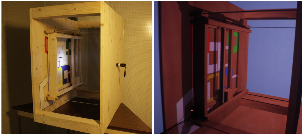
Figure 5.10: 3 degree of freedom translations. Left: physical device. Right: virtual device.
