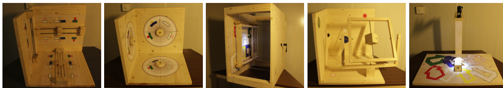
Figure 5.2: Devices used to decompose motion. From left to right: 1D translations, 1D rotations, 3D translations, 3D rotations, free movement.
