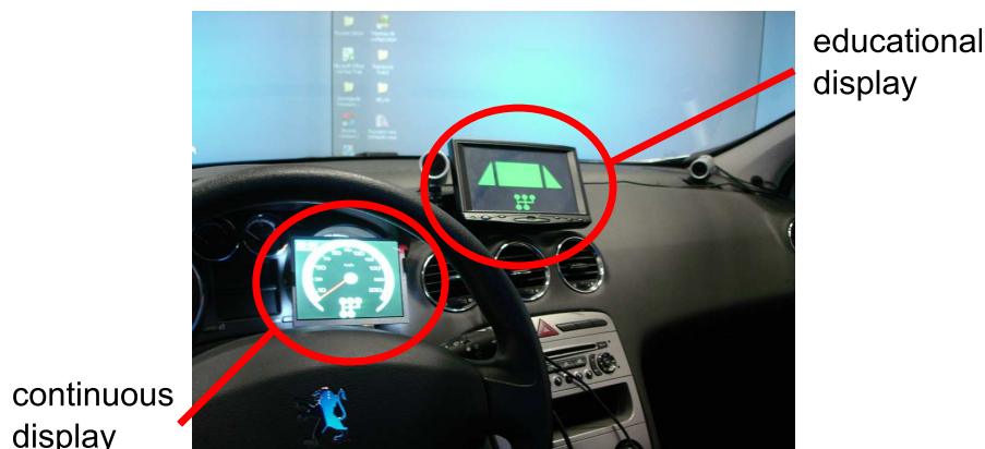
FIGURE 7.7: Installation of HMI
