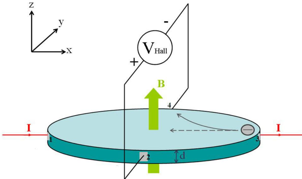
**Figure 4-14 Schematic of a Hall effect measurement**
