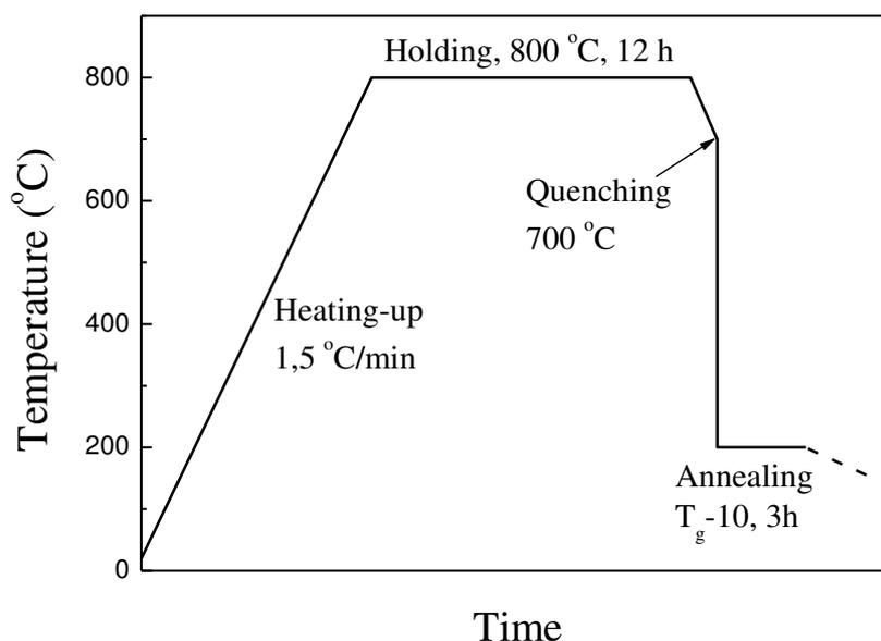
**Figure 2-6 Thermal procedure for chalcogenide glass synthesis**
