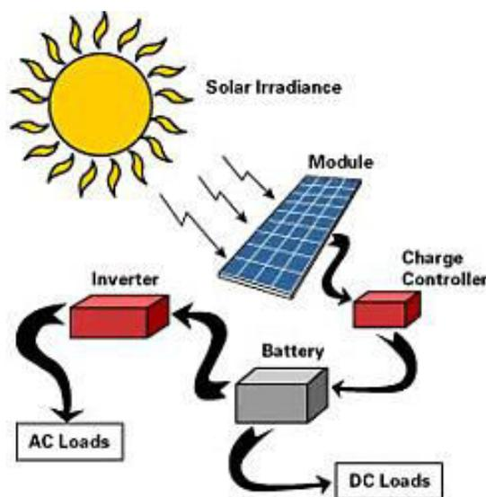
**Figure 1-12 Solar energy photoelectric conversion system [20]**
