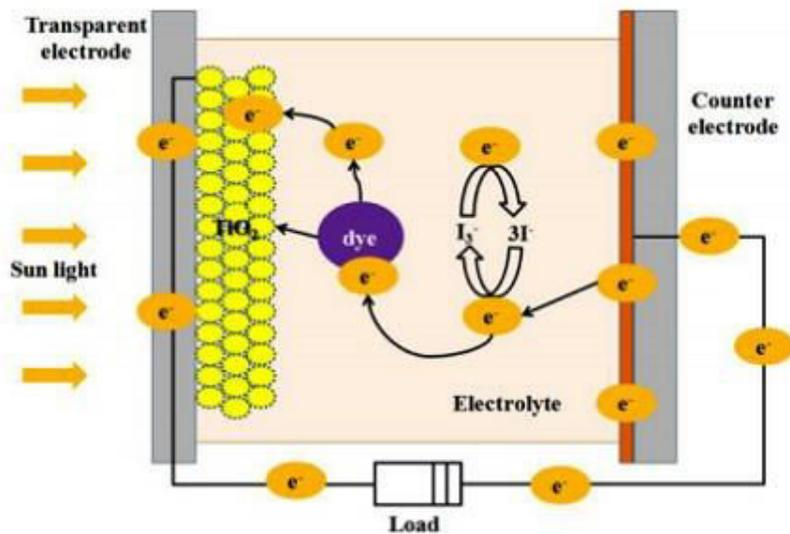
**Figure 1-23 Schematic diagram of dye-sensitized solar cells (DSSC) [55]**
