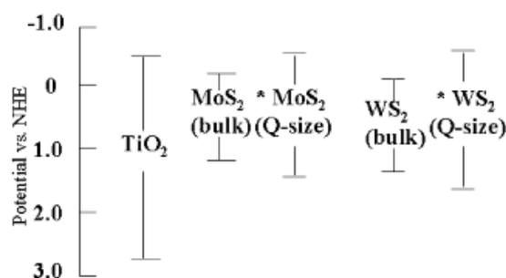
**Figure 1-33 Energy levels of the conduction and valence band edges versus normal hydrogen electrode (NHE) for pure TiO<sub>2</sub>, WS<sub>2</sub> and MoS<sub>2</sub> with various sizes at pH 7 [150]**
