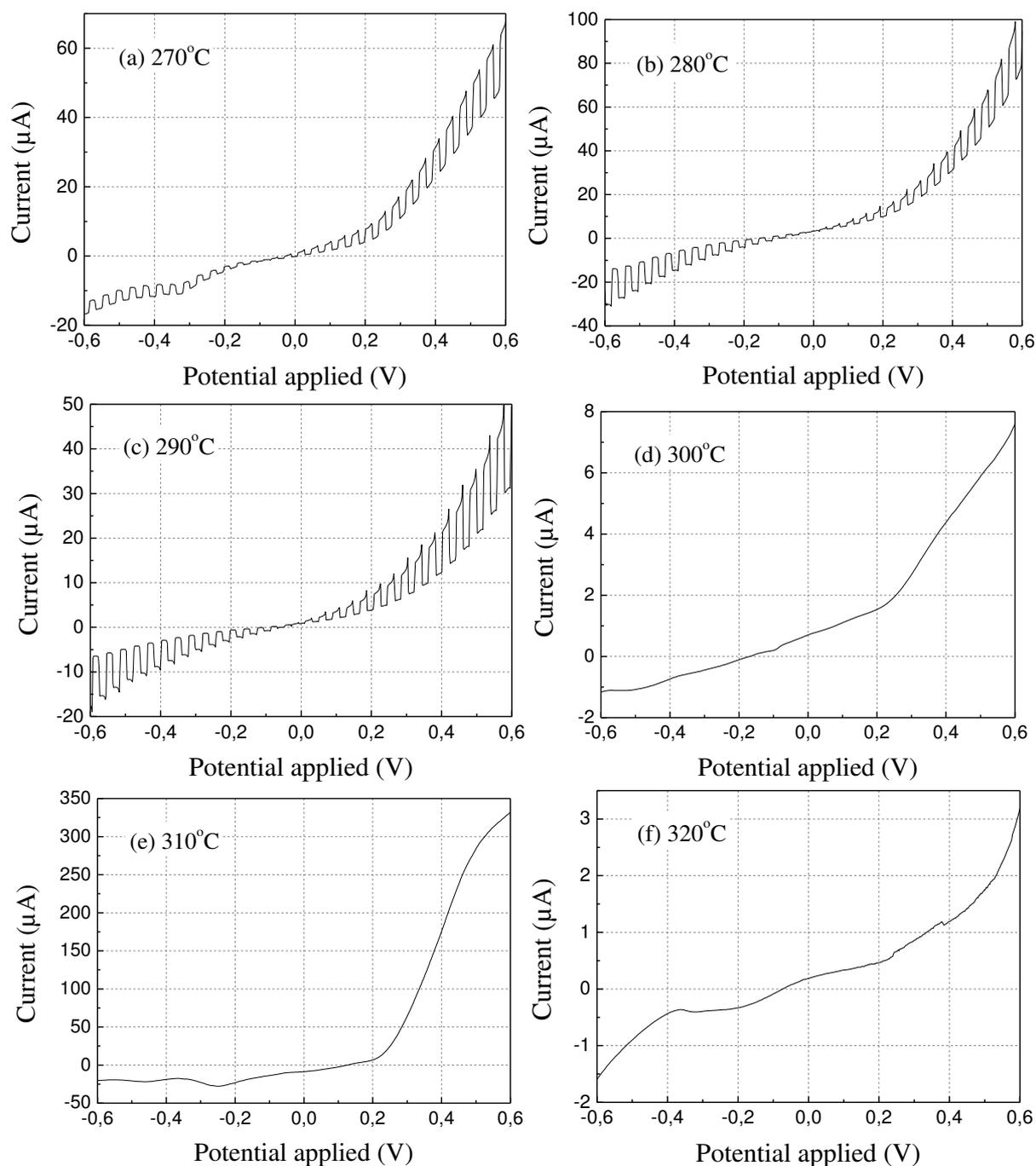
**Figure 3-20 Current-voltage characteristics of the glass ceramics with different crystallization temperature under chopped visible light illumination**
