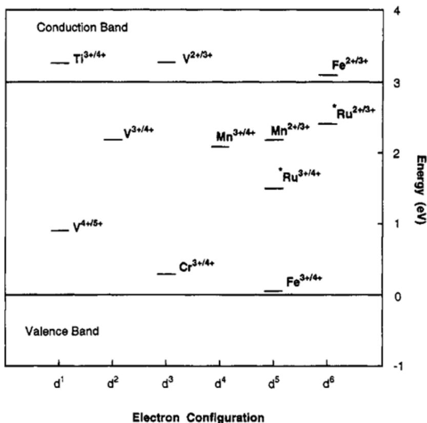
**Figure 1-28 Energy levels of impurity metal ions in TiO<sub>2</sub> [129]**
