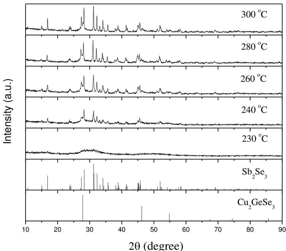
Figure 3-1 XRD patterns of the glass ceramics with different annealing temperature
