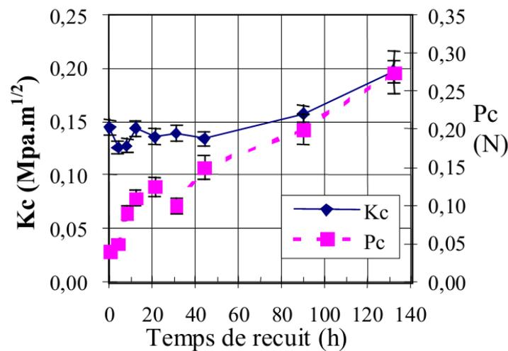
**Figure 2-2 Tenacity ( $K_c$ ) and critical load for crack initiation ( $P_c$ ) of  $62.5\text{GeS}_2\text{-}12.5\text{Sb}_2\text{S}_3\text{-}25\text{CsCl}$  annealed at  $290^\circ\text{C}$  for different times**
