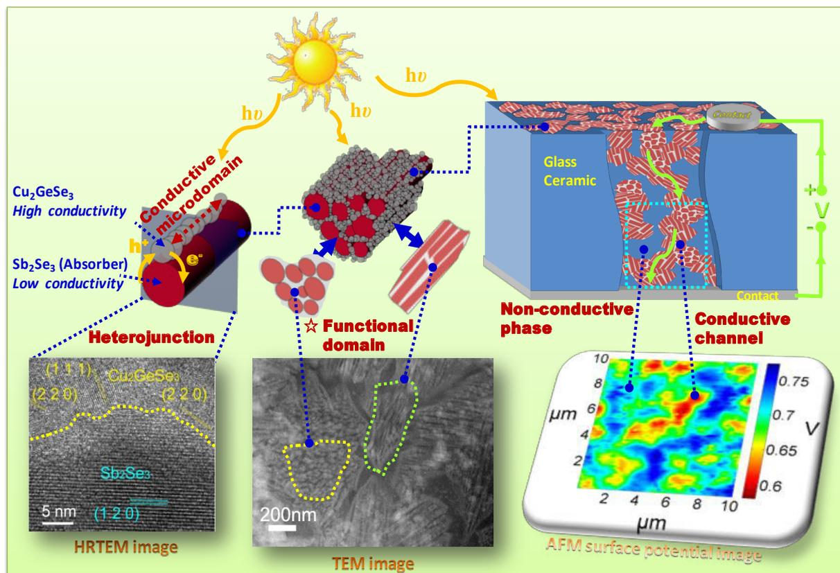
**Figure 4-18** Mechanisms of charge photo-generation, dissociation and transport in the photoelectric glass ceramic
