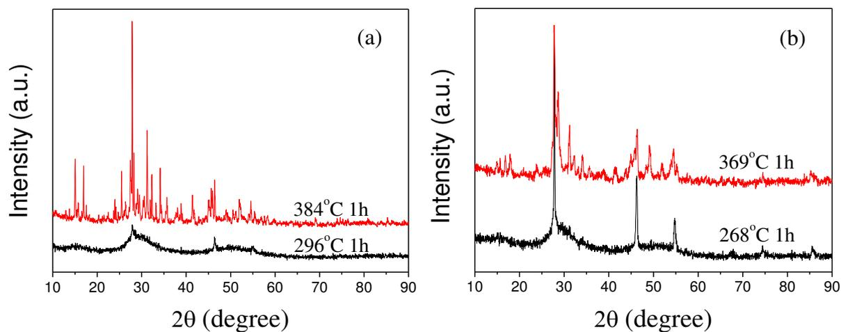
**Figure 2-18** XRD patterns of samples annealed at different crystallization temperature for 1 h: (a)  $72\text{GeSe}_2\text{-}18\text{Sb}_2\text{Se}_3\text{-}10\text{CuI}$ ; (b)  $64\text{GeSe}_2\text{-}16\text{Sb}_2\text{Se}_3\text{-}20\text{CuI}$
