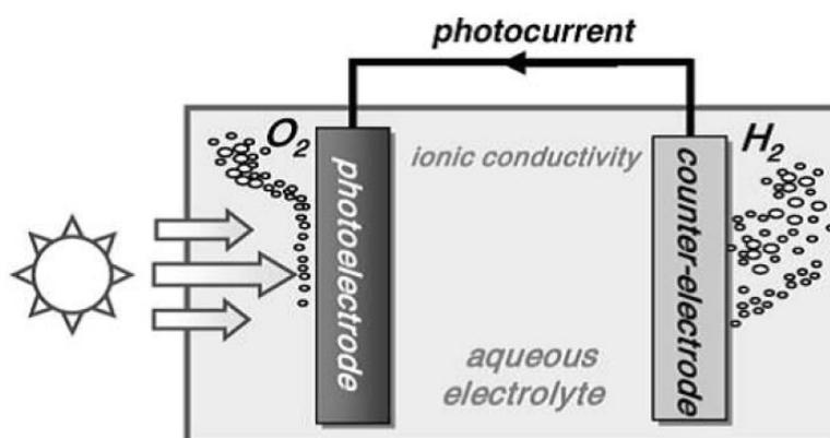
**Figure 1-11 typical setup for PEC water splitting**
