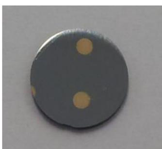
**Figure 4-9 Photograph of a sample with two contacts for I-V measurements**
