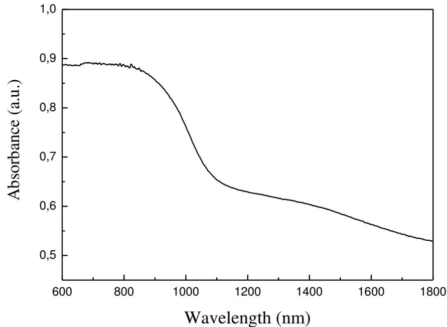
**Figure 4-7 Absorption spectrum of the glass ceramic**
