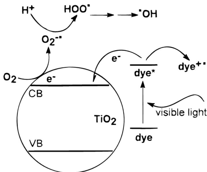
**Figure 1-30 Schematic diagram of dye sensitization mechanism of TiO<sub>2</sub> [144]**
