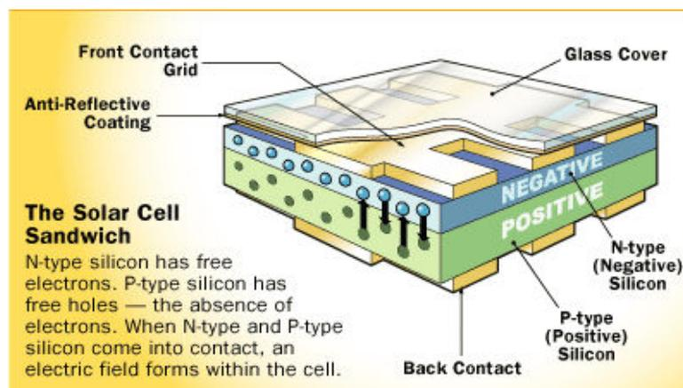
**Figure 1-16 principal of crystalline silicon solar cells (©2006 HowStuffWorks) [33]**
