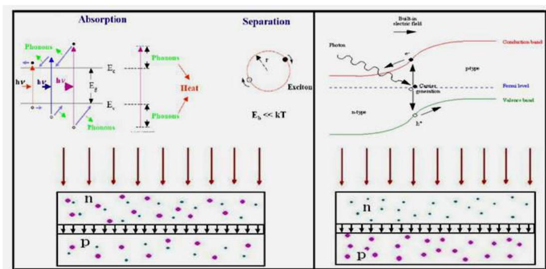
Figure 1-13 Working principle of semiconductor based solar cell
