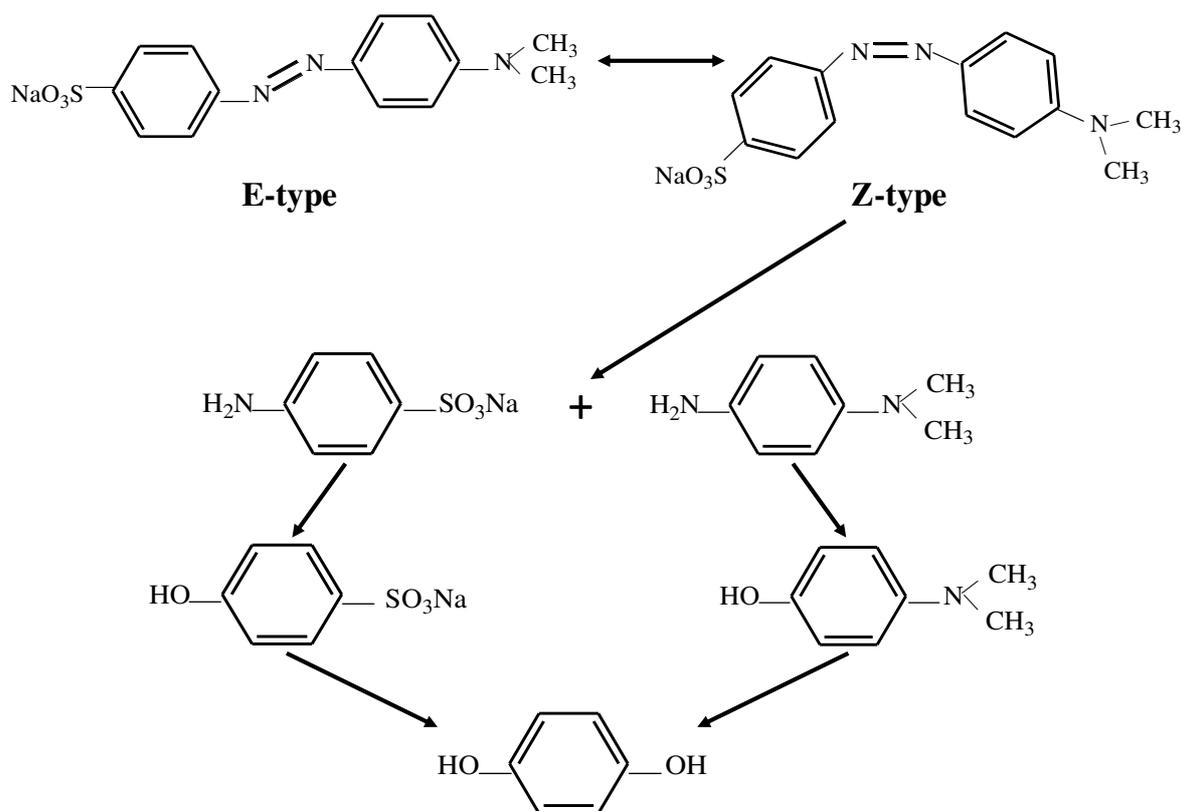
**Figure 5-11 Main pathways proposed for MO photodegraded by the glass ceramic under visible light.**
