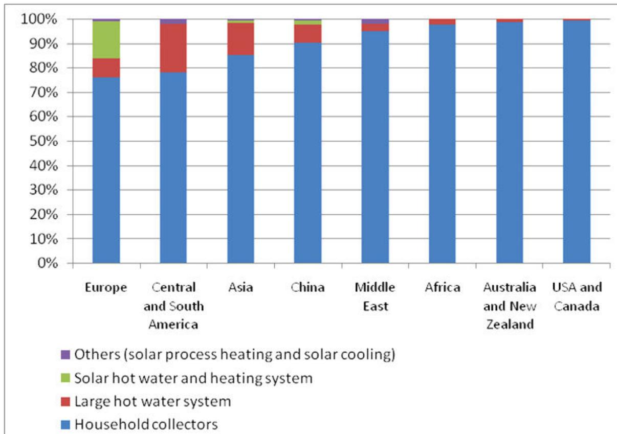
**Figure 1-4 Solar thermal utilization forms in the world [4]**
