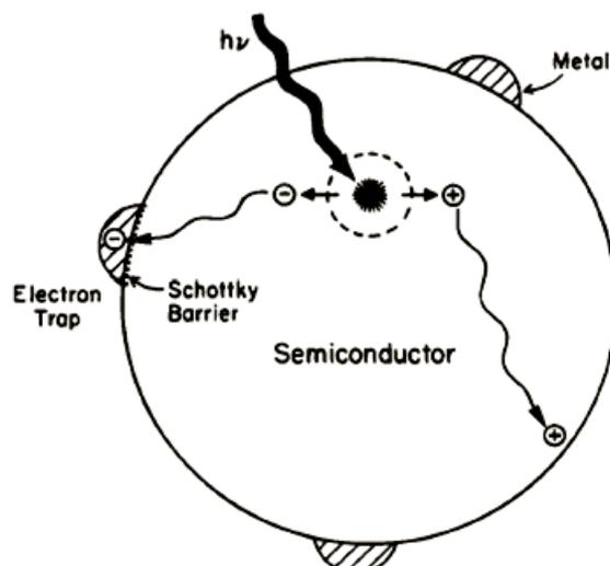
**Figure 1-29 Schematic diagram of photoexcitation in metal-modified semiconductor**
