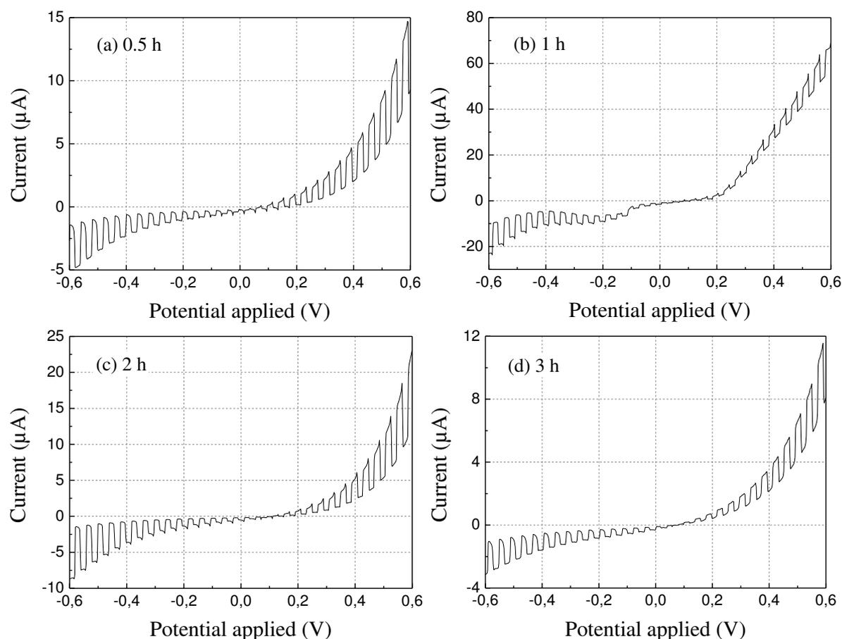
**Figure 3-22** Current-voltage characteristics of the glass ceramics with different crystallization time under chopped visible light illumination
