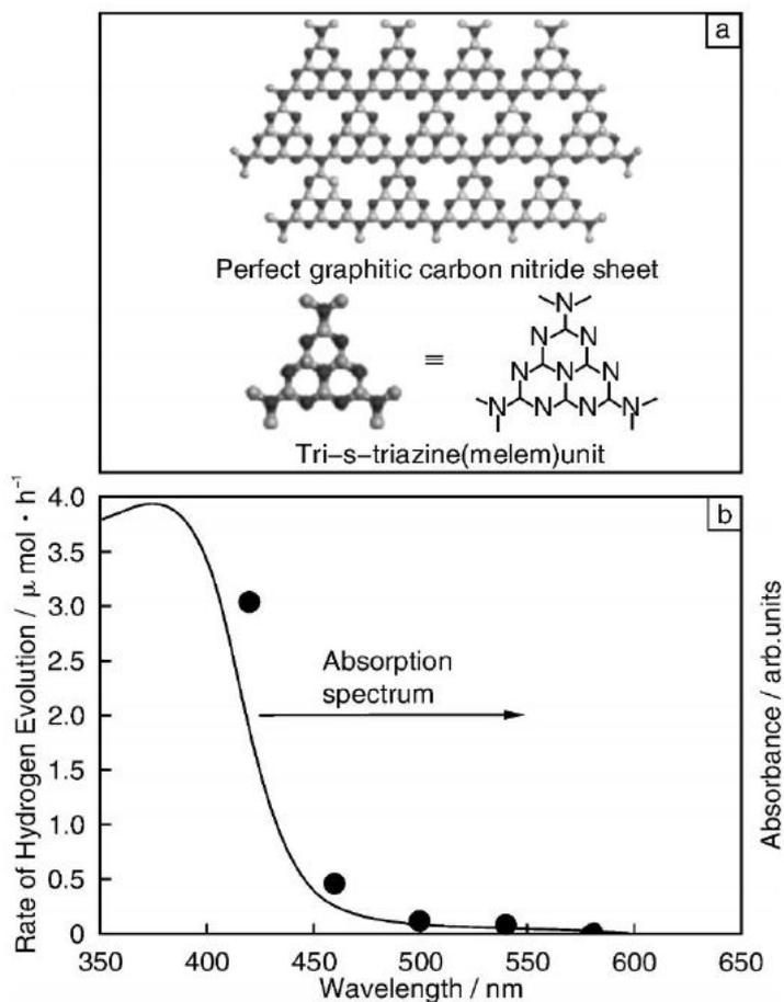
**Figure 1-34 (a) Crystal structure of g-C<sub>3</sub>N<sub>4</sub> and (b) relationship of the photocatalytic hydrogen production activity and the wavelength**
