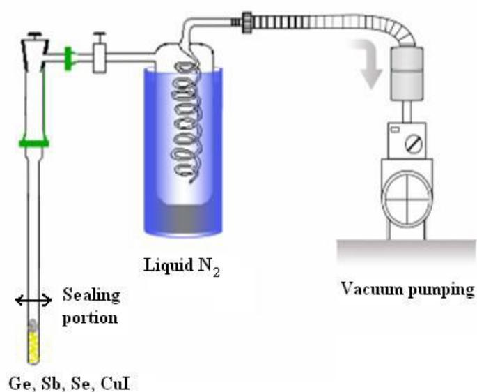
**Figure 2-4 Setup used for preparation of chalcogenide glasses**
