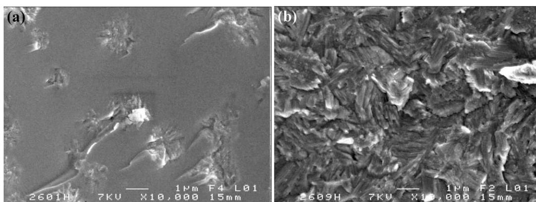
**Figure 3-6 SEM images of the glass ceramics with different annealing times: (a) 1h; (b) 9h**
