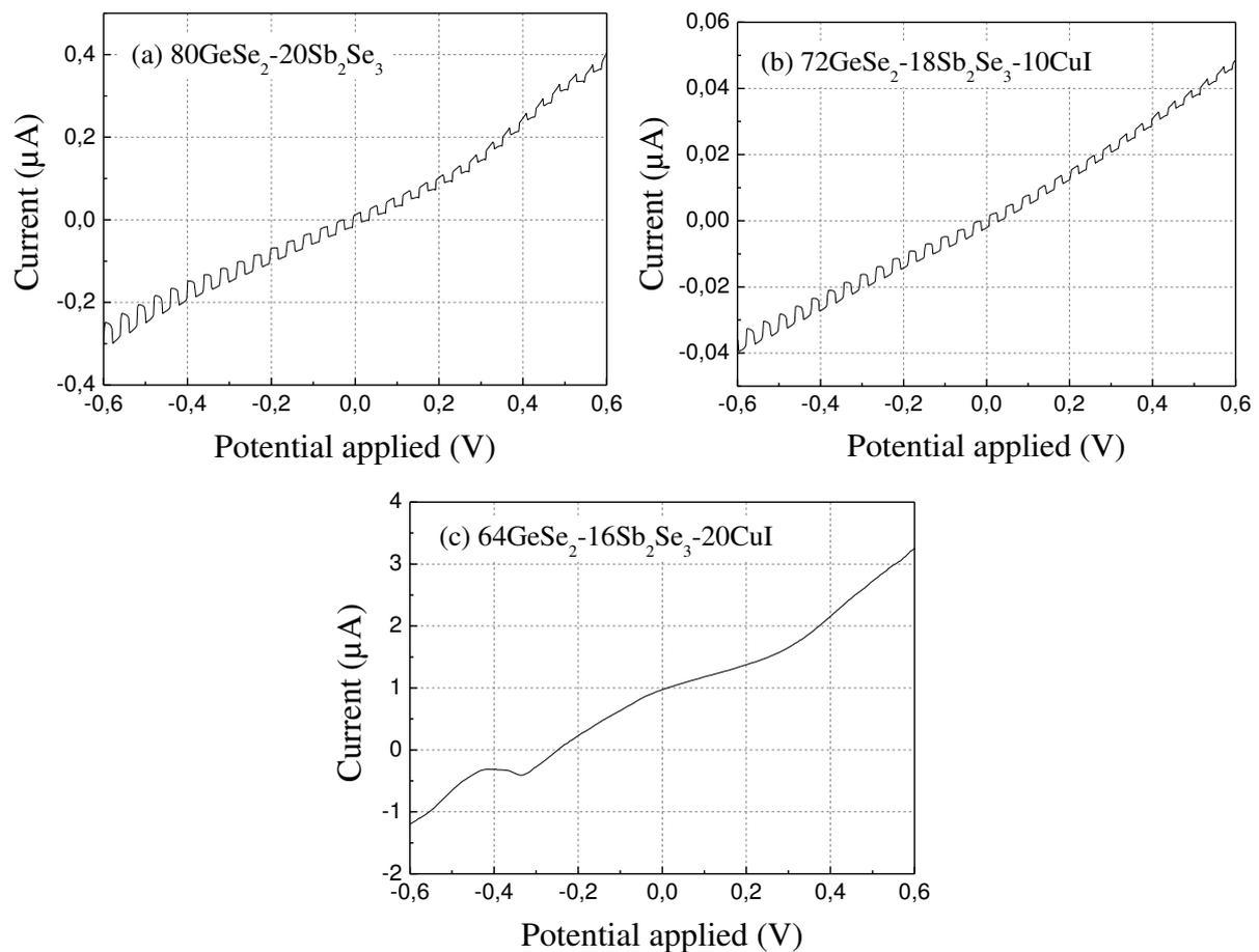
**Figure 2-20 Current-voltage characteristics of different glass ceramics in Series 1 under chopped visible light illumination**
