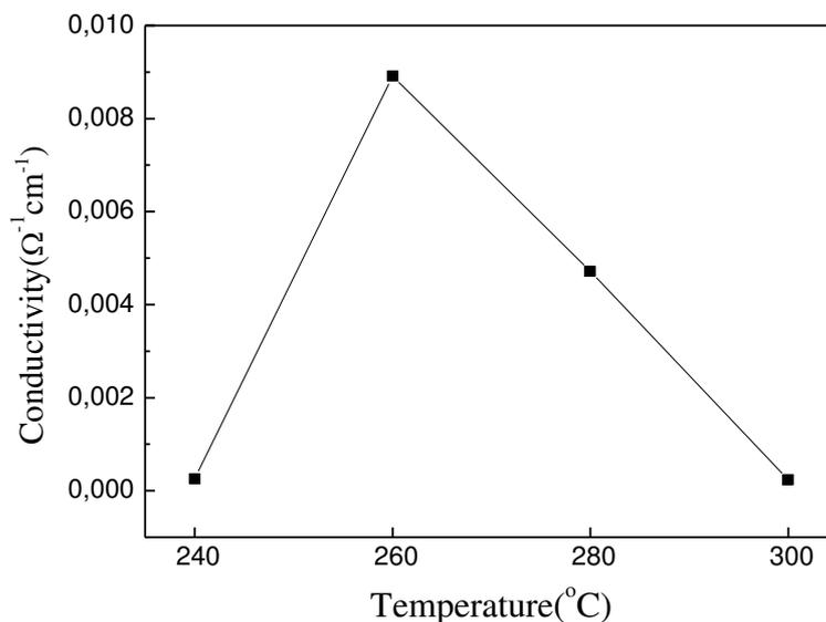
**Figure 3-3 Conductivities of the glass ceramics with different annealing temperatures**
