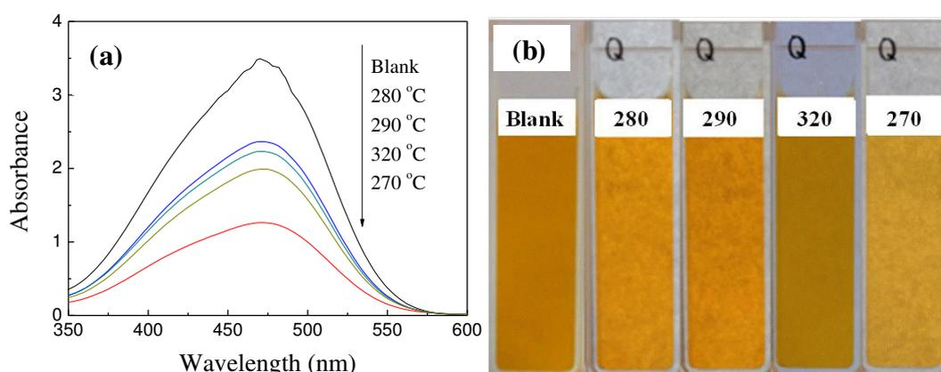
**Figure 5-6 (a) UV-vis absorption spectra and (b) corresponding color of MO solutions before and after photocatalytic reaction over different  $40\text{GeSe}_2\text{-}40\text{Sb}_2\text{Se}_3\text{-}20\text{CuI}$  glass ceramics prepared by a two-stage heat treatment with different temperatures**
