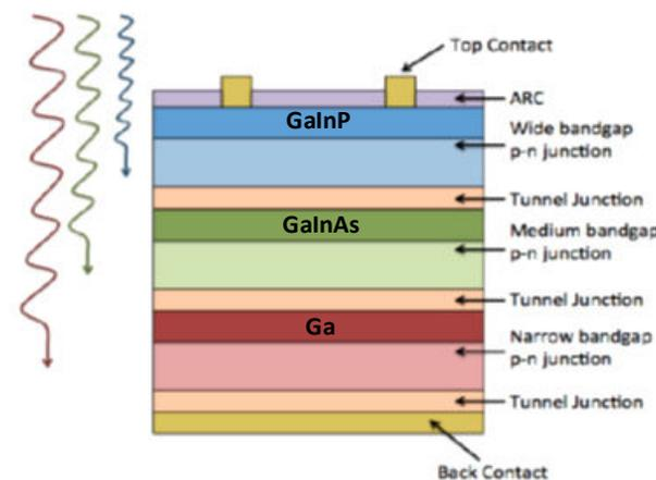
**Figure 1-24 Schematic of multi-junction GaAs solar cells**
