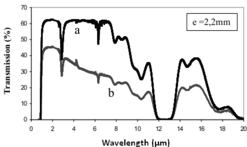
Figure 2-3 Transmission curve of (a) glass  $60\text{GeSe}_2\text{-}30\text{Sb}_2\text{Se}_3\text{-}10\text{CuI}$  and (b) glass ceramic obtained after annealing at  $260\text{ }^\circ\text{C}$  for 1 h
