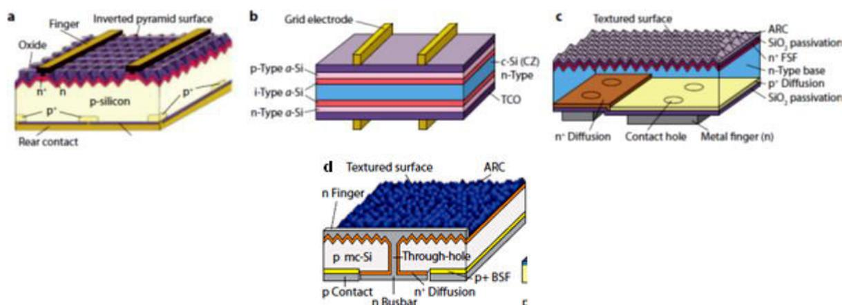
**Figure 1-19 Schematics of various crystalline solar cell structures**
