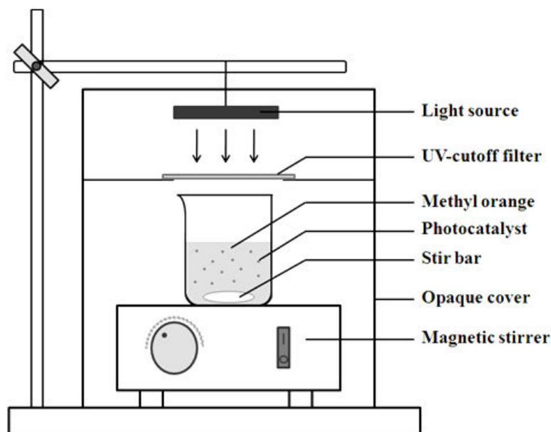
**Figure 5-2 Schematic presentation of the photocatalytic reactor**
