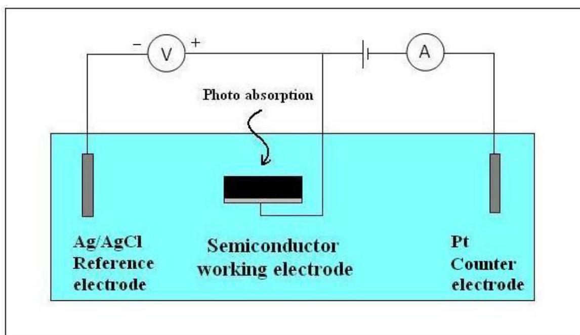
**Figure 2-13 Schematic presentation of three-electrode PEC method**
