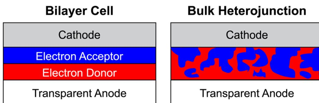
**Figure 1-22** Two kinds of structure of polymer solar cells
