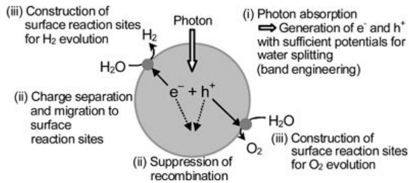
**Figure 1-9 Main processes of photocatalytic water splitting [16]**
