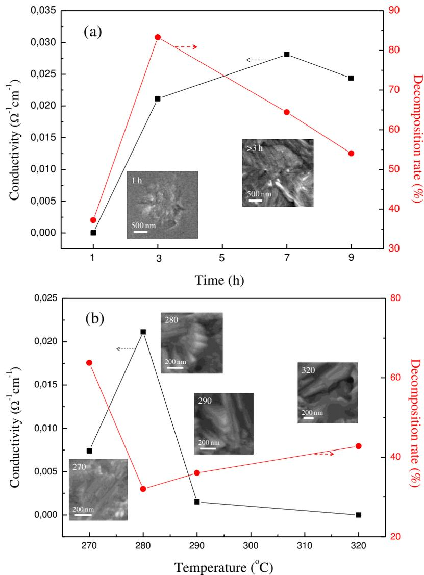
**Figure 5-7 SEM images, conductivities and photocatalytic decomposition rates of MO for different glass ceramics prepared (a) by a single-stage heat treatment at 260 °C for different times; (b) by a two-stage heat treatment with different temperatures.**
