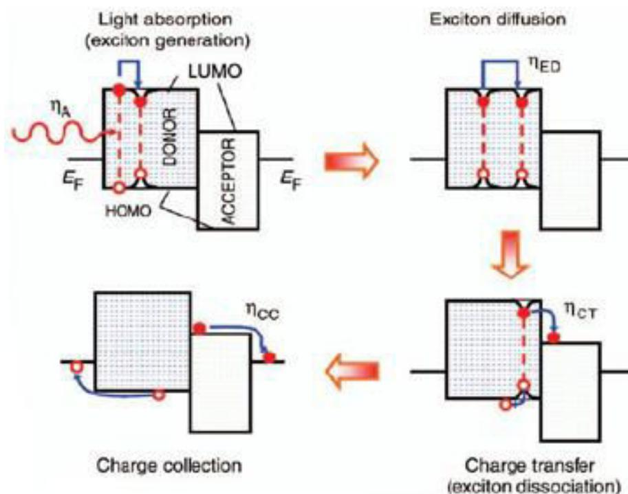
**Figure 1-21 Mechanism for polymer solar cells [45]**
