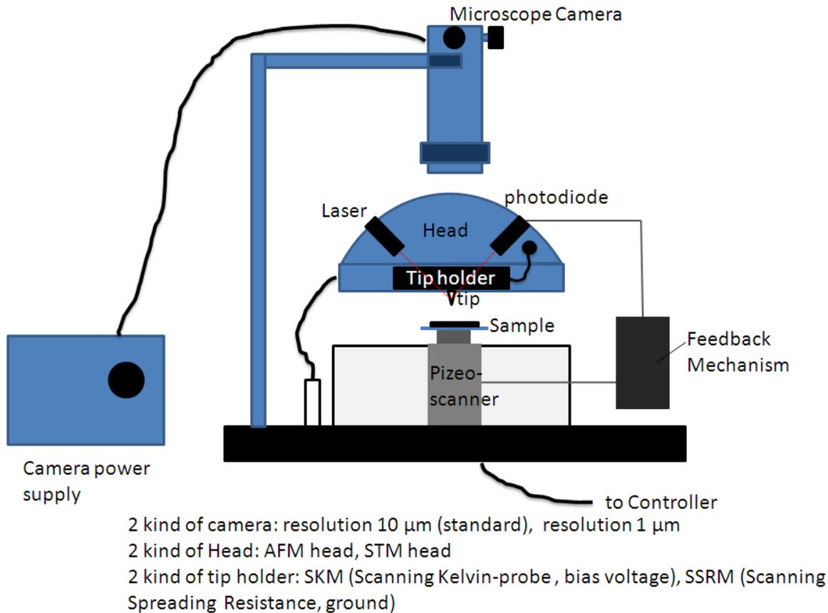
**Figure 4-4 Schematic presentation of atomic force microscope (AFM)**
