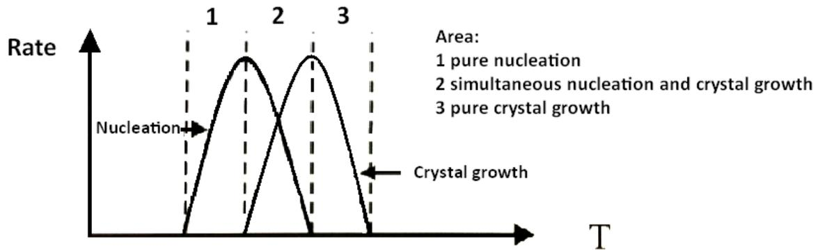
**Figure 2-9 Schematic diagram of the crystallization process**
