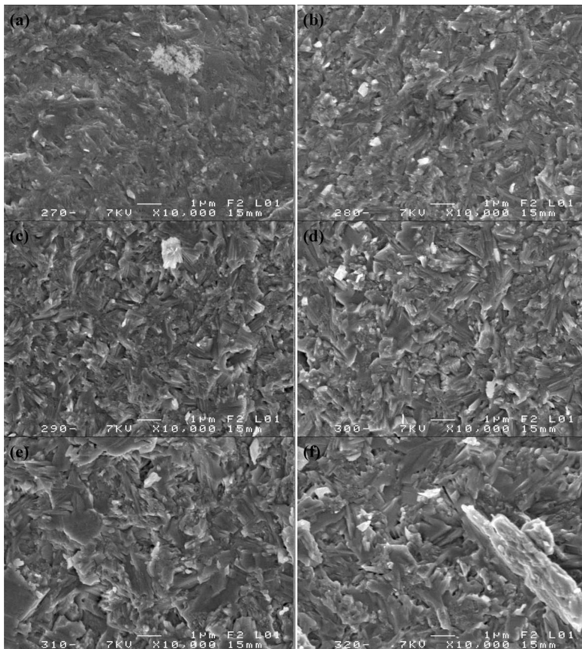
**Figure 3-17 SEM images of the cross section of the glass ceramics prepared by crystallizing the pre-nucleated (220 °C for 90 min) glasses at different temperatures for 1 h: (a) 270 °C; (b) 280 °C; (c) 290 °C; (d) 300 °C; (e) 310 °C; (f) 320 °C**
