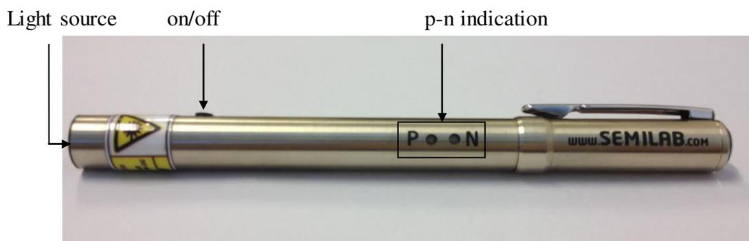
**Figure 2-15 Photograph of a Semilab PN tester**
