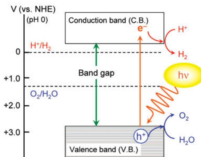
**Figure 1-10 Principle of water splitting using semiconductor photocatalysts**
