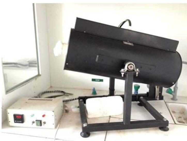
**Figure 2-5 Photograph of a rocking furnace**
