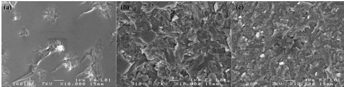
**Figure 4-3 SEM images of typical morphology of the glass ceramics with different conductivities (a)  $3.2 \times 10^{-8} \Omega^{-1} \cdot \text{cm}^{-1}$ ; (b)  $< 10^{-8} \Omega^{-1} \cdot \text{cm}^{-1}$ ; (c)  $2.1 \times 10^{-2} \Omega^{-1} \cdot \text{cm}^{-1}$**
