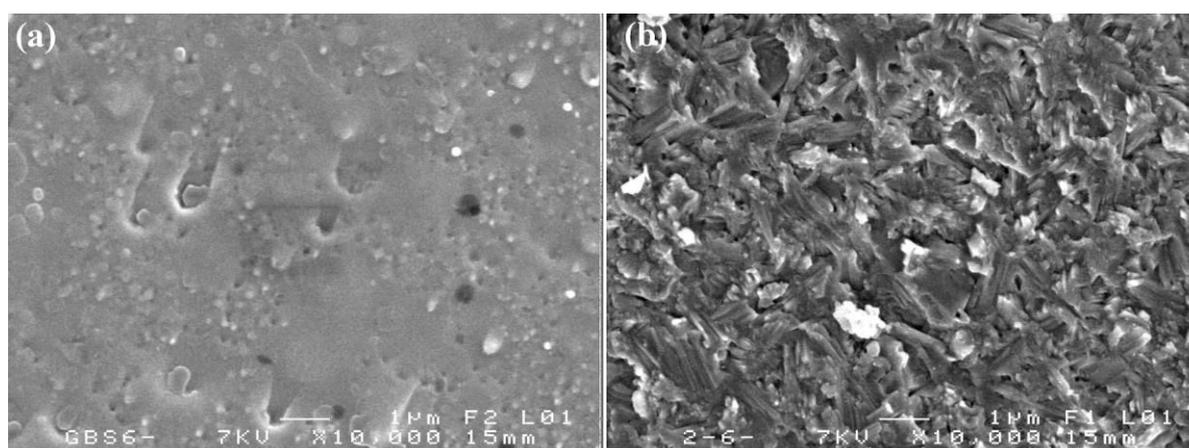
**Figure 2-30 SEM images of the different glass ceramics: (a)  $56\text{GeSe}_2\text{-}24\text{Sb}_2\text{Se}_3\text{-}20\text{CuI}$ ; (b)  $40\text{GeSe}_2\text{-}40\text{Sb}_2\text{Se}_3\text{-}20\text{CuI}$**
