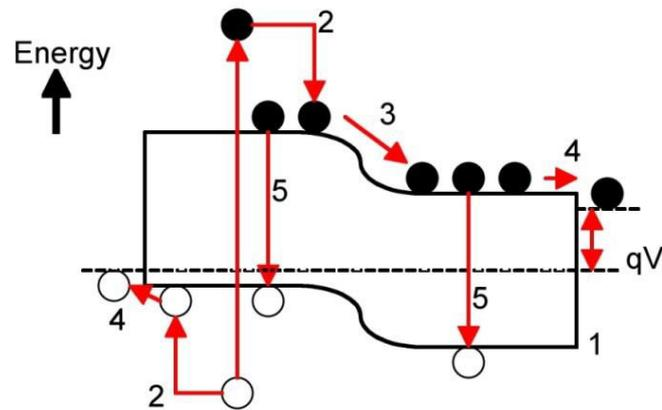
**Figure 1-17 Illustration of energy loss in a p-n junction silicon solar cell: (1) unabsorbed light, (2) excess energy loss as heat, (3) Fermi level mismatch with band gap, (4) transfer loss, and (5) electron-hole recombination**
