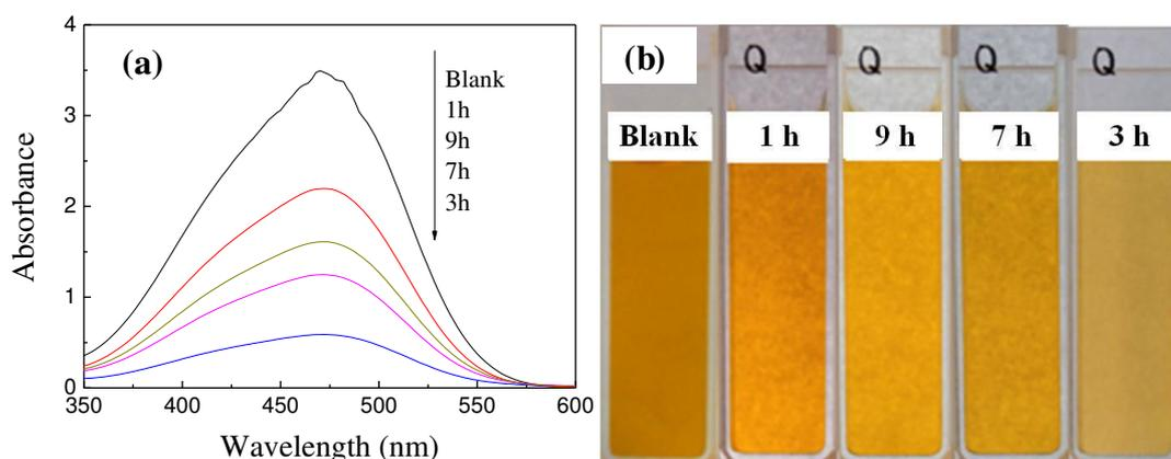
**Figure 5-5 (a) UV-vis absorption spectra and (b) corresponding color of MO solutions before and after photocatalytic reaction over different  $40\text{GeSe}_2\text{-}40\text{Sb}_2\text{Se}_3\text{-}20\text{CuI}$  glass ceramics prepared by a single-stage heat treatment at  $260\text{ }^\circ\text{C}$  for different times**
