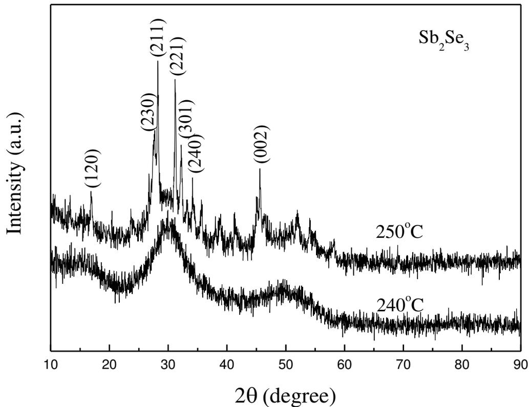
**Figure 3-11 XRD patterns of the 40GeSe<sub>2</sub>-40Sb<sub>2</sub>Se<sub>3</sub>-20CuI samples nucleated at 240 °C and 250 °C for 1h**
