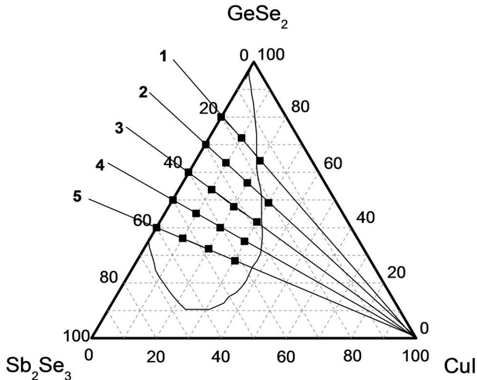
Figure 2-8 Glass-forming region in the ternary diagram of  $\text{GeSe}_2\text{-Sb}_2\text{Se}_3\text{-CuI}$
