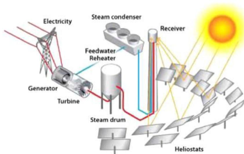
**Figure 1-6 Central receiver power tower system [9]**
