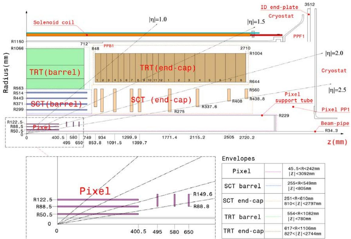
Figure 2.5 – Side view of the Inner Detector with its main elements, active dimensions and envelope.
