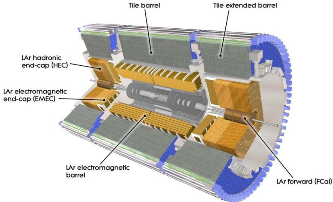
Figure 2.6 – Cut-away view of the ATLAS calorimeter system.
