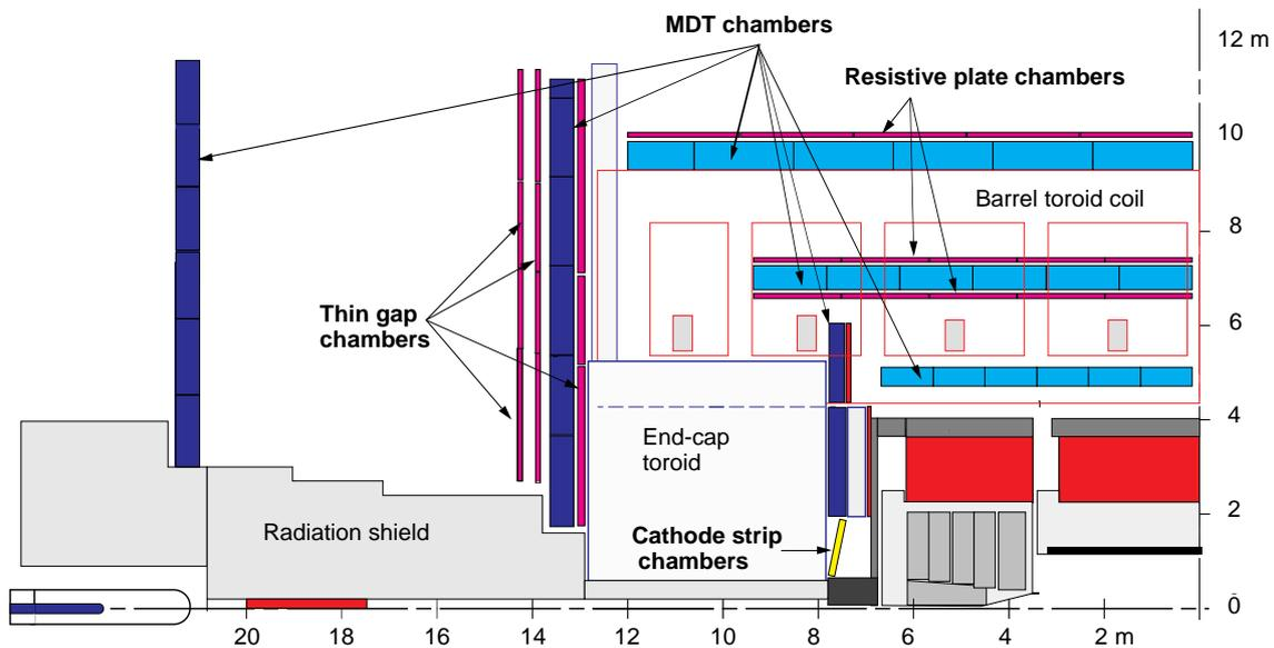
Figure 2.8 – Cross-section of the muon system in  $R$ - $z$  plane.
