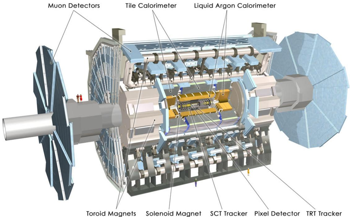
Figure 2.4 – Cut-away view of the ATLAS detector.
