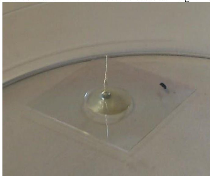
Fig.5-20. Needle of 1.2 cm height fabricated with 130 kHz amplified microchip laser with maximum average power of 200 mW to compensate for spherical aberration.
