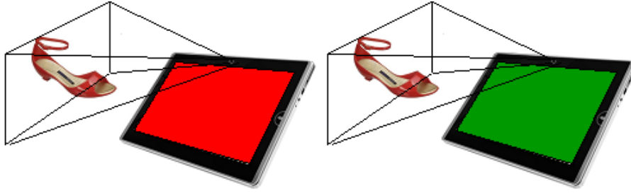
Figure 5.1: Multispectral data can be obtained with hand-held devices by using the screen to illuminate the object under various illuminations. The acquired measurements can be used to reconstruct the spectral reflectance.
