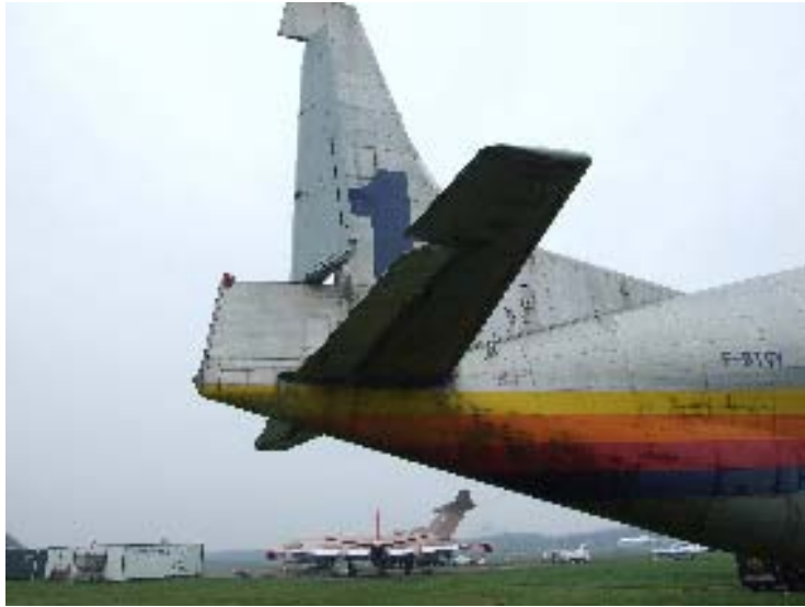
Figure 1.10 Hardover rudder on Airbus Skylink (by Mick Ward)
