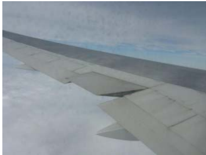
Figure 1.9 Stuck aileron on B-767 in flight
