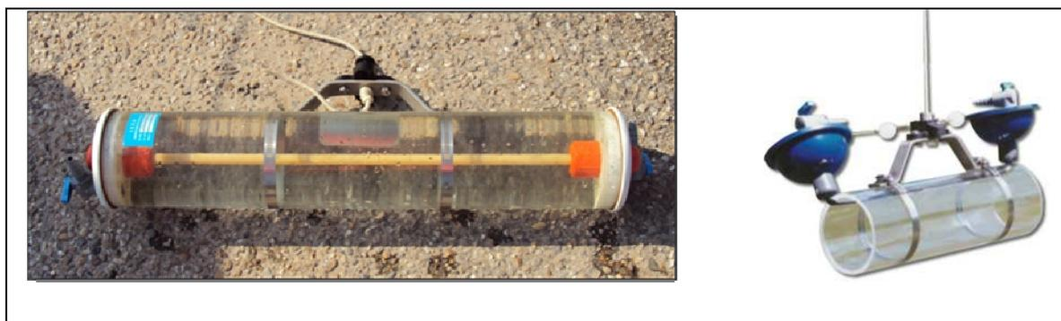
Figure III.10. Van Dorn water sampler (source of the picture on the right: Ecoenvironmental)
