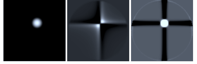
Fig. 4. Simulations of the influence function f_i in the pupil plane (left), and the effect using the two different estimators: we deconvolve by the mask ( \Phi_{\text{est}} , right) or not ( \Phi_{\text{est},2} , center).
