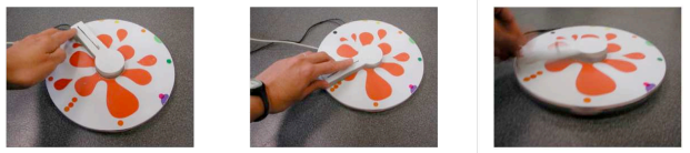
Figures 13, 14 and 15: Illustrations of actions for selecting and playing a list, selecting a play within a play-list, selecting music plays according to the BPM mode
