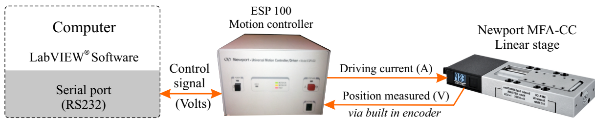
FIGURE C.2: Schematic layout of the linear stage control
