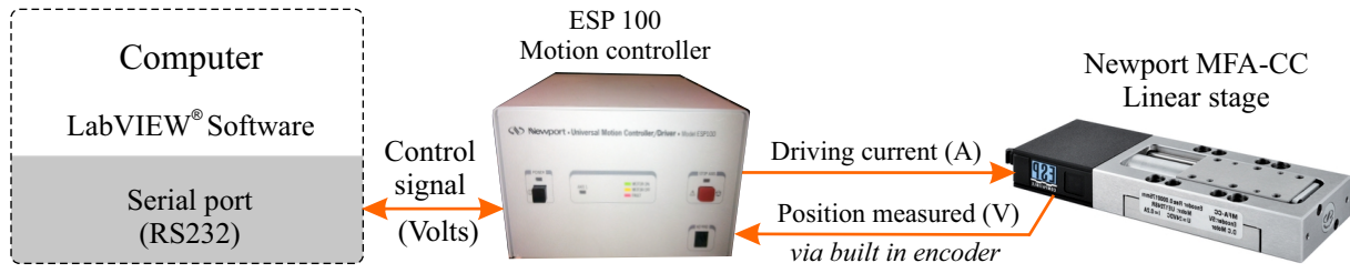
FIGURE C.2: Schematic layout of the linear stage control
