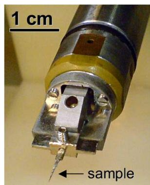
Figure 1.22: Home-made needle shape sample holder tip.
