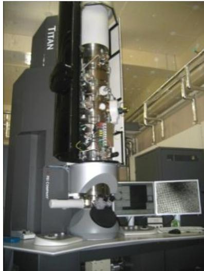
Figure 2.23: View of TEM of FEI TITAN with C<sub>s</sub>-corrector.
