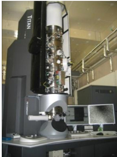
Figure 2.23: View of TEM of FEI TITAN with C_s -corrector.
