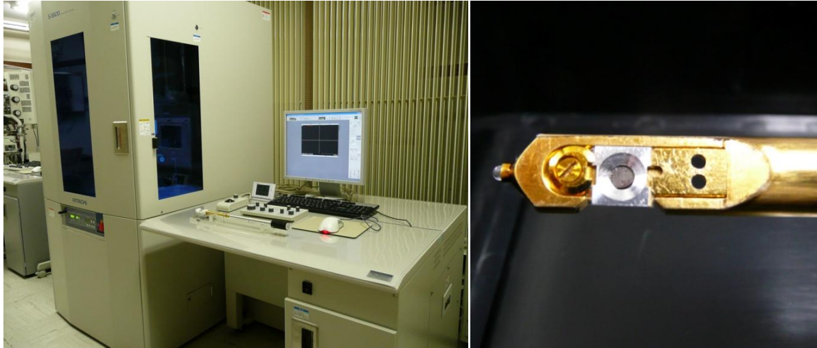
Figure 2.50: General view of the S5500 Hitachi microscope at Tohoku University (Sendai, Japan); on the right side, the tip of TEM specimen holder (compatible with the STEM mode in the SEM) is shown.
