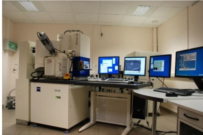
Figure 1.8: FIB/SEM NVision 40 of Carl Zeiss installed at CLYM.
