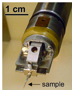
Figure 1.22: Home-made needle shape sample holder tip.
