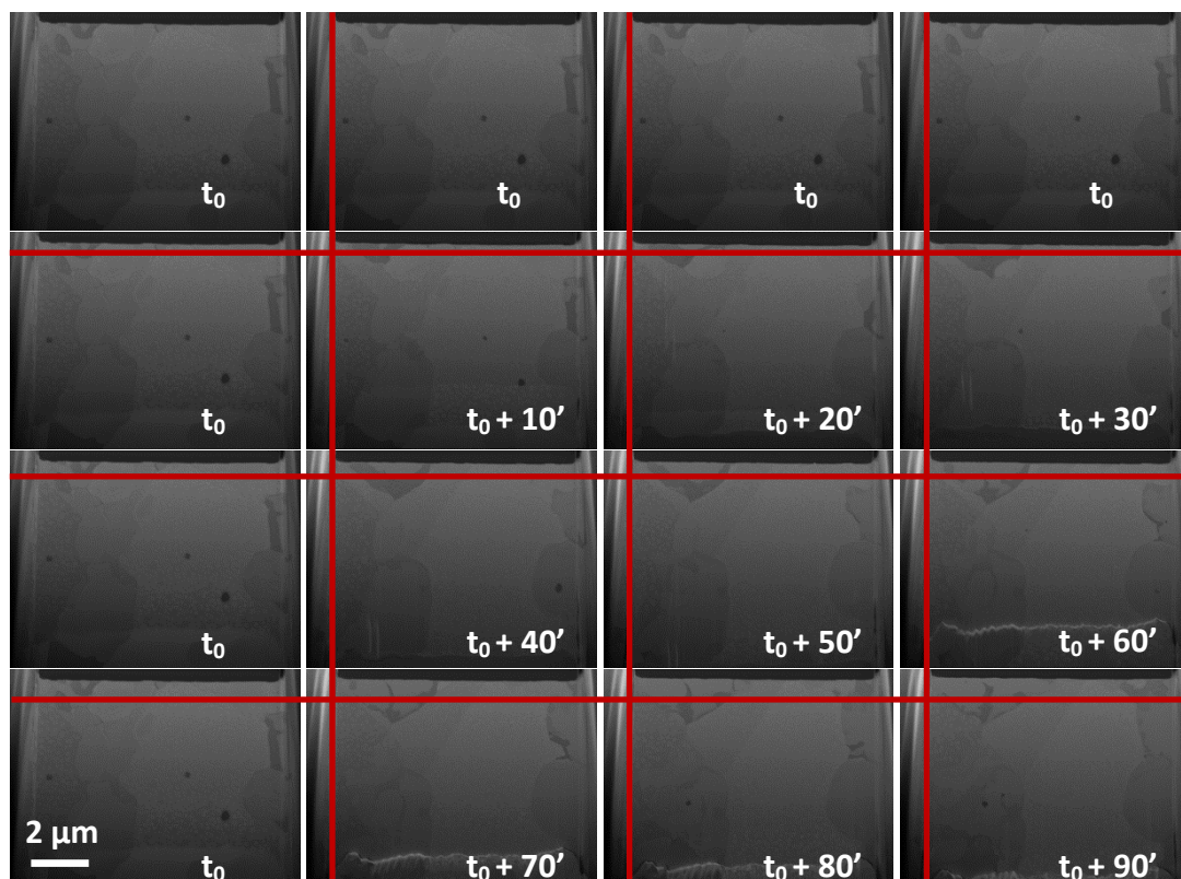
Figure 3.21: Reduced image series from a FIB/SEM tomography on a Ni alloy with the in-situ drift correction program running. The initial (reference at time t_0 ) image is repeated in the first row and column, the other ones being recorded at different times (as indicated). Red lines are guides for the eye indicating the left position of the carbon deposited layer as a reference marker, and proving the absence of any significant drift. [Yuan2012]
