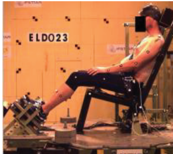
Fig. 27. Sled configuration based upon a standard sedan car environment of a front passenger restrained by a 3-point belt.
