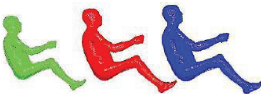
a) 5th female, 50th and 95th percentile male obtained from HUMOS mesh.
