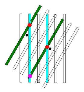
Fig. 6.3: Hit position reconstruction ambiguities with silicon strip detectors. The figure displays a false double layer equipped with silicon strips placed with a stereo angle. Coloured are the strips that give a hit signal. The two black dots represent the real hits, while their reconstructed positions are shown in red. A ghost hit, marked with magenta colour, will be reconstructed.
