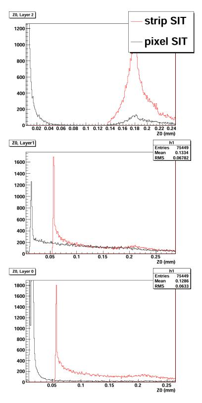
Fig. 6.6: Uncertainty  $\delta z_0$  on the track extrapolation for the strip SIT (red) and the pixel SIT (black). Top: extrapolation from layer 3 to layer 2. Center: extrapolation from layer 2 to layer 1. Bottom: extrapolation from layer 1 to layer 0.
