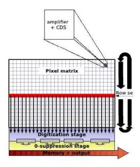
Fig. 3.4: The principle of column parallel readout [Baudot 10].
