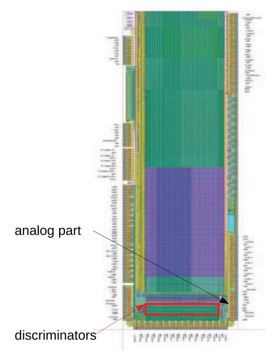
Fig. 4.4: Layout of the MIMOSA 22 sensor. The rolling shutter is performed from the top to the bottom of the pixel array.
