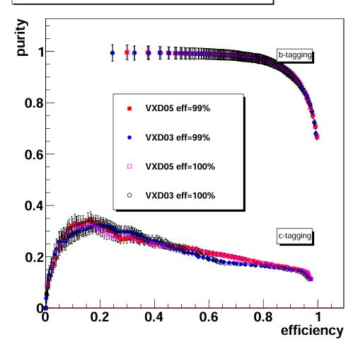
Fig. 5.14: Purity versus efficiency for b- and c-tagged jets for each geometry. The red full squares stand for the VXD05 and detection efficiency of 99%, the pink open squares stand for the VXD05 and detection efficiency of 100%, the blue full circles for the VXD03 and detection efficiency of 99% and the black open circles for the VXD03 and detection efficiency of 100%
