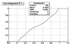
Fig. 4.2: Left part: the  $\eta$  distribution built on a reference plane of the silicon strip beam telescope. Right part: the normalised integral of the  $\eta$  distribution over 700 events for the same plane.
