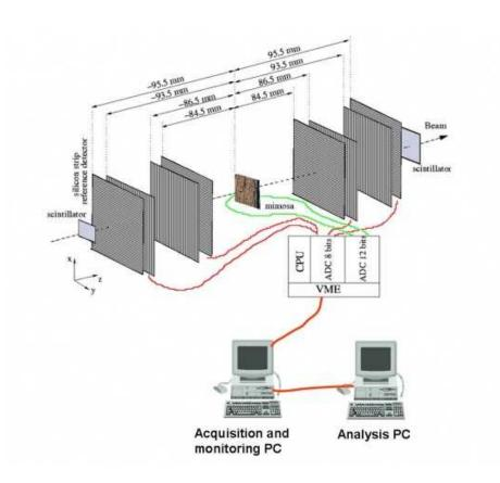
Fig. 4.1: Schematic representation of the silicon strip telescope and its DAQ system.
