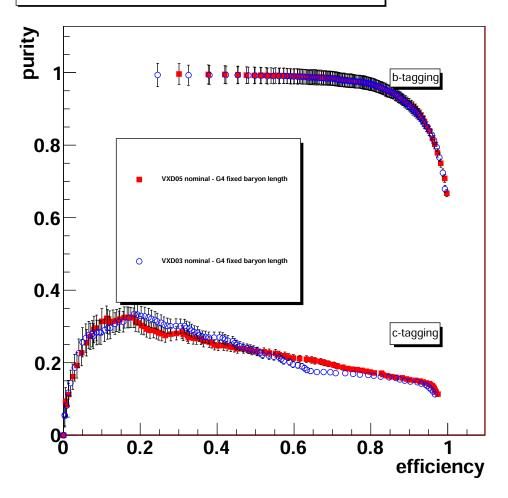
Fig. 5.7: Purity versus efficiency for b- and c-tagged jets for each geometry. The red full squares stand for the VXD05, the blue circles for the VXD03. Only statistical uncertainties are shown.
