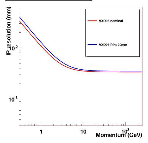
Fig. 5.8: Impact parameter resolution. The blue line is standing for the nominal VXD05 geometry and the red for the VXD05\_rint20.
