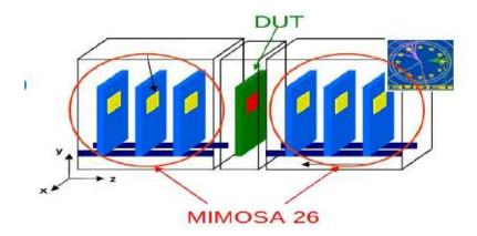
Fig. 3.5: The EUDET beam telescope. It consists of two arms each made of three planes of two MIMOSA 26 sensors. The Detector Under Test (DUT) is placed between the two reference planes (see sub–section 4.1.2 for beam telescopes general description).
