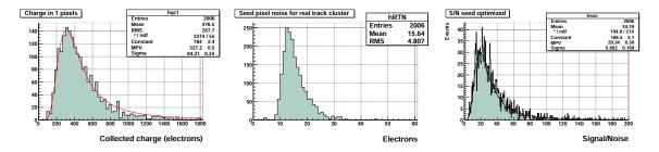
Fig. 4.17: MIMOSA 24 submatrix 1 (diode size equal to  $6 \times 6 \,\mu\text{m}^2$ ) test beam results: left part, charge collected at the seed pixel; middle part, seed pixel ENC; right part, seed pixel SNR.
