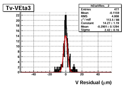
Fig. 4.8: Track-hit residuals of submatrix 5 of a non-irradiated chip. The hit position was recostructed with the  $\eta$  algorithm. The residuals on the U coordinate are illustrated at the top of the figure, while at the bottom are the ones on the V coordinate.
