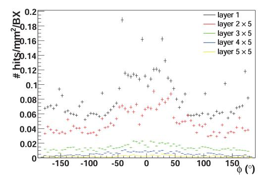
Fig. 2.8: Number of hits per  $mm^2$  per BX for all 5 layers as function of the  $\phi$  (azimuth) angle, assuming the nominal beam parameters. This number has been multiplied by a factor of 5 for layers 2-5. From [De Masi 09]
