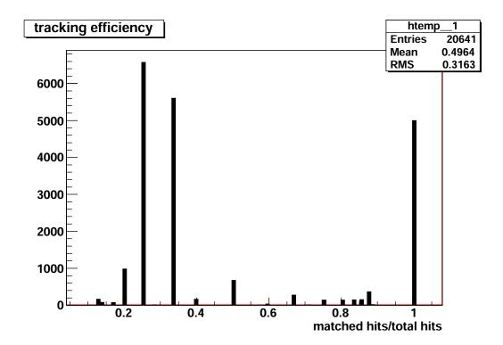
Fig. 5.15: Tracking efficiency of the standalone silicon tracking algorithm, when the beam background hits are included. The horizontal axis represents the ratio of the hits associated to a track that have been generated from the same true particle, versus the total number of hits associated to this track.
