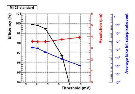
Fig. 3.7: MIMOSA 26 sensor detection efficiency (black line), spatial resolution (red) and fake hit rate (blue) as a function of the discriminator thresholds in units of mV.
