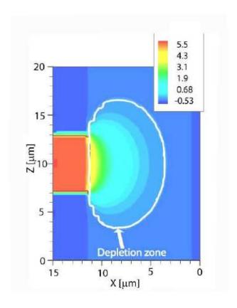
Fig. 3.10: Simulation results from [Dorokhov 10] showing the depleted region created around the diode in a high resistivity  $(1k\Omega \cdot cm)$  epitaxial layer MAPS.
