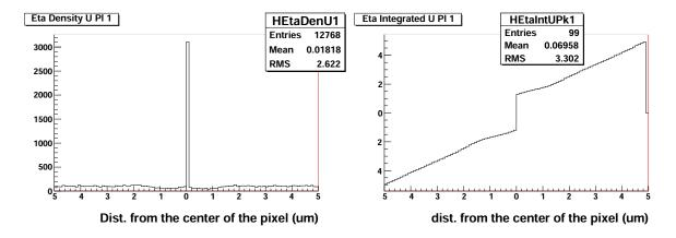
Fig. 4.18:  $\eta$  distributions for the first plane of the TAPI telescope (MIMOSA 18 sensor).Left part:  $\eta$  density, right part:  $\eta$  integrated density. At the horizontal axis is the distance from the center of the pixel.
