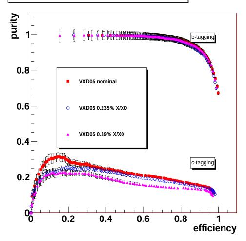
Fig. 5.11: Purity versus efficiency for b- and c-tagged jets as a function of the material budget of the ladder for the VXD05 geometry. The red full squares stand for the nominal material budget of  $0.16\,\%\,X_0$ , the blue circles for  $0.235\,\%\,X_0$  and the pink full triangles for  $0.39\,\%\,X_0$
