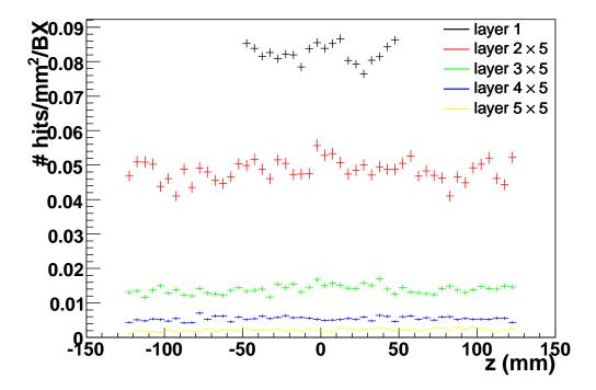
Fig. 2.7: Number of hits per  $mm^2$  per BX for all 5 layers as function of the distance to the IP on the z-axis, assuming the nominal beam parameters. This number has been multiplied by a factor of 5 for layers 2-5. From [De Masi 09]
