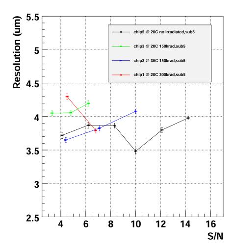
Fig. 4.12: Spatial resolution of submatrix 5 for several integrated radiation doses of the chip and temperatures. Unless otherwise stated, the tests were conducted in a temperature of  $20^{0}$  C. The black line corresponds to 0 radiation, the green to an integrated dose of 150 kRad, the blue to an integrated dose of 150 kRad at a temperature of  $35^{0}$  C and the red to an integrated dose of 300 kRad. the horizontal axis is the discriminators threshold in units of SNR.
