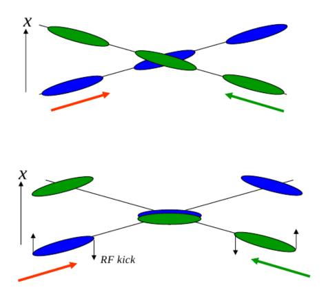
Fig. 2.3: Illustration of the crab crossing technique. The green and blue oval surfaces represent the bunch transverse section of the colliding beams. At the top of the figure one can observe the small overlapping area of the two beams, which leads to a loss of luminosity. Using the crab crossing technique (bottom of the figure), the overlapping area is maximised. From [Zimmerman]
