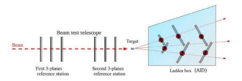
Fig. 3.9: The beam test infrastructure provided within the AIDA framework aiming to investigate the alignment issues on vertex detectors.
