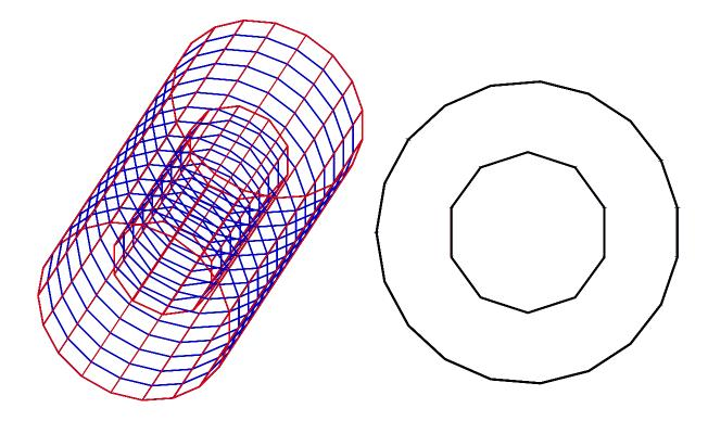
Fig. 6.2: Visualisation of the SIT, as described inside the simulation framework used for the DBD studies. Left: 3D view of the SIT. We can observe the ladder and sensor structure. Right: view of the SIT from the  $R\phi$  plane.
