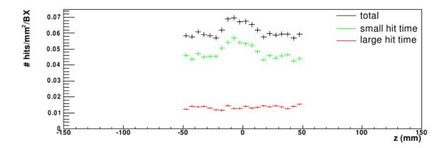
Fig. 2.9: Hit densities due to beamstrahlung in the innermost layer of the VXD as a function of the z coordinate. Top: without the anti-DID field. Bottom: with the anti-DID. The black crosses show the overall hit density, the green (small hit time) the one originating from particles impinging directly the VXD ladders, while the red ones (large hit time) originates from the backscattered particles. From [De Masi 09]
