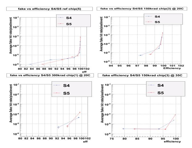
Fig. 4.14: Detection Efficiency–average fake hit rate per pixel trade off for the submatrices S4 (blue line) and S5 (red line) of MIMOSA 22bis. Unless otherwise stated, the tests were conducted in a temperature of  $20^{0}\,C$ . Top: on the left is for the non irradiated chip, on the right for an integrated dose of 150 kRad. Bottom: on the left for an integrated dose of  $300\,\mathrm{kRad}$ .
