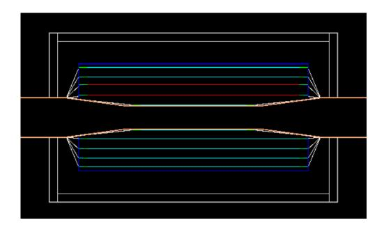
Fig. 2.14: Visualisation of a section of the VXD05 design as described inside the simulation framework (Mokka, see section 5.4) used for the LoI studies. We can see the three double sided ladders (the support is visualised with red, the sensitive with cyan and the supporting electronics with green), the Be support shell (blue), the kapton cables (white) and the cryostat (grey), while the beam pipe is visualised with orange colour.
