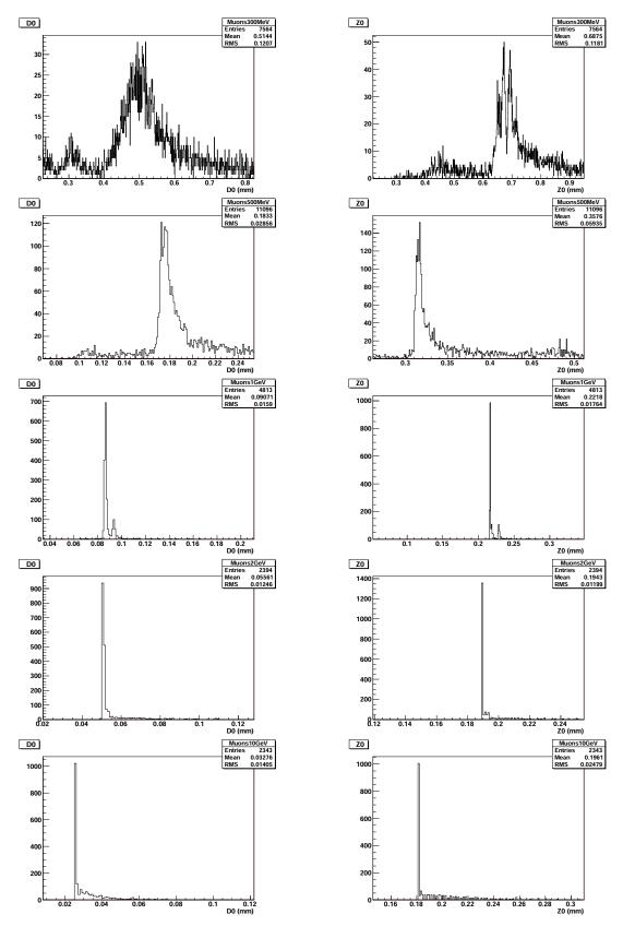
FIG. 6.4: Uncertainties on the extrapolation from the TPC to the outermost SIT layer of the impact parameters  $\delta d_0$  and  $\delta z_0$ , for muon tracks featuring various momenta. Left:  $\delta d_0$ . Right  $\delta z_0$ . Going from top to bottom the muons momenta are 300 MeV, 500 MeV, 1 GeV, 2 GeV and 10 GeV.
