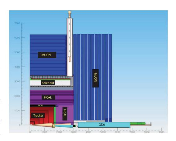
Fig. 2.15: Transverse view of one quadrant of the SiD ([SiD 09]).
