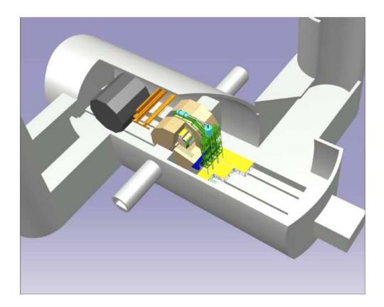
Fig. 2.4: Possible design of the foreseen detector hall for the ILC.
