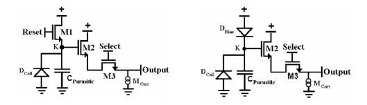
Fig. 3.3: 3T (left) and SB pixel (right) architectures.
