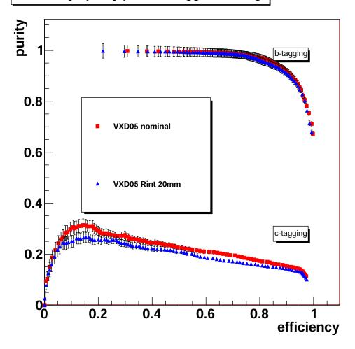
Fig. 5.10: Purity versus efficiency for b- and c-tagged jets in case of VXD05, for two values of the innermost layer radius. The red full squares stand for for 16 mm and the blue full triangles for 20 mm (so-called VXD05\_rint20 variant).
