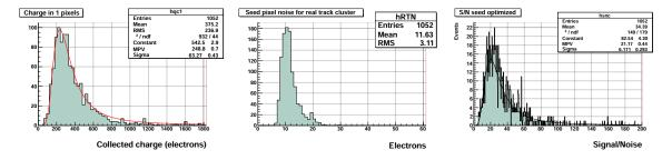
Fig. 4.16: MIMOSA 24 submatrix 0 (diode size equal to  $4.3 \times 3.4 \,\mu\text{m}^2$ ) test beam results: left part, charge collected in the seed pixel; middle part, seed pixel ENC; right part, seed pixel SNR.
