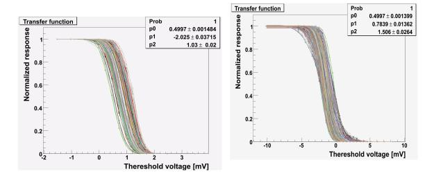
Fig. 4.6: Transfer functions of the MIMOSA 22bis discriminators when applying a threshold scan: Left, standalone; right, connected with the pixel submatrices. The tests were conducted at a temperature of  $20^0 C$ .
