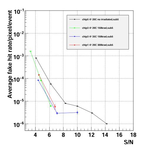
Fig. 4.13: Average fake hit rate per pixel of submatrix 5 for several integrated radiation doses of the chip and temperatures. Unless otherwise stated, the tests were conducted in a temperature of  $20^{0}$  C. The black line corresponds to 0 radiation, the green to an integrated dose of 150 kRad, the blue to an integrated dose of 150 kRad at a temperature of  $35^{0}$  C and the red to an integrated dose of 300 kRad. the horizontal axis is the discriminators threshold in units of SNR.
