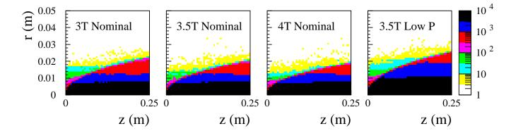
Fig. 2.6: Beamstrahlung  $e^+e^-$  pair particles track density as a function of the radius (vertical axis) and the distance in z (horizontal axis) for several magnetic fields and beam options. The magnetic field value and set of beam parameter are written on each plot. The colour scale at the right part of the figure, decodes the track density. From [LoI 10]
