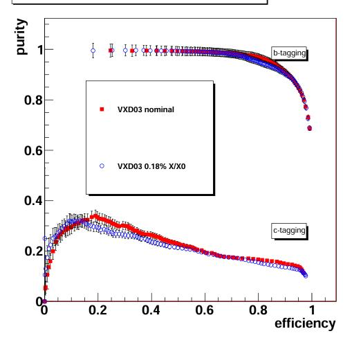
Fig. 5.12: Purity versus efficiency for b- and c-tagged jets as a function of the material budget of the ladder for the VXD03 geometry. The red full squares stand for the nominal radiation length of 0.11% while the blue circles stand for 0.18%.
