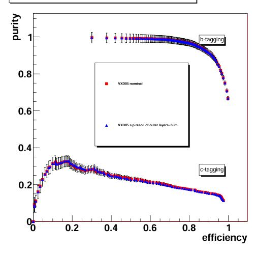
Fig. 5.13: Purity versus efficiency for b- and c-tagged jets using the VXD05 model. The red full squares stand for an assumed sensor's single point resolution for the 2 outer double layers of 2.8  $\mu m$ , while the blue full triangles stand for a 5  $\mu m$  resolution instead.
