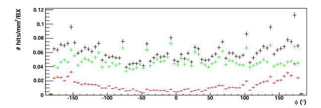
Fig. 2.10: Hit densities due to beamstrahlung in the innermost layer of the VXD as a function of the azimuthal  $\phi$  angle. Top: without the anti–DID field. Bottom: with the anti–DID. The black crosses show the overall hit density, the green (small hit time) the one originating from particles impinging directly the VXD ladders, while the red ones (large hit time) originates from the backscattered particles. From [De Masi 09]
