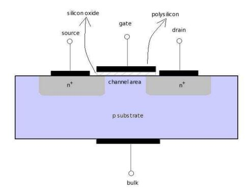
Fig. 3.1: Section of an NMOS FET.
