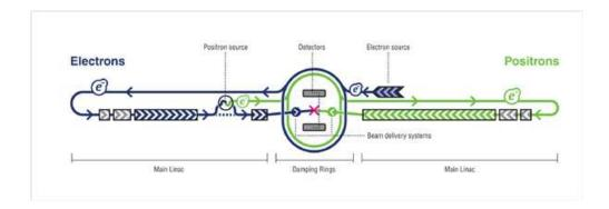
Fig. 2.2: Schematic layout of the ILC for the 500GeV option.
