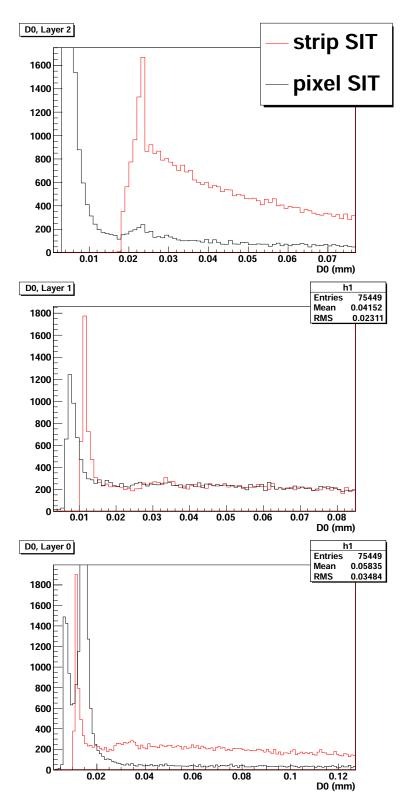
Fig. 6.5: Uncertainty  $\delta d_0$  on the track extrapolation for the strip SIT (red) and the pixel SIT (black). Top: extrapolation from layer 3 to layer 2. Center: extrapolation from layer 2 to layer 1. Bottom: extrapolation from layer 1 to layer 0.
