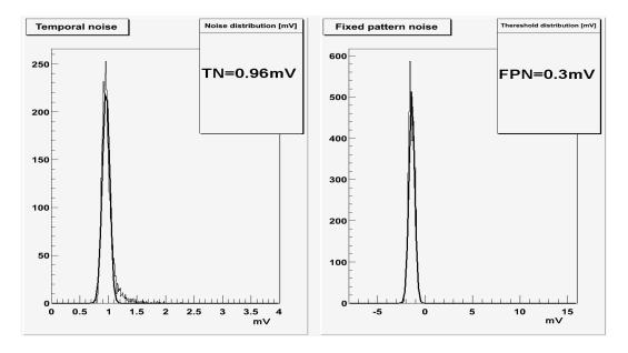
Fig. 4.7: Noise performance of the submatrix S5 of MIMOSA 22bis combined with the discriminators, after being irradiated with an integrated dose of 300 kRad, at a temperature of  $20^{0}$  C. Left, temporal noise; it corresponds to  $\sim 17\,e^{-}$  ENC. Right, fixed pattern noise dispersion; it corresponds to  $\sim 5\,e^{-}$  ENC.
