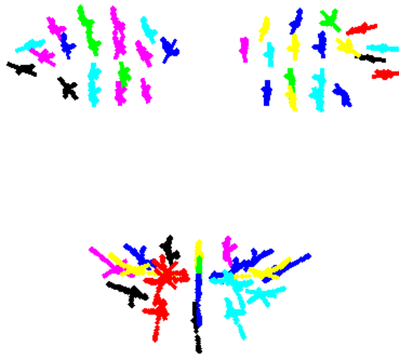
Figure 3.3: Identification of the principle axes of the displacement of the facial landmarks of one subject. These landmarks are traced while the subject blinks his eyes, lowers his eyebrows, frowns and says A/I/O phonemes.
