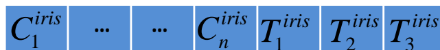
Figure 3.16: A chromosome of the genetic algorithm; The parameters inside are those of the iris appearance and pose
