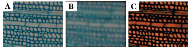
Figure 3. Difference of Gaussian filtering on a cross-section of Mahogany stained with toluidine blue. A: the image obtained by applying a small Gaussian blurring ( \sigma = 3 pixels). B: the image resulting from a strong Gaussian blurring ( \sigma = (\text{image width})/10 ). C: subtraction of images A and B which increases the contrast wall / lumen.
