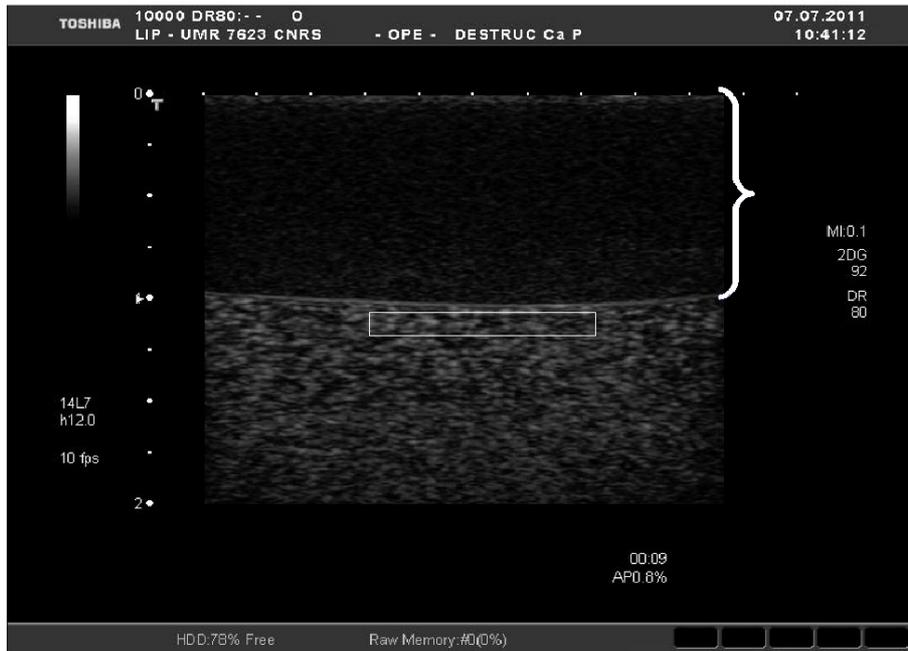
Figure 3.1: Image acquired during the dose ranging experiment ( $2 \times 10^5$  microbubbles/mL). The bracket designates the gelatin stand-off placed between the transducer and the surface of the microbubble suspension. The white rectangle delimits the region of interest in the contrast agent suspension from which average echo-power was calculated. Image pixel values were converted into echo-power using custom software developed by our group [50].
