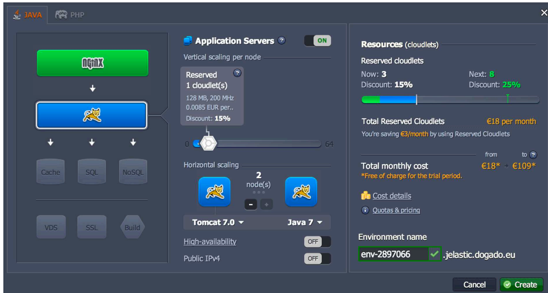
Figure 4.2: Configuring two application server instances in Jelastix
