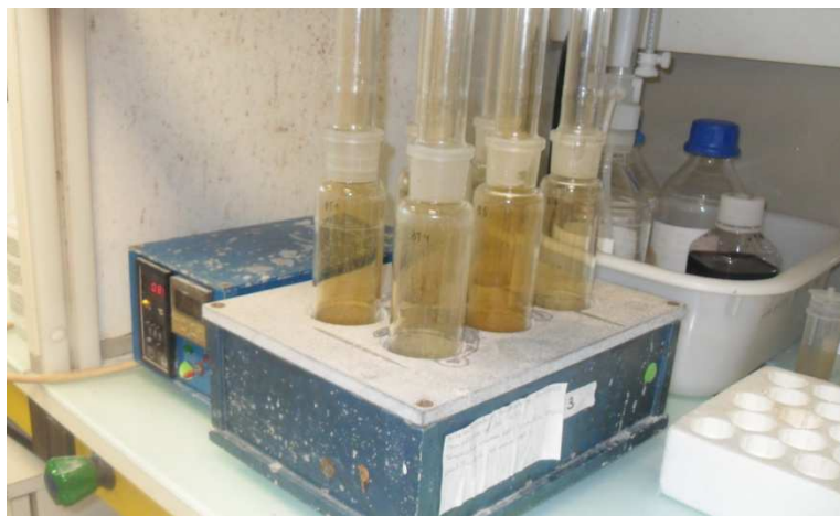
Picture 3.3 Digestion of mollusk samples by hot plate
