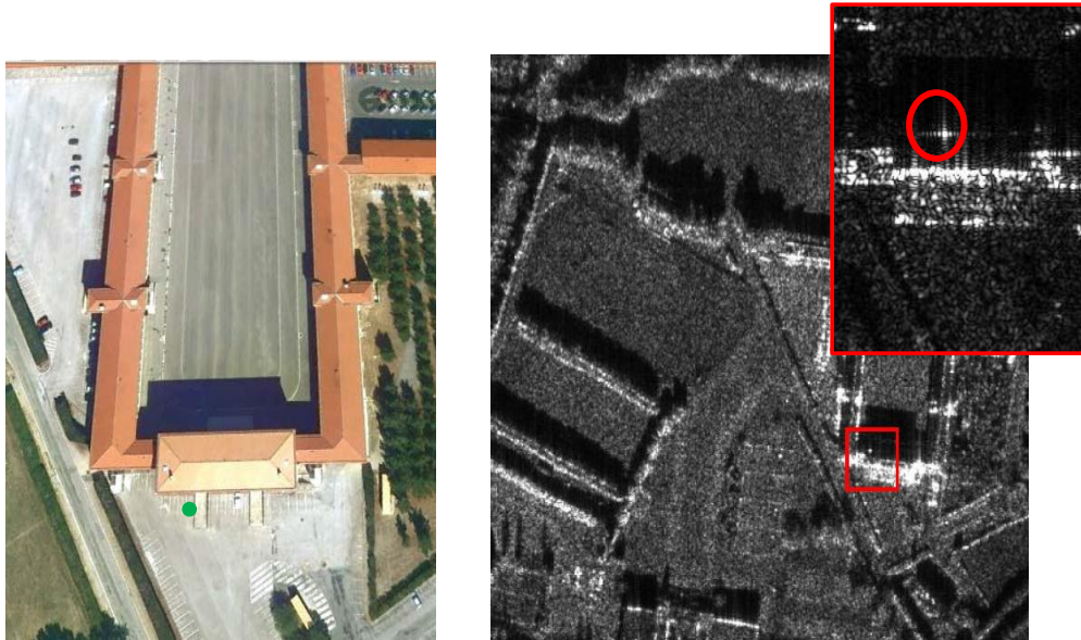
Figure 1.1: (Left) Real building of interest with a target located in front of it (the green point indicates the position of the target). (Right) Corresponding SAR image acquired and processed by ONERA through a measurement campaign involving the BUSARD motor glider platform equipped with the Drive radar. The frequencies band is [33-37] GHz and the incidence angle is 60^\circ . This image contains an artifact: a target located in front of the building is synthesized at the shadow area located behind the building (see the red rectangle).
