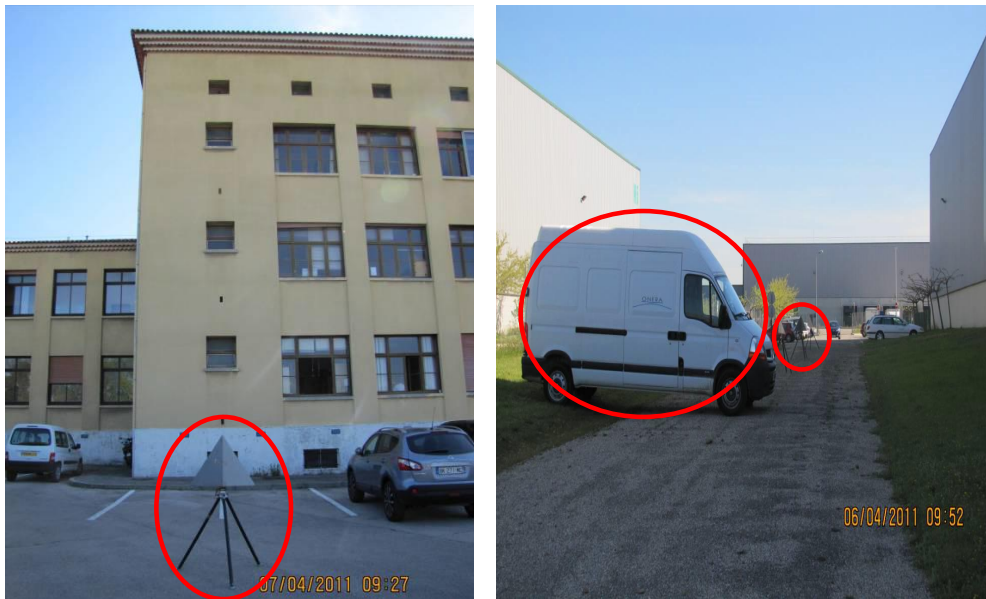
Figure 2.9: (Left) First scene of study: an example of a corner reflector (in red circle) facing the reflector wall of the Air Force Base. (Right) Second scene of study: three corner reflectors and a vehicle (in red circle) are located inside the canyon of interest in the commercial area.
