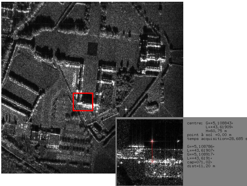
Figure 2.10: SAR image of the first scene of study corresponding to a corner located in front of the building of the Air Force Base. Zoom on the area of interest (red rectangle).
