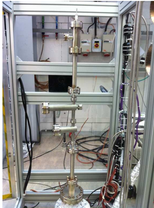
Figure 2.A.2: Vacuum parts being coated with the NEG of TiZrV at a facility in CERN (engineering schemes in fig. 2.A.1). Photo courtesy of Ivo Wevers.
