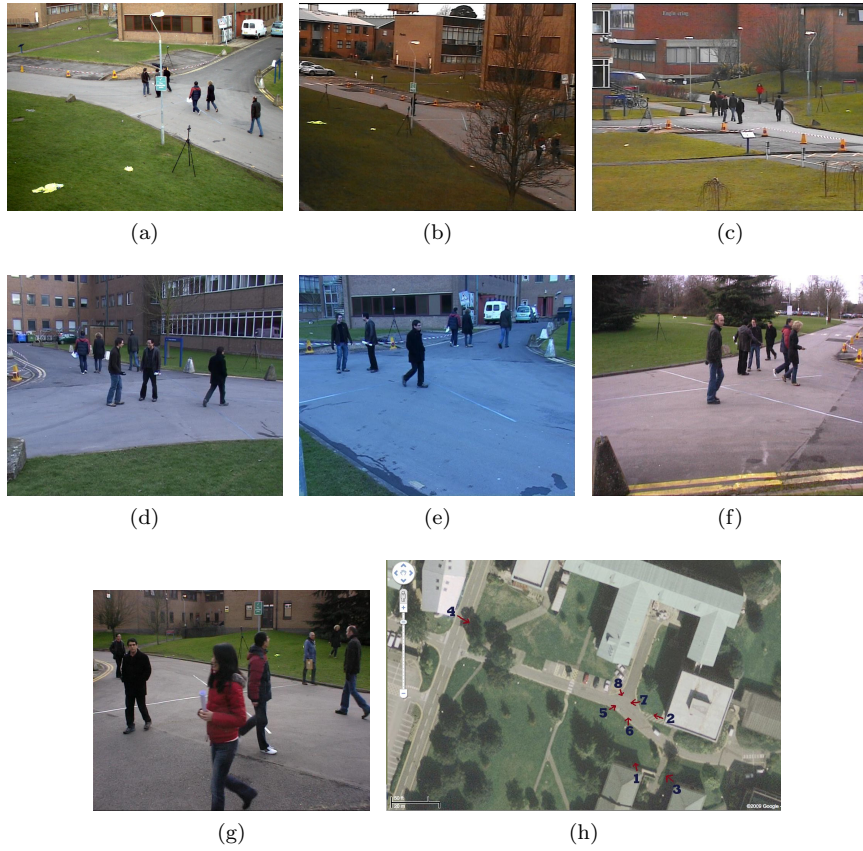
Figure 5.2 Camera views used in the PETS2010 database. We can note that each view emphasizes one or more problem. For example, the first one (a) causes occlusions between persons and the pole while the second one (b) is characterized by several occlusions between persons and the tree. In (h) the position of the cameras on the plane is shown.
