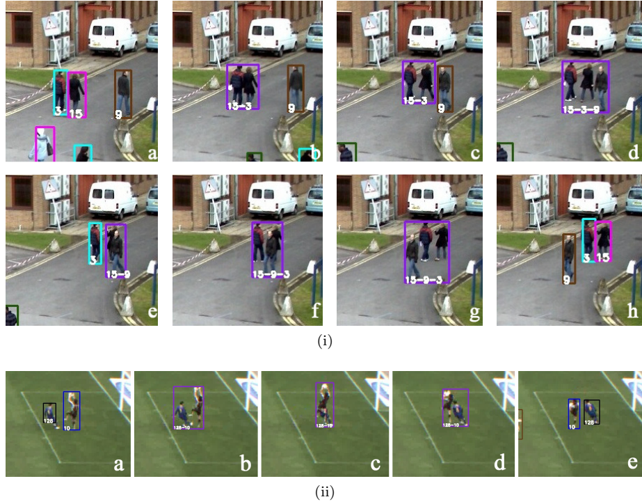
Figure 5.12 The output of the proposed method over two sequences of the PETS 2010 dataset (i) and of the ISSIA Soccer Dataset (ii) containing an occlusion. Note how the object 9 in (i) is correctly tracked inside the different groups although it quickly changes its direction in the frame (c).
