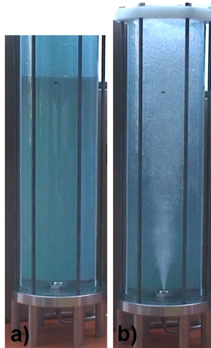
Figure 4.5: a) Water height before gas injection; b) gas coalescence induced by the open surface.
