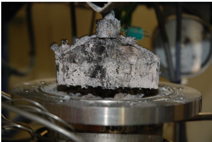
Figure 3.6: A picture of the comb of thermocouples after an experimental test.
