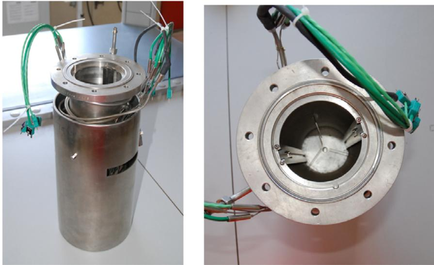
Figure 3.3: The test cell filled with sodium. Inside the cell the rails for the movement of the comb of thermocouples can be seen.
