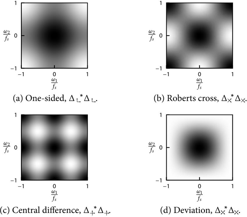
Figure 3: Anisotropies in eigenvalues of discrete two-dimensional Laplacians, derived from various finite differences schemes. Eigenvectors constitute a Fourier basis, so that they are indexed by spatial frequencies  $(\omega_1, \omega_2)$ , normalized by the spatial sampling frequency  $f_s$ . Each colormap is linearly scaled between black (null modulus), and white (highest eigenvalue modulus).
