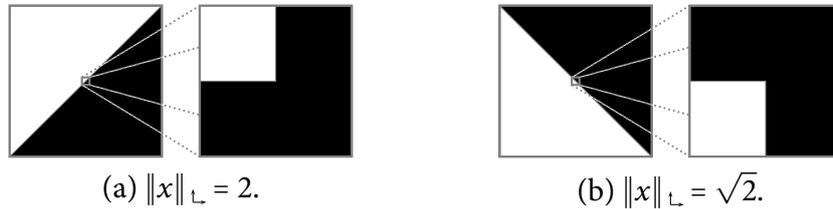
Figure 4: Example of two edge orientations that are weighted differently by one-sided discretization. On each figure, the edge is represented on the left side, and a schematic view of the discretization is shown on the right side. The values of the resulting one-sided TV semi-norms, defined as  $\|x\|_{\mathcal{L}} \stackrel{\text{def}}{=} \sum_p \|(\Delta_{\mathcal{L}}(x))_p\|_2$ , are given after normalization by the side length of the square.
