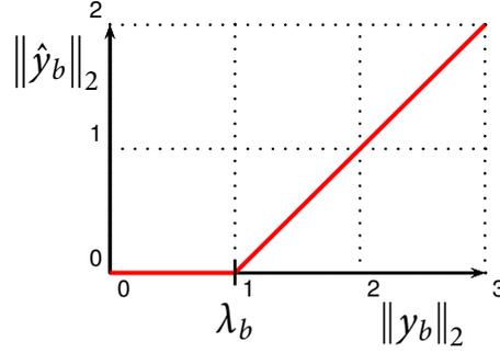
Figure 1: Group soft-thresholding;  $\lambda_b \stackrel{\text{set}}{=} 1$ .
