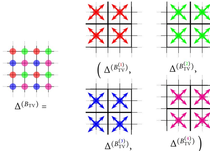
Figure 5: Illustration of the splitting of the deviation spatial gradient in dimension  $D^{\text{set}} = 2$ , into four deviation operators over nonoverlapping block structures. On the left side, each dot is the center of a block of size  $2 \times 2$ ; their color indicates which block grid they belong to in the splitting. We can see that all possible blocks of size  $2 \times 2$  are taken into account.
