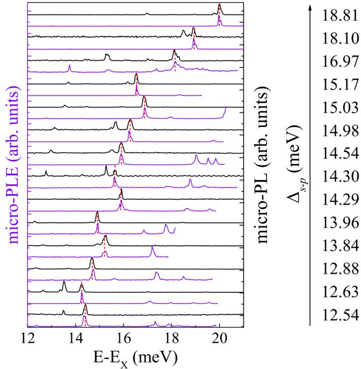
Figure 7.19: The micro-PLE spectra detected on the  $X^{+*}$  emission line (purple curves) and the micro-PL spectra (black curves) of a series of different QDs. The red dashed vertical lines indicate the energy of the resonant peak  $R^*$  and the  ${}^pX^{+*}$  emission line. The scale of the horizontal axis is set by the energy relative to the  $X$  emission line. The spectra are normalized to the most intense peaks and vertically shifted for clarity purpose.
