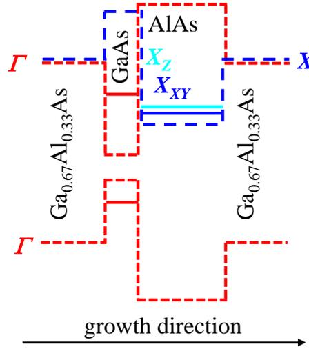
Figure 3.2: Distribution of the energy bands and the position of the confined levels, characteristic of the GaAs/AlAs type II QW structure. Red dashed line -  $\Gamma$ -symmetry band; blue dashed line -  $X$ -symmetry band. The positions of the  $\Gamma$ - and  $X$ -symmetry states in the QW are marked in red and yellow colours, respectively.
