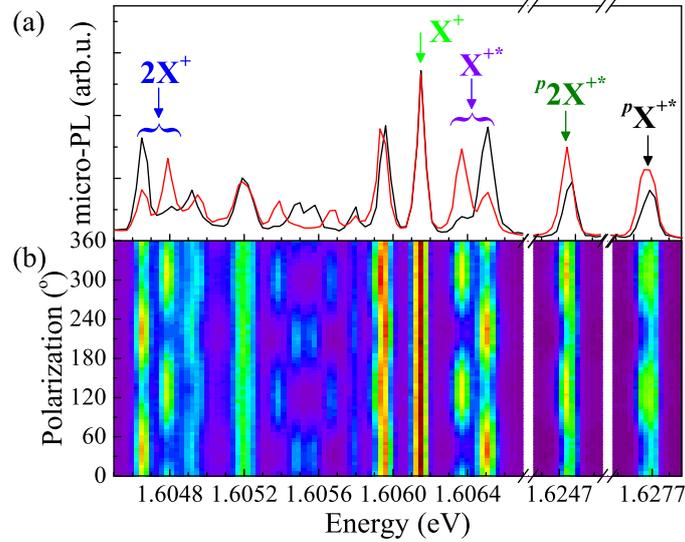
Figure 7.2: (a) The micro-PL spectra of a single GaAlAs QD recorded for two different linear polarizations:  $\pi_x$  (violet curve) and  $\pi_y$  (red curve) oriented along the crystallographic directions  $[110]$  and  $[1\bar{1}0]$ , respectively. (b) Color plot presenting the micro-PL spectra of the same QD measured using different linear polarizations of detection. The  $45^\circ$  and  $135^\circ$  correspond to the crystallographic directions  $[110]$  and  $[1\bar{1}0]$ , respectively.
