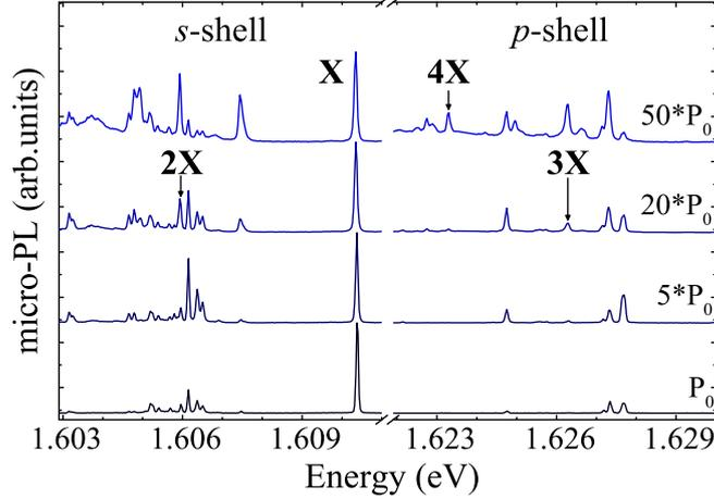
Figure 6.1: The excitation-power evolution of the micro-PL spectra of a single GaAlAs/AlAs QD measured at  $T=4.2 \text{ K}$ . The spectra are excited quasi-resonantly ( $E_{exc}=1.71 \text{ eV}$ ).  $P_0=10 \mu\text{W}$  indicates the excitation power. The spectra are normalized to the intensity of the X emission line and vertically shifted for clarity purpose.
