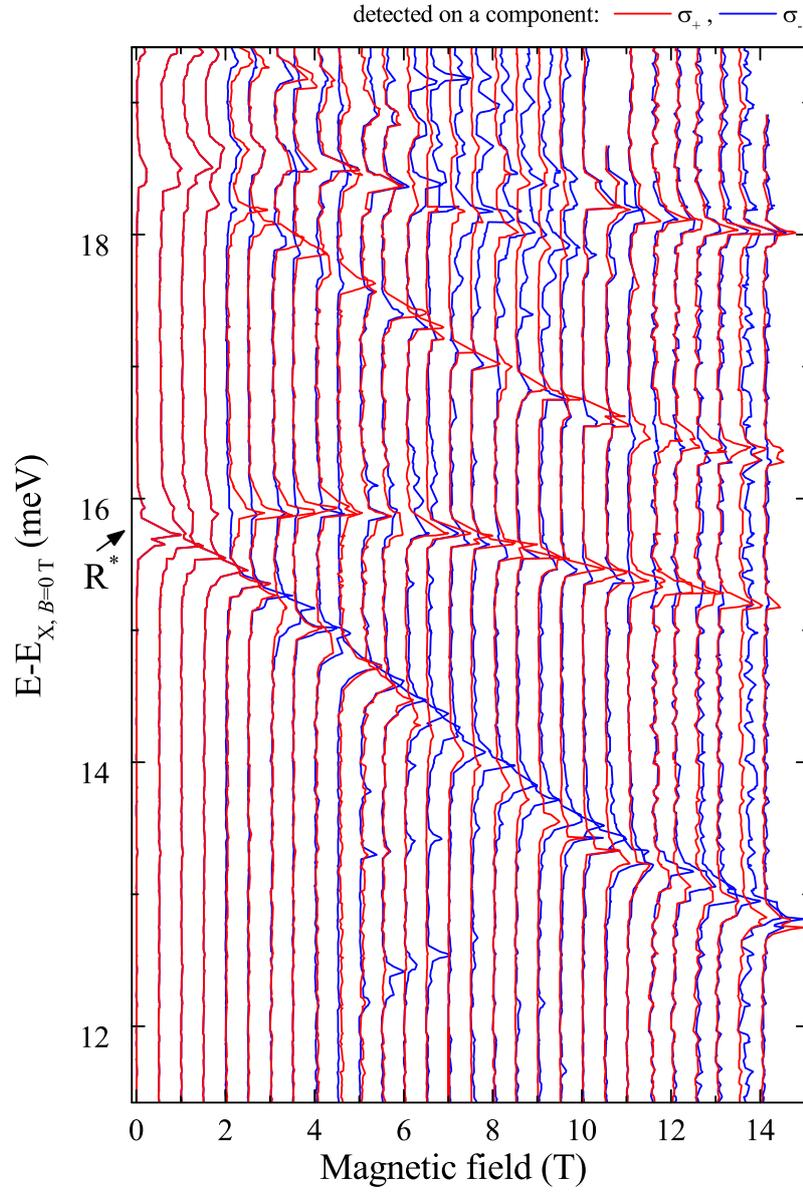
Figure 7.15: The magnetic-field evolution of micro-PL spectra detected on the  $X^{+*}$  emission line (dot with  $\Delta_{s-p}=14.29$  meV). The scale of the horizontal axis is set by the energy relative to the X emission line. The spectra are normalized to the most intense peaks and shifted for clarity purpose.
