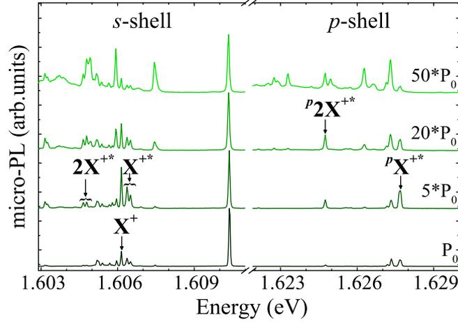
Figure 7.1: The excitation-power evolution of the micro-PL spectra of a single GaAlAs/AlAs QD measured at  $T=4.2$  K. The spectra are excited quasi-resonantly ( $E_{exc}=1.71$  eV).  $P_0=10$   $\mu$ W and indicates the excitation power. The spectra are normalized to the intensity of the X emission line and vertically shifted for clarity purpose.
