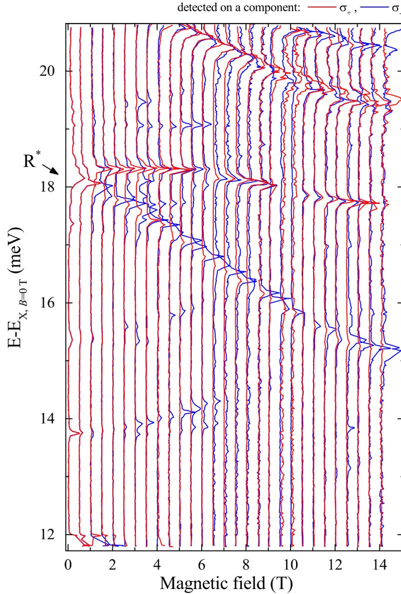
Figure 7.17: The magnetic-field evolution of micro-PLE spectra detected on the  $X^{+*}$  emission line (dot with  $\Delta_{s-p}=16.97$  meV). The scale of the horizontal axis is set by the energy relative to the X emission line. The spectra are normalized to the most intense peaks and shifted for clarity purpose.
