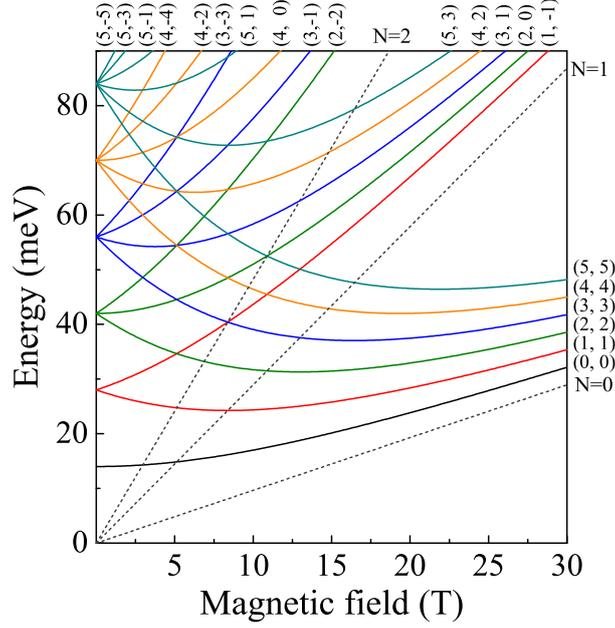
Figure 2.4: Simulated FD spectrum of the first five states in magnetic field for  $\hbar\omega_0=14$  meV and  $\mu^*=0.06 m_0$ . The pairs of values in brackets correspond to the  $(n, m_z)$  quantum numbers. Dashed lines present the evolution of the first three Landau levels (see Eq. 2.6).
