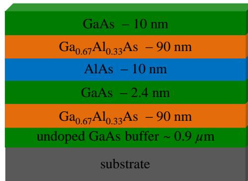
Figure 3.1: The nominal structure of the investigated sample.
