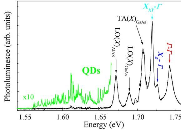
Figure 3.3: A characteristic macro-PL spectrum ( $\sim 1 \text{ mm}^2$  of the laser spot) of the investigated sample.
