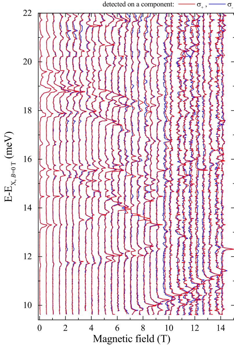
Figure 7.13: The magnetic-field evolution of micro-PL spectra detected on the  $X^+$  emission line (dot with  $\Delta_{s-p}=14.30$  meV). The scale of the horizontal axis is set by the energy relative to the X emission line. The spectra are normalized to the most intense peaks and shifted for clarity purpose.
