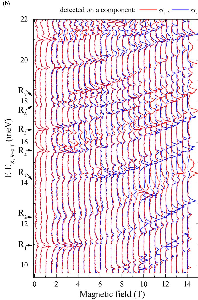
Figure 6.19: The magnetic-field evolution of micro-PL spectra detected on the X emission line (dot with  $\Delta_{s-p}=14.30$  meV). The scale of the horizontal axis is set by the energy relative to the X emission line. The spectra are normalized to the most intense peaks and shifted for clarity purpose.
