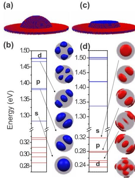
Figure 2.2: (a) lens shaped InAs QD embedded in GaAs matrix, (b) Electron probability density isosurfaces and electron and hole energies for dot (a), (c) disk shaped InAs QD (grown by the indium-flush method [23]), (d) Hole probability density isosurfaces and electron and hole energy shells for dot (c). From Ref. 22.
