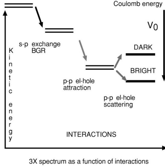
Figure 2.6: Contributions to energy levels and oscillator strength of the triexciton complex. The  $s$  and  $p$  letters describe the electron and hole on the  $s$ - and  $p$  shells, respectively. From Ref. 8.
