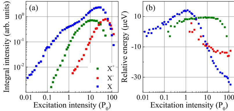
Figure 5.11: The excitation-power dependence of the integrated intensity (a) and the relative energy (b) of three main emission lines:  $X$ ,  $X^-$ , and  $X^+$ . The plots are drawn in the log-log and the semi-log scale, respectively.
