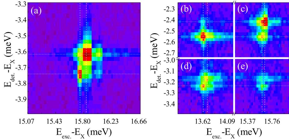
Figure 7.22: The micro-PLE maps measured at: (a) 0 T, (b) - (e) 9 T. The white dashed horizontal (vertical) lines indicate the position of the split components of the  $X^{+*}$  emission line (the resonant peak  $R^*$ ). The excitation/detection polarizations are: (b)  $\sigma_-/\sigma_+$ , (c)  $\sigma_+/\sigma_+$ , (d)  $\sigma_-/\sigma_-$ , (e)  $\sigma_+/\sigma_-$ .
