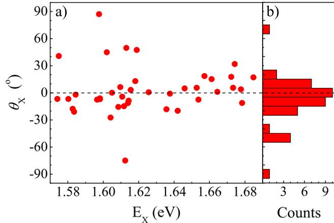
Figure 6.9: (a) The anisotropy axis,  $\theta_X$ , of the neutral exciton state as a function of its energy. (b) A histogram of the  $\theta_X$  obtained for a number of single dots under investigation.  $0^\circ$  indicates the [110] crystallographic direction.
