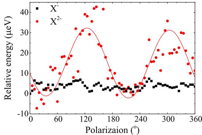
Figure 8.2: The energy of the  $X^-$  and  $X^{2-}$  emission lines as a function of the angle of a polarization analyser (points). The FSS of the  $X^{2-}$  emission line is determined by means of fitting the cosine-squared function (a red solid curve).
