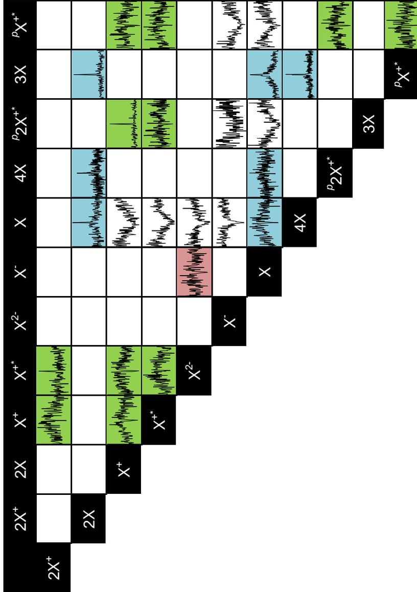
Figure 5.9: The photon auto- and cross-correlation histograms of the excitonic lines related to the  $s$ - and  $p$ -shell of the single QD under quasi-resonant excitation. Colours of background indicate the cross-correlations between emissions from the same family: blue - neutral, green - positively charged, red - negatively charged.
