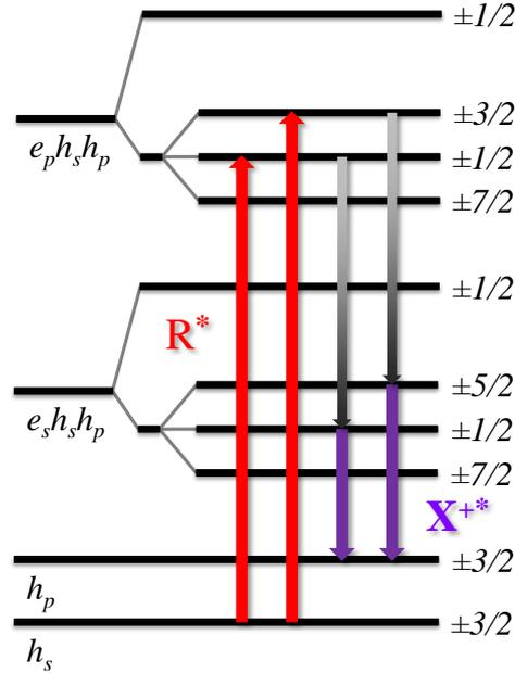
Figure 7.23: Theoretical structure (not to scale) of two states related to the resonant peak  $R^*$  and the  $X^{+*}$  emission line. The symbols  $e_s$  ( $h_s$ ) and  $e_p$  ( $h_p$ ) denote the electron (hole) occupying the  $s$ - and  $p$ -shell, respectively. The half-integers are the projections  $J_z = J_z^e + J_z^h$  of the total momentum.
