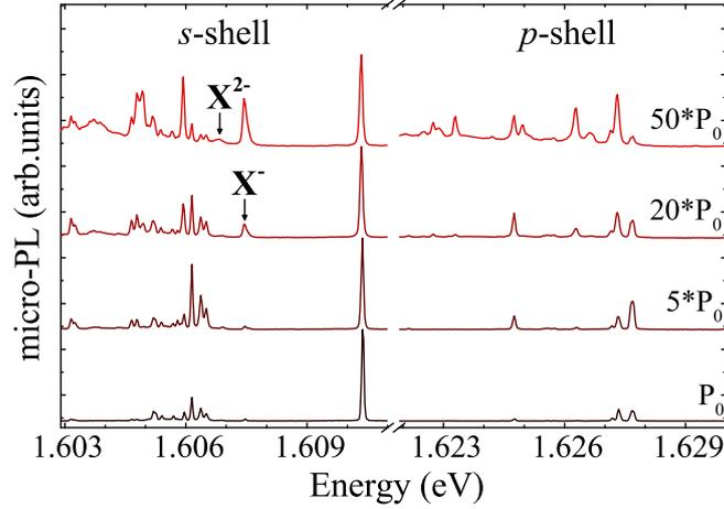
Figure 8.1: The excitation-power evolution of the micro-PL spectra of a single GaAlAs/AlAs QD measured at  $T=4.2$  K. The spectra are excited quasi-resonantly ( $E_{exc}=1.71$  eV).  $P_0=10$   $\mu$ W and indicates the excitation power. The spectra are normalized to the intensity of the X emission line and vertically shifted for clarity purpose.
