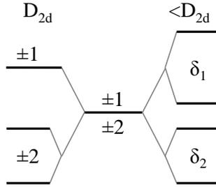
Figure 2.8: Scheme of the neutral exciton fine structure at zero magnetic field. The central part of the figure illustrates the situation when the  $eh$  exchange interaction is neglected ( $M = \pm 1$  and  $M = \pm 2$  are degenerate). The left panel shows the excitonic fine structure for QDs with  $D_{2d}$  symmetry, while the right panel accounts for dots with a symmetry lower than  $D_{2d}$ .
