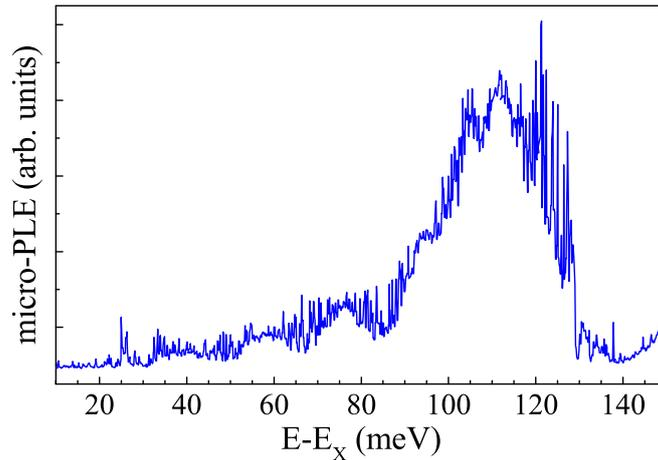
Figure 6.14: Micro-PLE spectrum of a single dot detected on the X emission line (dot with  $\Delta_{s-p}=12.63$  meV). The scale of the horizontal axis is set by the energy relative to the X emission line.
