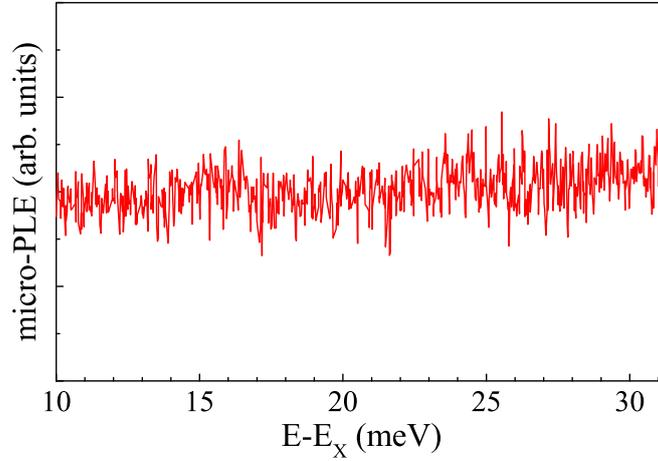
Figure 8.3: Micro-PLE spectrum detected at the energy of the recombination of the negatively charged exciton.  $\Delta_{s-p} = 14.30$  meV. The scale of the horizontal axis is set by the energy relative to the X emission line.
