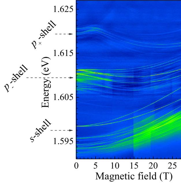
Figure 5.4: The evolution of the micro-PL spectrum of the highly excited GaAlAs/AlAs QD ( $E_{exc}=1.71$  eV) in the magnetic field up to 28 T. The background intensity variation is an artifact resulting from the procedure described at the beginning of this Section.
