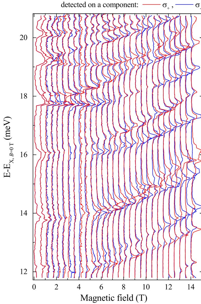
Figure 6.21: The magnetic-field evolution of micro-PL spectra detected on the X emission line (dot with  $\Delta_{s-p}=16.97$  meV). The scale of the horizontal axis is set by the energy relative to the X emission line. The spectra are normalized to the most intense peaks and shifted for clarity purpose.
