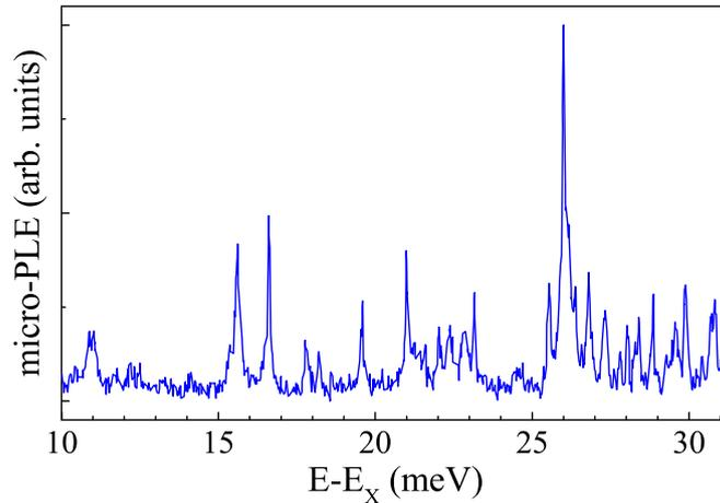
Figure 6.15: Micro-PLE spectrum of a single GaAlAs QD detected on the X emission line (dot with  $\Delta_{s-p}=14.30$  meV). The scale of the horizontal axis is set by the energy relative to the X emission line.
