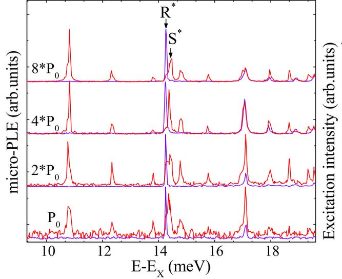
Figure 7.11: The excitation-power evolution of micro-PL spectra detected on the  $X^+$  (red curves) and the  $X^{+*}$  (violet curves) emission lines (dot with  $\Delta_{s-p}=12.63$  meV). The scale of the horizontal axis is set by the energy relative to the  $X$  emission line. The spectra are normalized to the most intense peaks and vertically shifted for clarity purpose.
