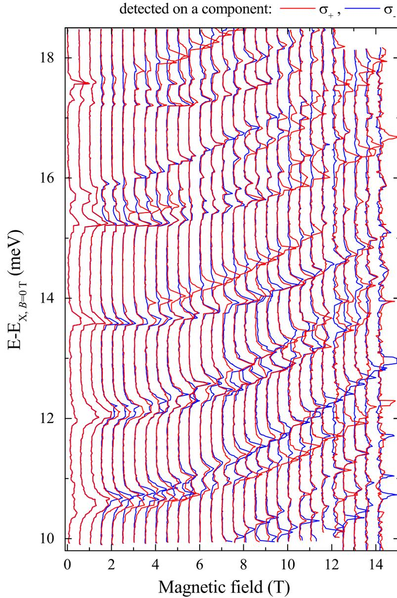
Figure 6.20: The magnetic-field evolution of micro-PLE spectra detected on the X emission line (dot with  $\Delta_{s-p}=12.24$  meV). The scale of the horizontal axis is set by the energy relative to the X emission line. The spectra are normalized to the most intense peaks and shifted for clarity purpose.
