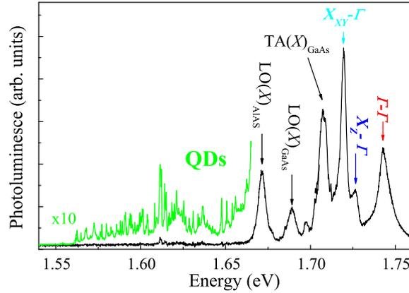
Figure 5.1: The PL spectrum of a 1 mm size area of the investigated sample measured at  $T=4.2$  K.
