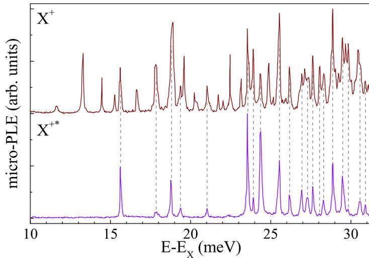
Figure 7.8: Micro-PL spectra of a single dot detected on the  $X^+$  and  $X^{+*}$  emission lines (dot with  $\Delta_{s-p}=14.30$  meV). The grey vertical dashed lines indicate the energy of resonant peaks associated with the  $X^{+*}$  line. The scale of the horizontal axis is set by the energy relative to the  $X$  emission line. The spectra are normalized to the most intense peaks and vertically shifted for clarity purpose.
