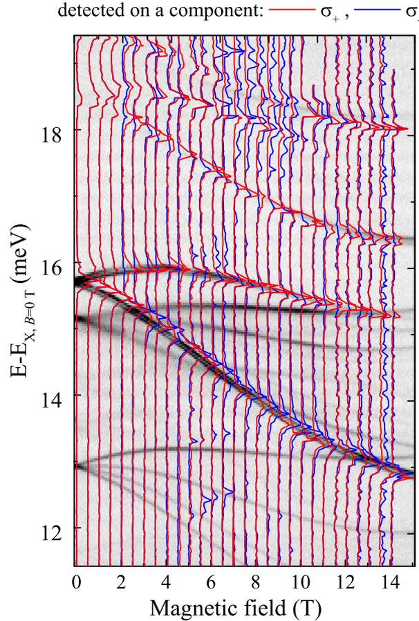
Figure 7.20: The magnetic-field evolution of the micro-PL spectra detected on the  $X^{+*}$  emission line (the blue and red curves), superimposed on a gray-scale map displaying the micro-PL spectra of the same dot, plotted as a function of the magnetic field.  $\Delta_{s-p}=14.29$  meV. The scale of the horizontal axis is set by the energy relative to the X emission line. The spectra are normalized to the most intense peaks and vertically shifted for clarity purpose.
