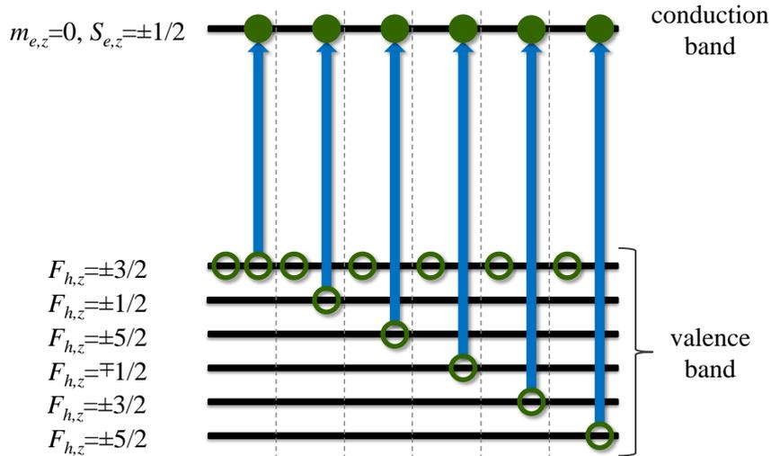
Figure 7.18: Black horizontal lines illustrate the ladders of levels in the conduction and valence bands. The blue (red) arrows indicate the possible absorption transitions between the valence band levels and the  $s$ -shell ( $p$ -shell), respectively.
