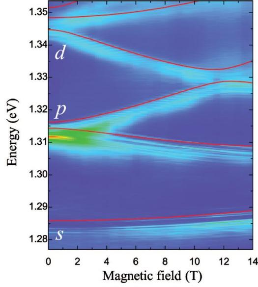
Figure 2.5: Luminescence from the  $s$ -,  $p$ -, and  $d$ -shell of the single InAs/GaAs QD at magnetic field up to 14 T. Red lines represent the simulation based on the excitonic Fock-Darwin diagram. From Ref. 10.
