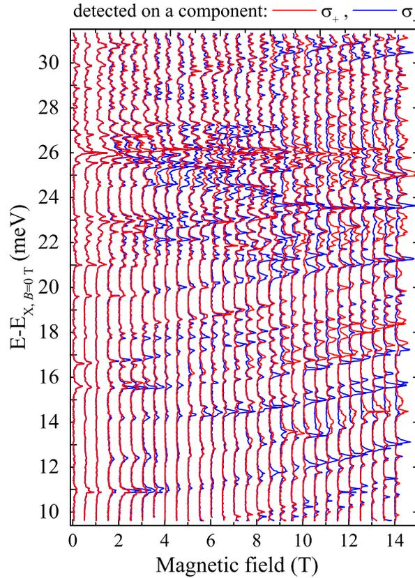
Figure 6.18: The magnetic-field evolution of micro-PLE spectra detected on the X emission line (dot with  $\Delta_{s-p}=14.30$  meV). The scale of the horizontal axis is set by the energy relative to the X emission line. The spectra are normalized to the most intense peaks and shifted for clarity purpose.
