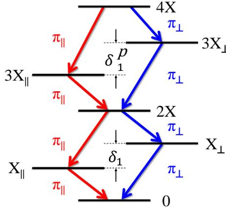
Figure 6.5: Schematic diagram of the cascade decay of a quadexciton in a single QD. The solid blue (red) arrows denote the radiative transitions in two perpendicular polarizations. The  $\pi_{||}$  and  $\pi_{\perp}$  are the parallel and perpendicular linear polarizations with respect to  $[110]$  crystallographic direction, respectively.
