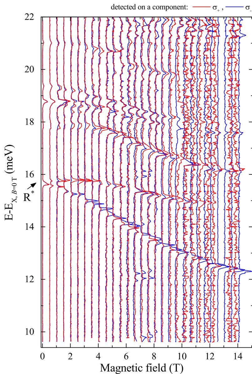
Figure 7.16: The magnetic-field evolution of micro-PL spectra detected on the  $X^{+*}$  emission line (dot with  $\Delta_{s-p}=14.30$  meV). The scale of the horizontal axis is set by the energy relative to the X emission line. The spectra are normalized to the most intense peaks and shifted for clarity purpose.
