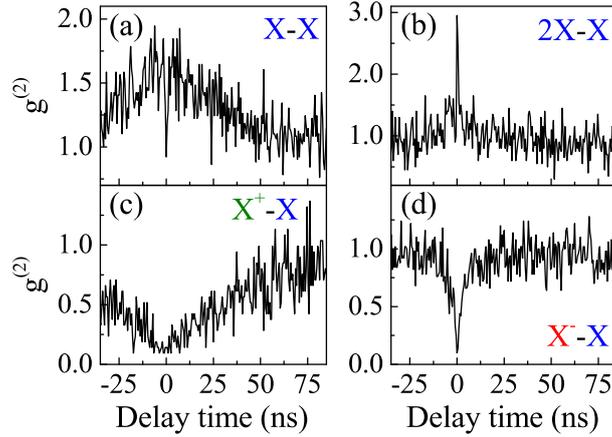
Figure 5.8: A set of correlation histograms: (a) an auto-correlation on the X emission line, (b)-(d) cross-correlations between the 2X and X, the X<sup>+</sup> and X, and the X<sup>-</sup> and X emission lines, respectively. The histograms (a) and (c) were measured at  $P_{exc}=50 \mu\text{W}$  whereas (b) and (d) at  $P_{exc}=500 \mu\text{W}$ .
