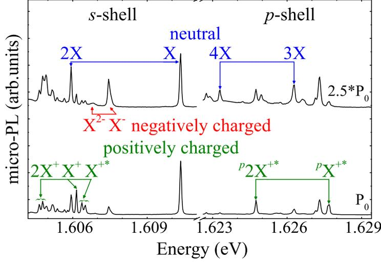
Figure 5.7: The micro-PL spectra of a single GaAlAs/AlAs QD, excited quasi-resonantly at  $E_{exc}=1.71$  eV and measured at  $T=4.2$  K for two different excitation powers:  $P_0=200$   $\mu$ W and  $2.5 \cdot P_0$ . The spectra are normalized to the intensity of the X emission line and vertically shifted for clarity purpose.
