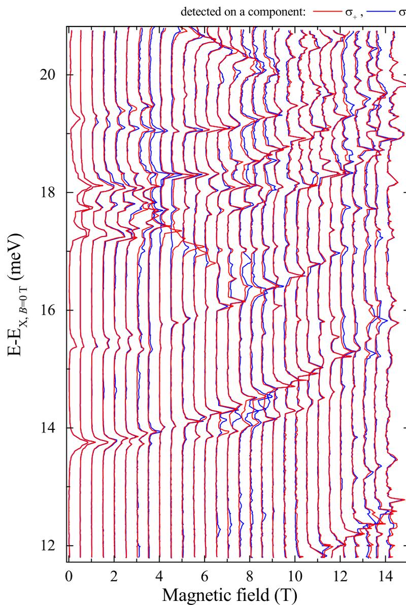
Figure 7.14: The magnetic-field evolution of micro-PL spectra detected on the  $X^+$  emission line (dot with  $\Delta_{s-p}=16.97$  meV). The scale of the horizontal axis is set by the energy relative to the X emission line. The spectra are normalized to the most intense peaks and shifted for clarity purpose.
