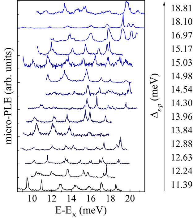
Figure 6.16: Micro-PL E spectra detected on the X emission line, measured for a series of QDs characterized by different amplitude of  $\Delta_{s-p}$ . The scale of the horizontal axis is set by the energy relative to the X emission line. The spectra are normalized to the most intense peaks and vertically shifted for clarity purpose.
