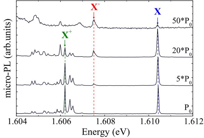
Figure 5.10: The excitation-power evolution of the micro-PL spectra of a single GaAlAs/AlAs QD measured at  $T=4.2$  K. The spectra are excited quasi-resonantly ( $E_{exc}=1.71$  eV).  $P_0=10$   $\mu$ W and indicates the excitation power. The spectra are normalized to the intensity of the X emission line and vertically shifted for clarity purpose.
