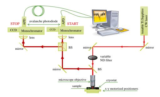
Figure 4.3: Scheme of the photon correlation experimental setup.
