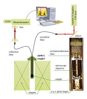
Figure 4.2: The scheme of the micro-PL setup used for measurements in magnetic fields. An inset photo comprising of a microscope objective and piezoelectric x-y-z stages with the sample.
