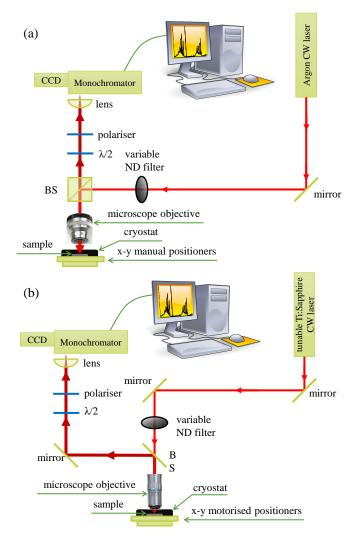
Figure 4.1: Scheme of micro-photoluminescence setups available in: (a) Faculty of Physics, University of Warsaw, (b) Grenoble High Magnetic Field Laboratory.
