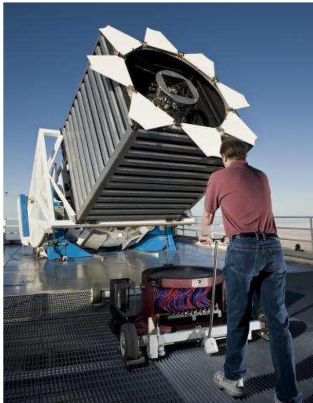
FIGURE 2.5: The cartridge is brought to the 2.5 m SDSS telescope and installed on the focal plane. (Figure from [www.sdss3.org](http://www.sdss3.org).)
