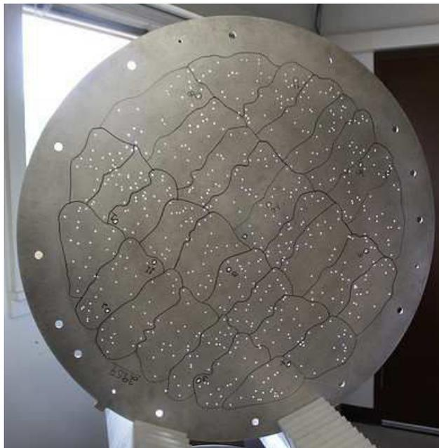
FIGURE 2.3: An example of a BOSS plate drilled and waiting to be observed. The aluminum plates are  $\frac{1}{8}$  in. thick with a 32 in. diameter. (Figure from [www.sdss3.org](http://www.sdss3.org).)
