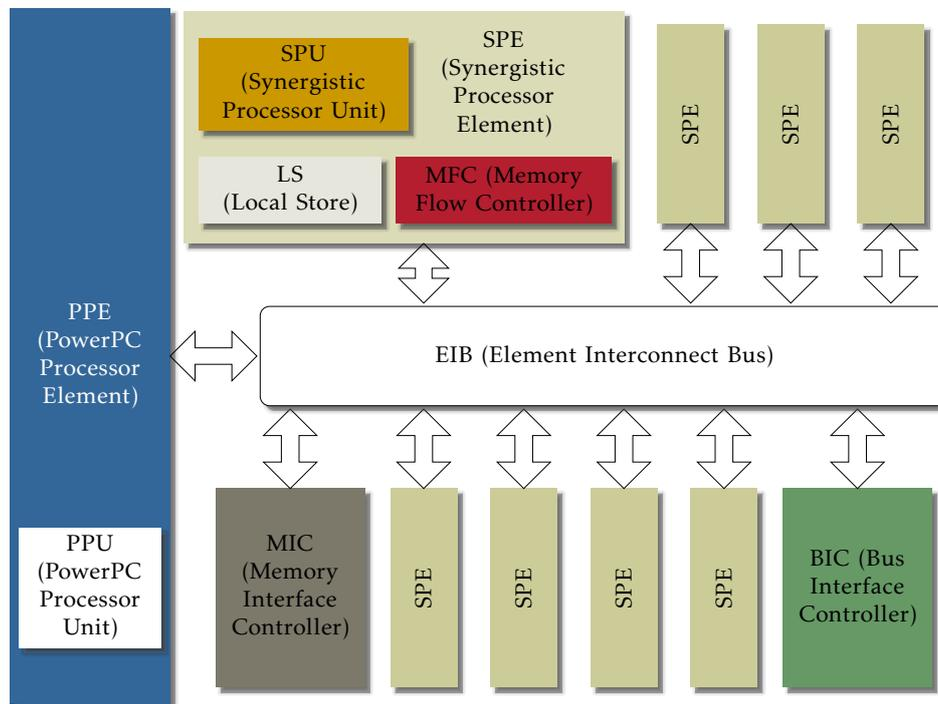
Figure 3.4 – IBM Cell BE processor
