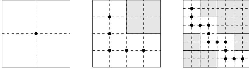
Figure 4.4 – Exploring the cost space via grid refinement. The dark points indicate the new candidates for exploration after each refinement.
