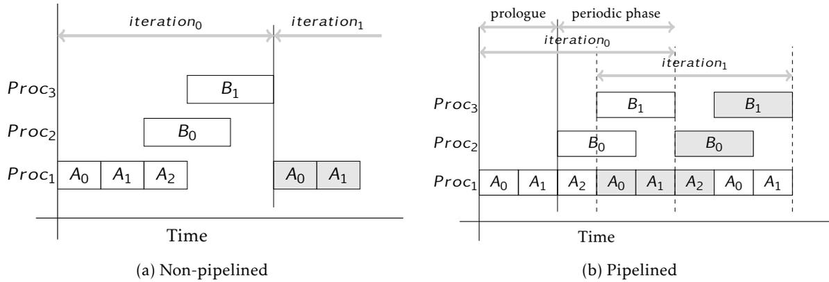
Figure 2.5 – Example schedule of a Synchronous DataFlow graph
