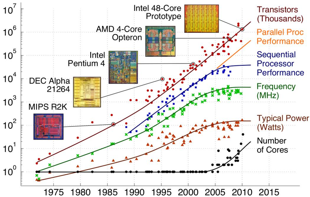
Figure 1.1 – Evolution of multi-core processors <sup>1</sup>
