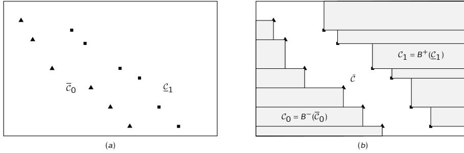
Figure 4.3 – (a) Sets  $\mathcal{C}_0$  (**unsat**) and  $\mathcal{C}_1$  (**sat**) represented by their extremal points  $\bar{c}_0$  and  $c_1$ ; (b) The state of our knowledge at this point as captured by  $\mathcal{C}_0$  (infeasible costs)  $\mathcal{C}_1$  (feasible costs) and  $\tilde{\mathcal{C}}$  (unknown). The actual Pareto front is contained in the closure of  $\tilde{\mathcal{C}}$ .
