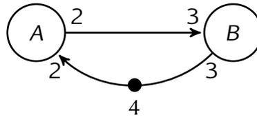
Figure 2.3 – SDF with backward edge
