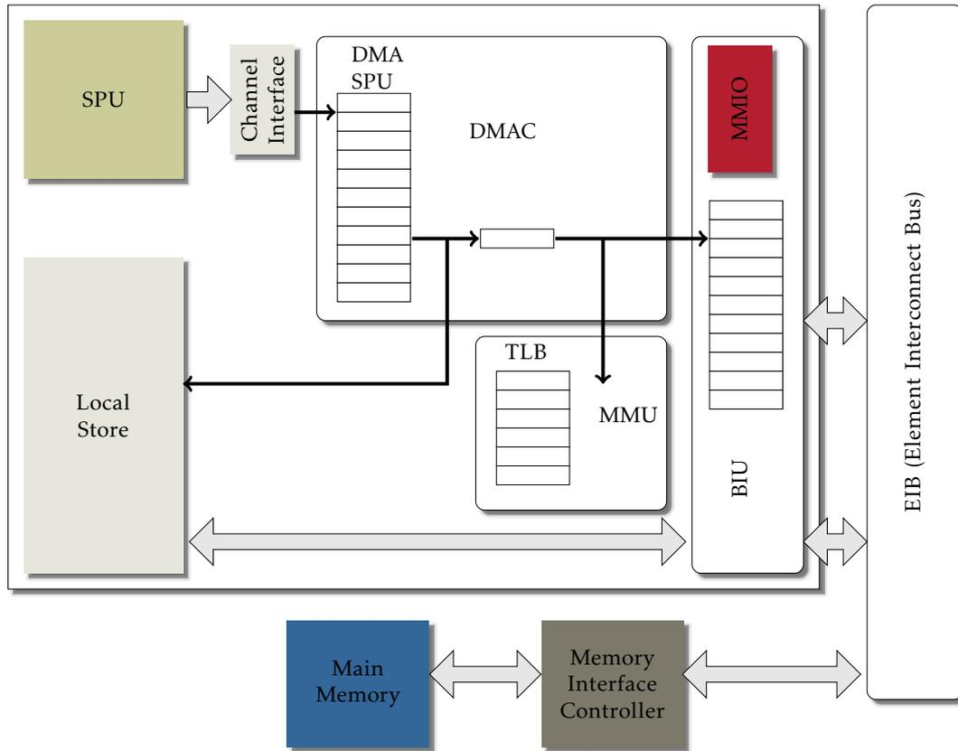
Figure 3.5 – IBM Cell processor DMA controller
