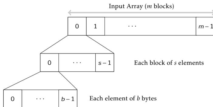
Figure 8.5 – Decomposition of one dimensional input array
