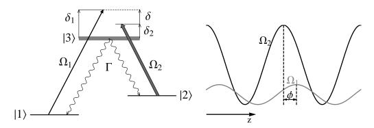
Figure 3.4: The  $\Lambda$  scheme, a simplification of the <sup>7</sup>Li level structure, used to understand the effect of the Raman configuration. The cooling (repumping) light is represented by a standing wave with Rabi frequency  $\Omega_2(z)$  ( $\Omega_1(z)$ ).
