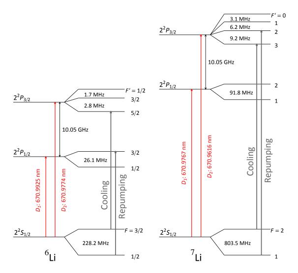
**Figure 2.1:** Level schemes of  ${}^{7}$ Li and  ${}^{6}$ Li, the most accurate measurements of the optical transitions, fine and hyperfine splittings can be found in [*Sansonetti et al., 2011*]. Note the near perfect tuning between the  ${}^{7}$ Li  $D_{1}$  and  ${}^{6}$ Li  $D_{2}$  lines. The transitions used for cooling and repumping in the magneto-optical trap are indicated in grey, see main text.
