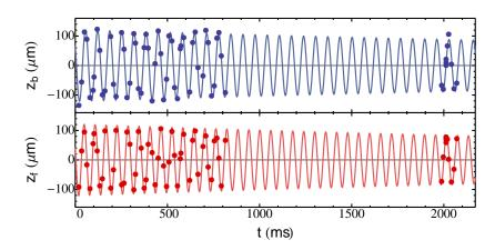
**Figure 5.8:** Center-of-mass motion of a  $^7$ Li cloud (blue circles) and a  $^6$ Li cloud (red circles) in a double superfluid at  $860\,\mathrm{G}$ . The solid lines show fit to the data with exponentially damped sinusoids, yielding a damping rate  $\gamma \leqslant 0.1\,\mathrm{s}^{-1}$ . The very-long lifetime of these oscillations show the superfluid character of our mixture.
