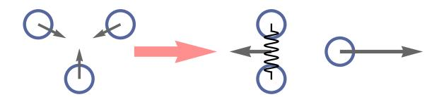
**Figure 4.1:** Schematical representation of a three-body recombination event. Left, initial state of a 3-body collision involving 3 free atoms. Right, final state corresponding to an inelastic collision forming a free atom and a bound dimer (represented by the spring). Both products carry the binding energy of the dimer as kinetic energy.
