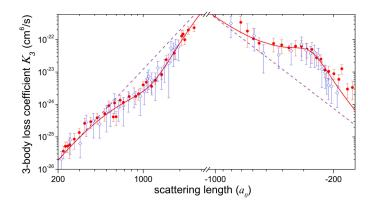
**Figure 4.2:** Three body recombination constant  $L_3$  (called here  $K_3$ ) as a function of a through a Feshbach resonance, from [*Gross et al., 2010*]. Blue and red points show the experimental data. The dashed purple lines show the underlying  $a^4$  scaling and the solid red line show the theory from a solution of the three-body problem, see main text below.
