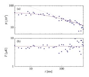
FIG. 1 (color online). Time dependence of the atom number (a) and temperature (b) for  $U = \eta k_B T$ , with  $T = 5.2(4) \mu K$ ,  $\eta = 7.4$ , and (uncorrected)  $L_3 = 1.2(2)_{\rm stat} \times 10^{-21} {\rm cm}^6 {\rm s}^{-1}$ . The dotted line shows the long time  $t^{-1/2}$  dependence of the number of atoms.
