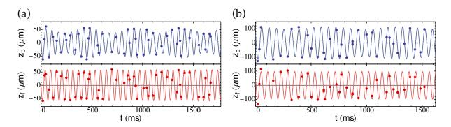
**Figure 5.13:** Coupled dipole oscillations of the Bose-Fermi superfluid mixture (top:  $^{7}$ Li, bottom:  $^{6}$ Li) at different magnetic fields: (a):  $790 \, \text{G}$ , on the BEC side of the crossover, (b):  $860 \, \text{G}$  on the BCS side. The efficiency of the coherent energy exchange varies in the crossover due to a variation of the coupling.
