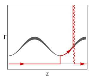
**Figure 3.1:** A grey molasses cycle. The bright state is dressed by the light standing wave, with a space variation of the light-shift and optical-pumping rate (linewidth), represented here for a wave with  $\delta>0$ . First the atom is coupled from a dark state to a bright state at a minimum of the potential created by the light shift. Second it climbs up a potential hill before being pumped back to a dark state through the excited state.
