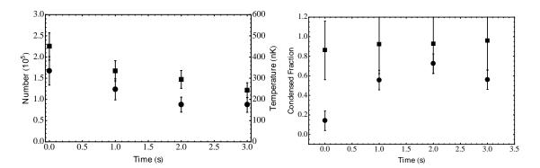
**Figure 2.9:** <sup>7</sup>Li thermalization dynamics after a fast evaporation (2 s) to a trap depth ( $U_0 \simeq 2 \,\mu {\rm K}$ ). Left: temperature (squares) and number (circles) as a function of time. Right: condensed fraction  $N_0/N$  as a function of time, comparison between the measured one (circles) and the one calculated from temperatures and numbers (squares).
