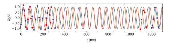
**Figure 5.10:** Center-of-mass motion of a  $^7$ Li cloud (blue circles) and a  $^6$ Li cloud (red squares) in the absence of the other species. The solid lines show sine fit to the data allowing to measure,  $\omega_b=2\pi\times 15.68$ ,  $\omega_f=2\pi\times 17.14$  with a ratio in agreement with the expectations of 1.1 for the magnetic trap.
