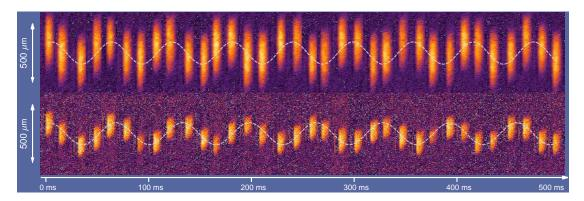
**Figure 5.7:** Motion of the two superfluids ( $^{6}$ Li top,  $^{7}$ Li bottom) in the presence of each other for the first  $500 \, \text{ms}$  with a picture every  $15 \, \text{ms}$ . The dashed white lines are guide to the eye.
