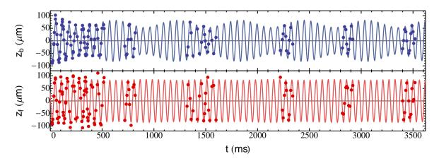
**Figure 5.12:** Coupled dipole oscillations of the Bose-Fermi superfluid mixture, top:  $^{7}$ Li, bottom:  $^{6}$ Li. Data taken at  $835\,G$  close to unitarity. The coherent energy exchange between the two superfluids and the very weak damping are clearly observed.
