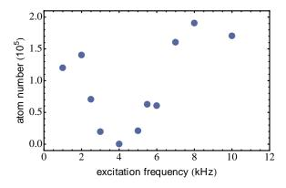
**Figure 2.13:** Atom number left in the dipole trap after a parametric excitation, for a trap depth of  $U_0 \simeq 12 \, \mu {
