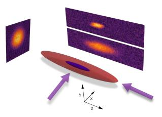
**Figure 2.10:** Schematic representation of the imaging system. The imaging directions are indicated by the purple arrows, we show three different optical density images, obtained from a Bose-Fermi mixture. A BEC of in the  $|2_b\rangle$  state is imaged in the radial direction, together with one spin-state of a degenerate Fermi gas, the other fermions spin state is imaged in time of flight in the axial direction.
