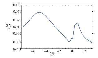
FIG. 8. (Color online) Continued fractions solution of the photon scattering rate  $\Gamma' = \Gamma \, \rho_{33}$  averaged over all relative phases of the repumper and principal standing waves as a function of the two-photon detuning  $\delta$ . Velocity-dependent effects are taken into account here by computing an average of  $\langle \Gamma' \rangle_{\phi}(v)$  weighed by a Maxwell-Boltzmann velocity distribution at 200  $\mu$ K.
