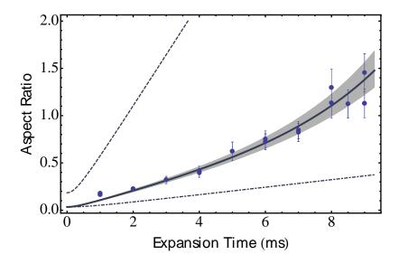
**Figure 5.4:** Aspect ratio of a  $^7$ Li BEC after release from the radial confinement. The solid line shows the result from the hydrodynamic equations with no fit parameters using our trap frequencies and the shaded region shows the uncertainty resulting from the uncertainty on the frequencies. The dashed line shows the solution of the Schrödinger equation of an expanding wave packet, the dot-dashed line that of a Boltzmann gas at  $100\,\mathrm{nK}$ .
