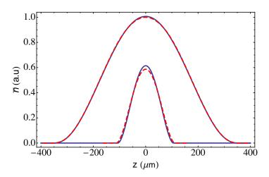
**Figure 5.2:** Theoretical doubly integrated density profiles of the bosons and one spin state of the fermions, at  $B=832\,\mathrm{G}$  obtained using LDA with  $N_{\mathrm{f}}=300\times10^3$  balanced fermions, and  $N_{\mathrm{b}}=30\times10^3$  bosons. Solid blue lines: theory neglecting the interspecies interaction. Red dashed lines: theory with the same atom numbers taking the Bose-Fermi coupling into account, see main text.
