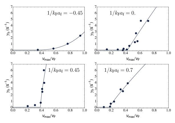
**Figure 5.20:** Damping of the BEC motion as a function of the relative velocity for four different points in the BEC-BCS crossover. On the BEC side and at unitarity ( $1/k_Fa_f \geqslant 0$ ), a sharp onset of damping is observed for increasing velocity, while friction is strongly reduced on the BCS side. The solid lines are fits with the ad-hoc function (5.46).
