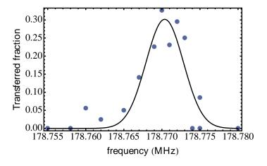
**Figure 2.14:** Example of magnetic field measurement by radio-frequency transfer from the  $|1_b\rangle$  state to the  $|2_b\rangle$  state by monitoring the population transfer. The central frequency is extracted by a gaussian fit to the data, yielding here a magnetic field  $B=837.5(1)\,\mathrm{G}$ .
