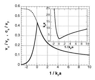
**Figure 1.5:** Critical velocity for (solid line) a Fermi gas as a function of  $1/k_{\rm F}a$  calculated using (1.58) and the dispersion relations for the elementary excitations as obtained in [Combescot et al., 2006]. The sound velocity on the BCS side is shown in dashed line. (The inset shows the healing length of a Fermi superfluid in the crossover.)
