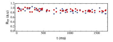
**Figure 5.16:** Time evolution of the Thomas-Fermi radius of the  $^{7}$ Li BEC (blue circles) and the  $^{6}$ Li Fermi superfluid (red squares) during dipole oscillations at  $790\,\mathrm{G}$  rescaled in arbitrary units. The absence of measurable periodic pattern suggests that no other collective modes than the dipole modes are excited. A weak decrease of both radii is due to residual atom loss during the oscillations.
