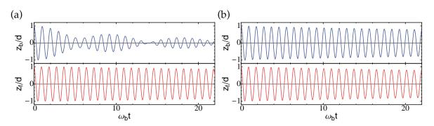
**Figure 5.22:** Numerical solution to the coupled oscillators model with a friction force  $f=-\alpha\,v$  between the two oscillators. The two cases are  $\alpha=0.2\,\omega_{\rm b}M_{\rm b}$  (a),  $\alpha=5\,\omega_{\rm b}M_{\rm b}$  (b). As the friction is increased (between (a) and (b)), the damping of the light oscillator (top) decreases, due to a frequency and phase-locking of the two oscillators.
