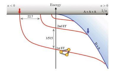
**Figure 4.3:** Representation of the energy of the Efimov trimers (ET) (red solid lines) and of the universal dimer (blue) as a function of 1/a taken from [Ferlaino et al., 2011]. The resonances in three-body recombination happen when the energy of a trimer meets the free atom continuum on the a<0 side (red arrow) and when it joins the dimer energy on the a>0 side (blue arrow). This picture was derived by V. Efimov.
