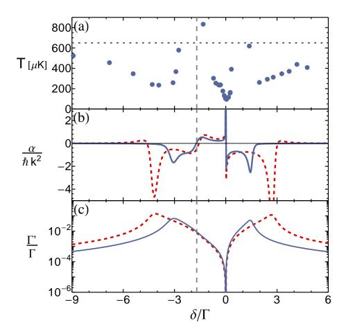
**Figure A.2:** Cooling efficiency as a function of the repumper detuning  $\delta$ . Same as figure 3.5 but with  $\delta_2=2\pi\times 10\,\mathrm{MHz}$ .
