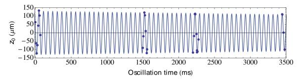
**Figure 2.12:** Oscillation of a BEC in the ODT in the axial direction. The fit by a damped sine function shows excellent agreement, with a long damping time ( $\geqslant 20\,\mathrm{s}$ ), showing the high harmonicity of the magnetic confinement.
