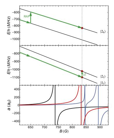
**Figure 2.7:** Schematic representation of the preparation sequence for the superfluid mixture. Top panel, magnetic field dependence of the <sup>7</sup>Li energy levels and the sequence `trajectory' in green arrows. Middle panel, same for <sup>6</sup>Li.
