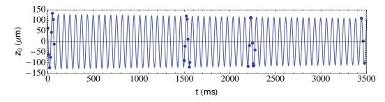
**Figure 5.11:** Long time oscillations of  $^7$ Li alone allowing for a precise frequency measurement. The long damping time observed  $\tau \gtrsim 20\,\mathrm{s}$  shows the high quality factor of the magnetic trapping in the axial direction.
