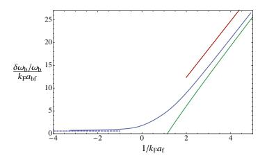
**Figure B.3:** Predicted frequency shift (blue line) over a broad range of  $1/k_{\rm F}a_{\rm f}$ . The dashed blue line shows the ideal Fermi gas limit. On the BEC side the green line shows the Lee-Huang-Yang prediction (B.8) and the red line the mean-field prediction.
