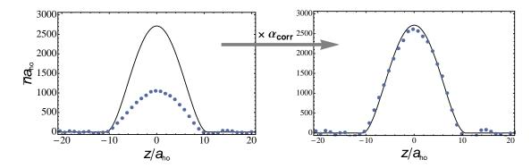
**Figure 2.11:** Calibration of the doubly integrated density for the  $|2_b\rangle$  state: the left picture shows data points obtained by an integration of the optical density measured, the black curve is the theoretical profile that is calculated from the extent of the cloud (Thomas-Fermi radius), the trap frequencies and the scattering length. Using this curve we correct our doubly integrated density (right).
