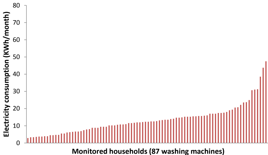
Figure 5.14 : Energy consumption of washing machines for each monitored household (Enertech et al., 2008)
