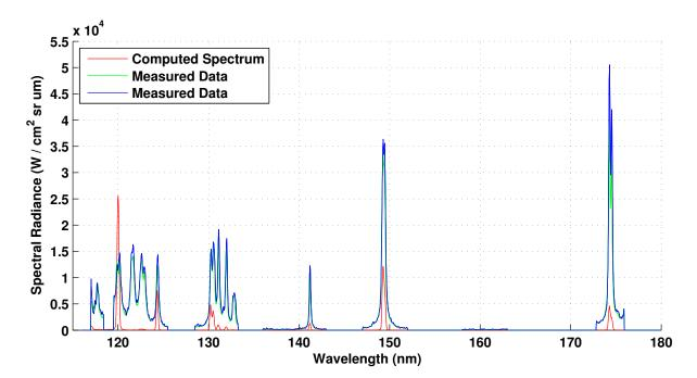
Figure 5.8: Computed and experimentally measured through surface spectra for condition 2.
