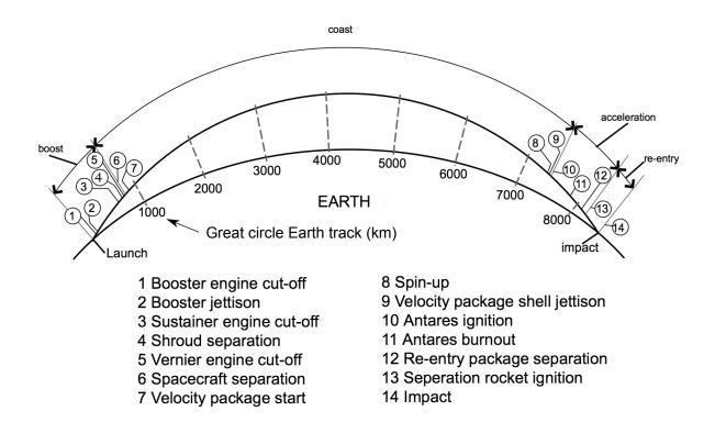
Figure 3.1: FIRE II mission trajectory. Adapted from [23]
