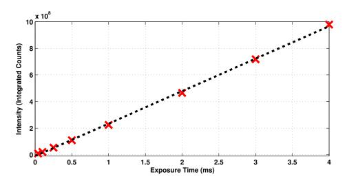
Figure 4.28: Linear response of the camera with variation in exposure time of the ICCD
