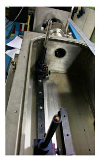
Figure 4.19: (Left) - Alignment tool mounted onto the edges of the flat model.(Right) - Installation of railings in the optical chamber and the mounting poles used in the alignment process.
