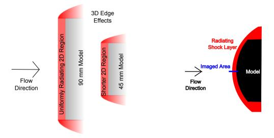
Figure 4.12: Self-absorption experiments concept, top down view (left). Area imaged spatially onto spectrometer when looking across the cylinder (right).
