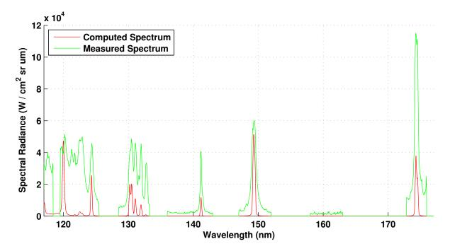
Figure 5.14: Computed and measured spectra across a  $90\,\mathrm{mm}$  cylindrical model at condition 2.
