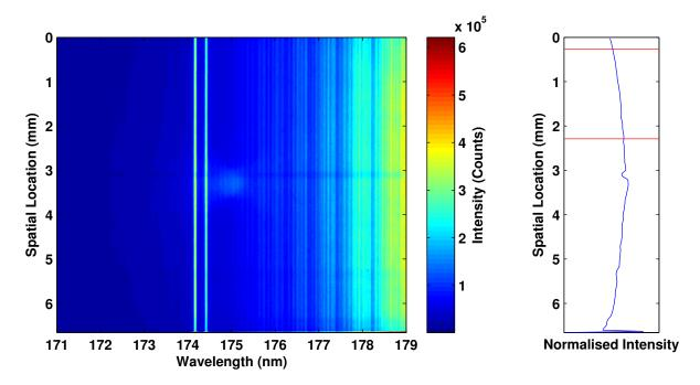
Figure 6.19: Uncalibrated, spatially resolved spectral image of plasma torch emission between 171 nm and 179 nm.
