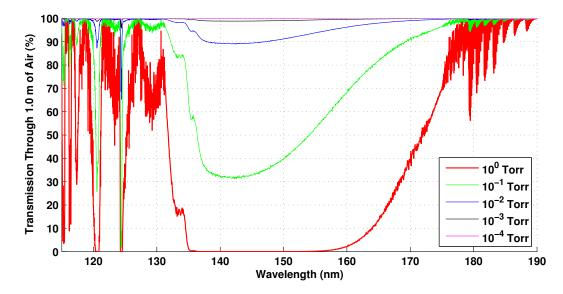
Figure 4.22: Transmission percentage of VUV radiation through  $1.0 \,\mathrm{m}$  of air at varying pressures.
