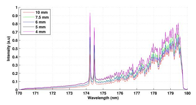
Figure 6.12: Plasma emission spectra obtained in the VUV with the water cooled window housing at 10 mm, 7.5 mm, 6 mm, 5 mm and 4 mm from the edge of the nozzle.
