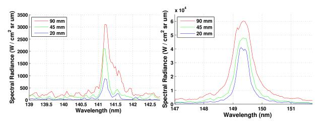
Figure 4.62: (Left) - Minimal peak broadening observed for condition 1 at the 141 nm line. (Right) - Strong peak broadening observed for the faster test condition on a self-absorbing line.
