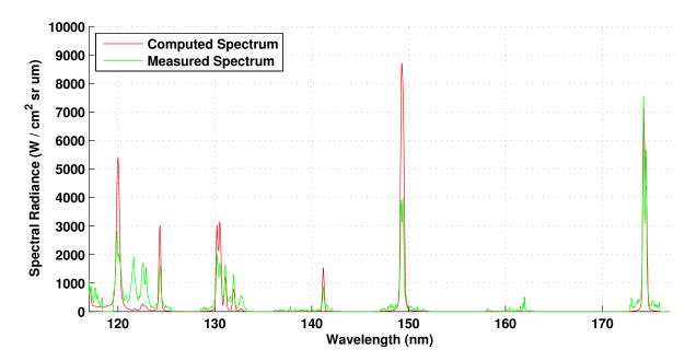
Figure 5.13: Computed and measured spectra across a  $20\,\mathrm{mm}$  cylindrical model at condition 1.
