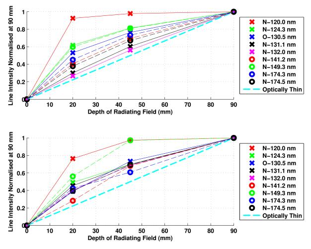
Figure 5.19: Spectral line intensities for condition 1 as a function of depth of radiating flow field, normalised at 90 mm depth of radiating flow field. (Top) - Computed results. (Bottom) - Experimental measurements.
