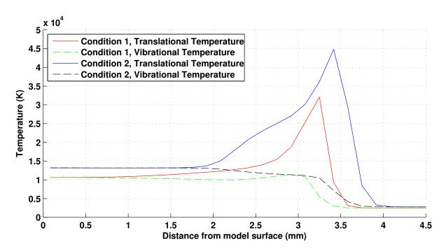
Figure 5.9: Computed stagnation streamline temperatures at both conditions.
