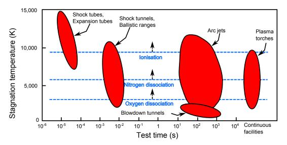
Figure 3.2: Stagnation temperature and test time ranges of various ground testing facilities. Adapted from Bertin [24].
