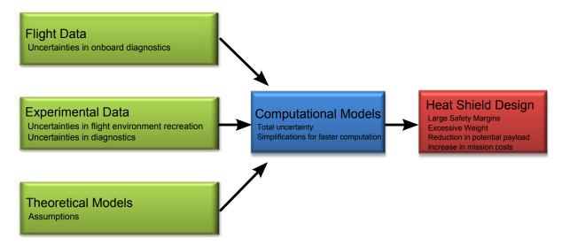
Figure 1.2: Design process of a spacecraft heat shield.
