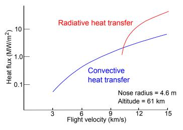
Figure 1.1: Variation of convective and radiative heat fluxes with increasing velocity. Radiative heat flux includes non-gray self-absorption and shock-layer radiative cooling. Adapted from Anderson [18].
