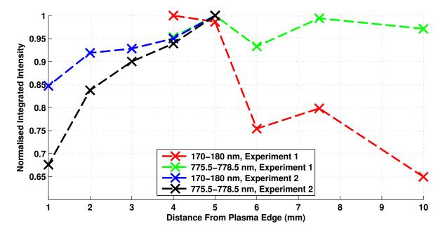
Figure 6.14: Integrated and normalised values of spectral measurements in the VUV between 170 nm and 180 nm and in the NIR between 775.5 nm and 778.5 nm for distances between 10 mm and 1 mm. Experiment 2 - Measurements between 1 mm and 4 mm. Experiment 1 - Measurements between 4 mm and 10 mm.
