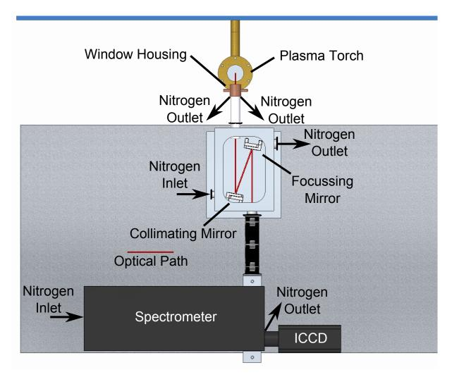
Figure 6.8: Optical configuration and nitrogen flow path for plasma torch experiments.
