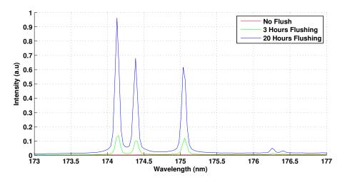
Figure 6.7: Increase in transmission through the optical path of the nitrogen and carbon lines between 173 nm and 177 nm after 0, 3 and 20 hours of flushing the spectrometer with nitrogen.
