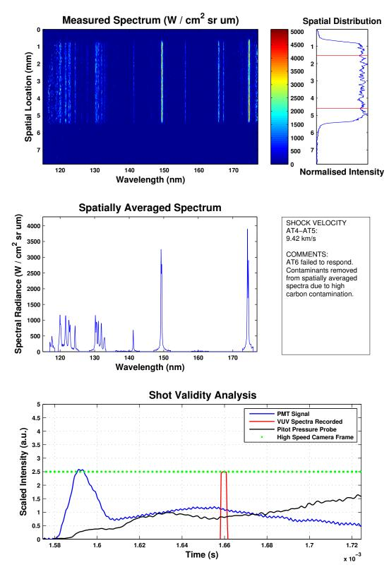
Figure D.3: x2s1954 - Primary shot data for through surface at condition 1.
