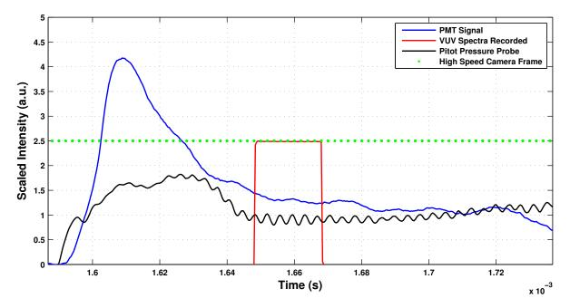
Figure 4.47: Shot validity graph showing ICCD exposure time in reference to the scaled intensity of the PMT data, the pitot pressure measured at the model and the points in time an image is recorded on the high speed camera.
