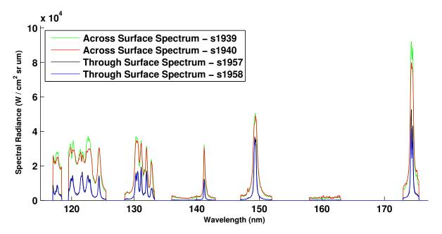
Figure 4.57: Comparison of across surface and through surface spectral measurements at condition 2.
