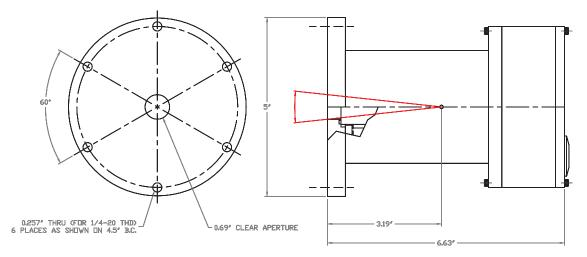
Figure 4.27: Calibration lamp internal dimensions
