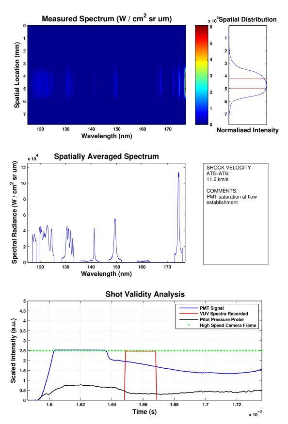
Figure D.16: x2s1930 - Repeat shot data for across the surface of a 90 mm model at condition 2.
