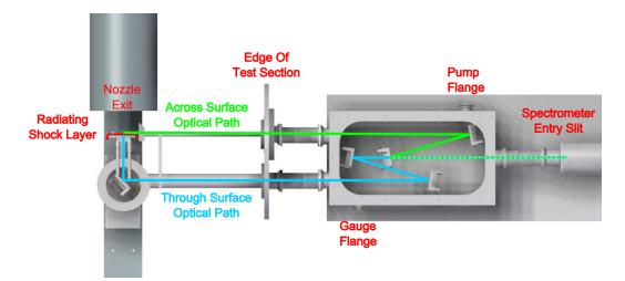
Figure 4.16: Imaging optics to observe radiation across and through the surface of the models. Image drawn to scale.
