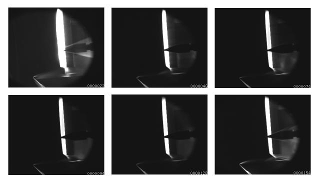
Figure 4.8: Steady flow for over 130  $\mu s$  achieved with a 10 mm gap. Counter in bottom right of each image is video time in  $\mu s$
