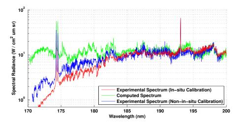
Figure 6.24: Comparison of measured spectra calibrated using an in-situ approach and a non-in-situ calibration and the spectrum computed by Specair.
