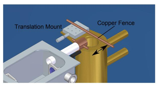
Figure 6.26: Concept of the traversable water cooled fence across the plasma to limit the depth of radiating flow field observed.
