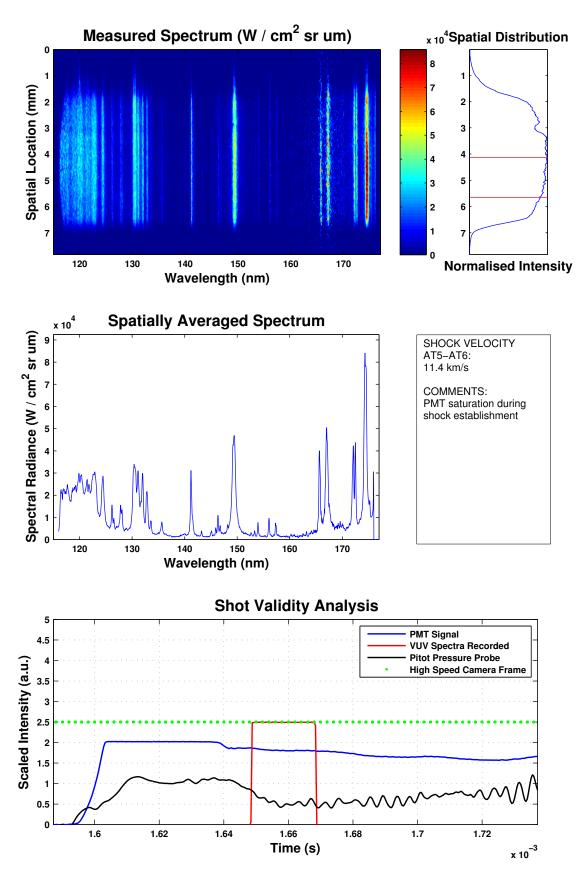
Figure D.6: x2s1939 - Repeat shot data for across the surface at condition 2.
