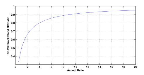
Figure 4.10: Shock stand off correction for varying aspect ratio square bodies in supersonic and hypersonic flow. An aspect ratio of 3.6 produces a 0.76 correction factor between two-dimensional and three-dimensional shock stand offs.
