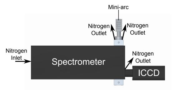
Figure 6.4: Initial nitrogen flush testing configuration with the mini-arc placed at the optical entrance of the spectrometer whilst nitrogen is flushed through it.
