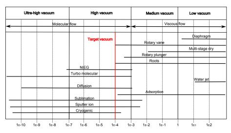
Figure 4.25: Array of vacuum pumping options available and their ranges. Source [28]
