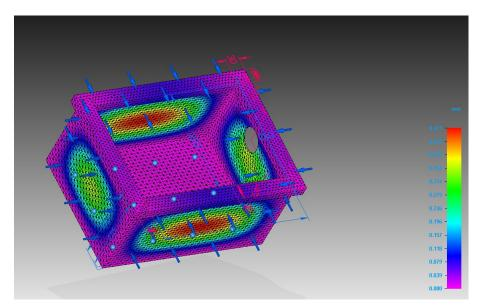
Figure 4.18: Deformation of the optical chamber with an atmospheric pressure force.
