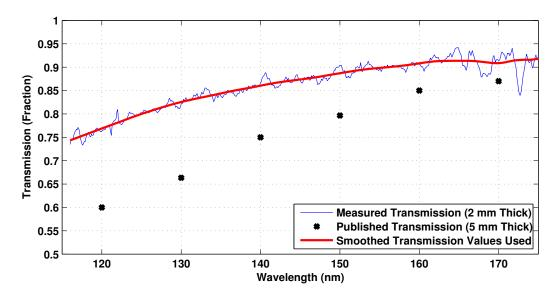
Figure 4.35: Measured and published transmissions of magnesium fluoride windows. Publish transmission from Crystran [29].
