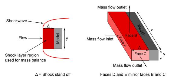
Figure 4.9: Left - Side on view of idealised two-dimensional shock stand off. Right - Three dimensional view of idealised region used for mass flow balance.
