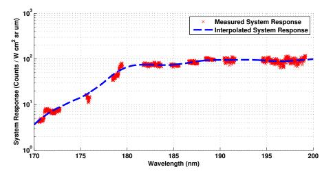
Figure 6.18: Spectral response of the system using in-situ calibration between 170 nm and 200 nm with interpolation across contaminant spectral lines.
