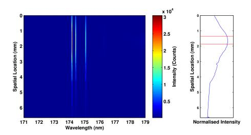
Figure 6.16: Spectral response of the system using in-situ calibration between 171 nm and 179 nm with interpolation across contaminant spectral lines.
