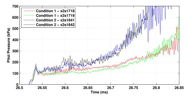
Figure 4.38: Experimental pitot traces for condition 1 and 2. Estimated test time for condition 1 is 26.55 ms to 26.70 ms and estimated test time for condition 2 is 26.55 ms to 26.65 ms.
