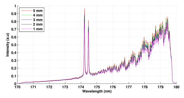
Figure 6.13: Plasma emission spectra obtained in the VUV with the window housing at 5 mm, 4 mm, 3 mm, 2 mm and 1 mm from the edge of the nozzle.
