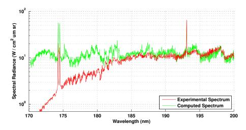
Figure 6.23: Comparison of the measured spectrum and the spectrum computed by Specair.
