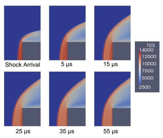
Figure 5.2: Time resolved images of shock arrival and flow establishment over the model.
