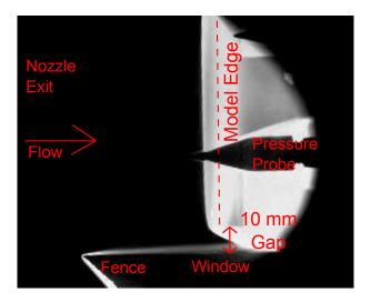
Figure 4.7: Top down view of second fence and window position with a  $10\,\mathrm{mm}$  gap to the blunt model.
