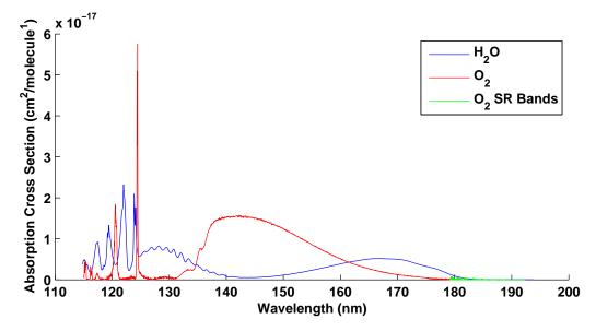
Figure 2.7: Absorption cross-sections for molecular oxygen [20],  $O_2$  Schumann-Runge bands [21] and water [22]
