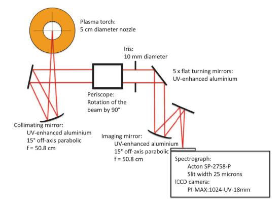
Figure 6.1: Optical system used to measure the atomic oxygen triplet at 777 nm [8].
