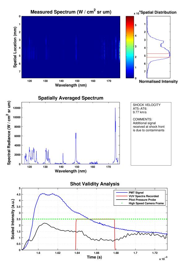
Figure D.12: x2s1933 - Repeat shot data for across the surface of a 45 mm model at condition 1.
