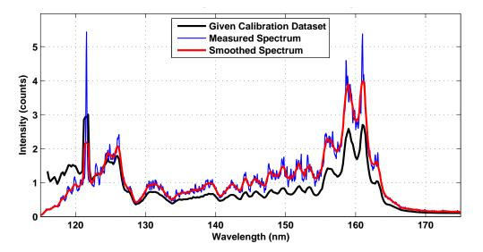
Figure 4.34: Spectral averaging or smoothing of measured data to achieve a spectral bandwidth matching that of the given calibration dataset.
