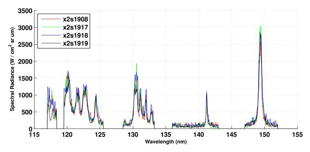
Figure 4.50: Results from repeatability study of condition 1 for the lower half of the VUV range.
