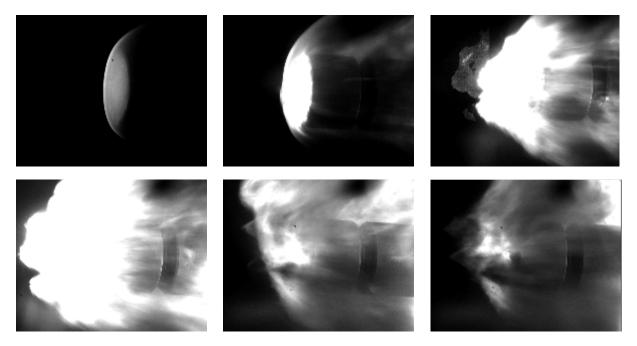
Figure 4.2: Mylar diaphragm fragments impacting on windows. The window during the steady test time can be seen in the top left image. Top right image shows the arrival of a large piece of Mylar diaphragm and its impact on the window.
