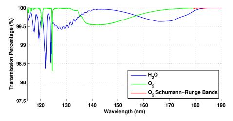
Figure 4.24: Results of a  $10^{-4}$  Torr vacuum pressure on the transmission of the VUV radiation through an optical path of 401.3 cm with a molecular oxygen mole fraction of 0.21 and a water vapour mole fraction of 0.5.
