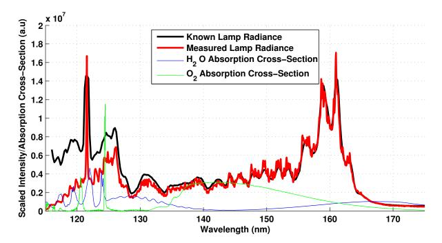
Figure 4.30: Scaled absorption cross-sections of water vapour and molecular oxygen superimposed on the measured and known spectral datasets.
