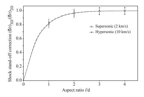
Figure 4.13: Shock stand off correction for varying aspect ratio cylinders in supersonic and hypersonic flow [27].
