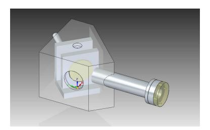
Figure 4.1: Proof of concept model with perspex front end and open mirror housing.
