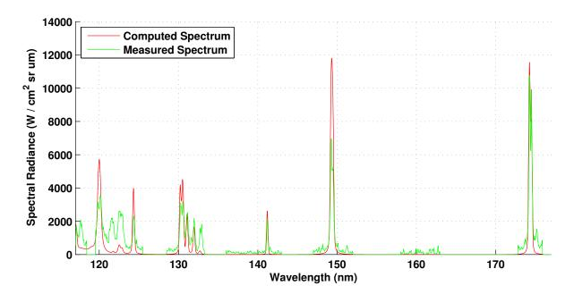
Figure 5.12: Computed and measured spectra across a 45 mm cylindrical model at condition 1.
