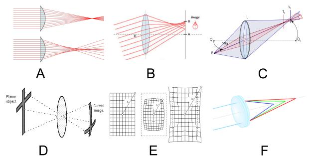
Figure A.1: Effects of A. spherical aberration, B. comatic, C. astigmatism, D. curvature of field, E. distortion and F. chromatic aberration
