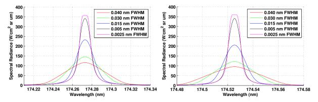
Figure 6.31: (Left) - Spectral line profile for various instrument broadening functions for the 174.27 nm atomic nitrogen spectral line. (Right) - spectral line profile for various instrument functions for the 174.53 nm atomic nitrogen spectral line. Both simulations conducted at atmospheric pressure at 6,700 K with a 4.5 cm depth of radiating flow field.
