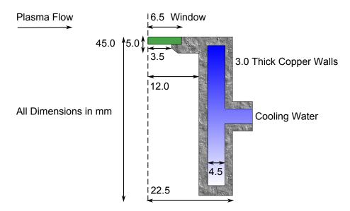
Figure 6.10: Final design of the water cooled window housing assembly.
