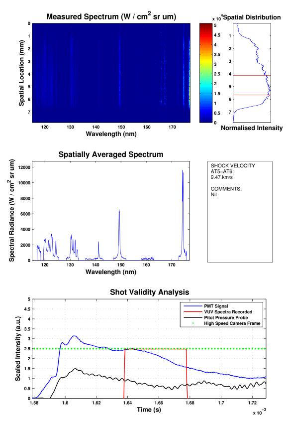
Figure D.2: x2s1936 - Repeat shot data for across the surface at condition 1.
