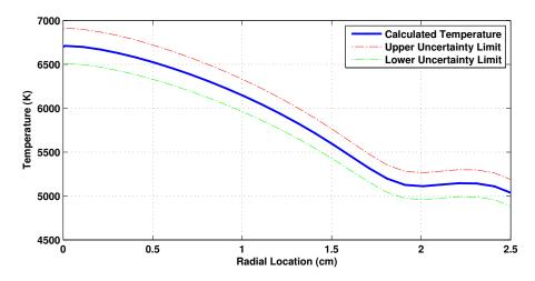
Figure 6.2: Measured temperature profile with upper and lower uncertainty limits.
