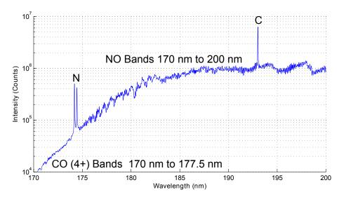
Figure 6.20: Uncalibrated spectrum of plasma emission from 170 nm to 200 nm.
