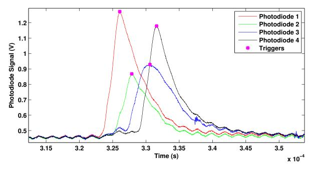
Figure 4.46: Signal traces from the photodiode array. Shock speed calculations between the three pairs of photodiodes produces 11.1 km/s, 7.3 km/s and 20.0 km/s. A curve of best fit predicts 10.1 km/s.
