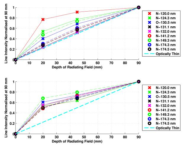
Figure 5.20: Spectral line intensities for condition 2 as a function of depth of radiating flow field, normalised at 90 mm depth of radiating flow field. (Top) - Computed results. (Bottom) - Experimental measurements.
