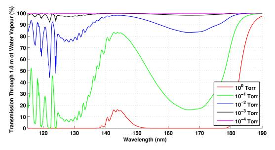
Figure 4.23: Transmission percentage of VUV radiation through 1.0 m of water vapour at varying pressures.
