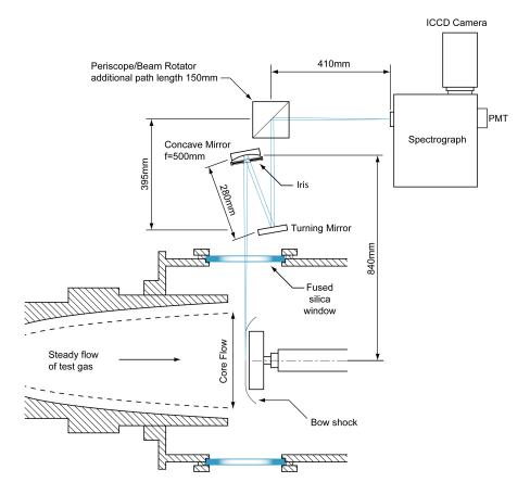
Figure 4.42: Optical system used with VNIR and UV spectroscopy system now used with a PMT. Adapted from [32]
