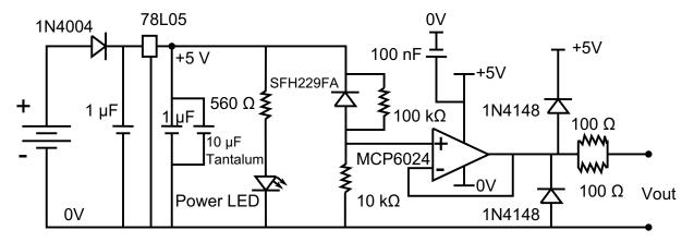
Figure 4.45: schematic of the amplifier and terminator circuit designed for each photodiode. Adapted from Zander [34]
