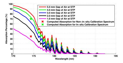
Figure 6.25: Radiation absorption of a slab of air at ambient temperature and atmospheric pressure with a molecular oxygen mole fraction of 0.21 at over various path lengths. The level of absorption predicted by the comparison of Specair simulation and the measured values using the two calibration approaches at a distance of 5 mm from the plasma edge are also presented.
