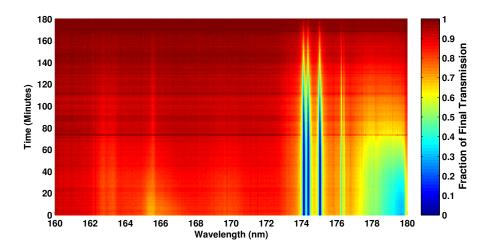
Figure 6.6: Increase in radiation transmission between 170 nm and 180 nm during 180 minutes of flushing the spectrometer with nitrogen.
