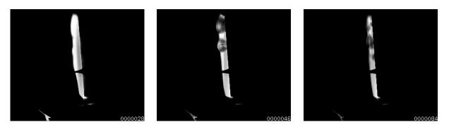
Figure 4.11: Top down view of vaporised aluminium impacting the surface. Flow from left to right.
