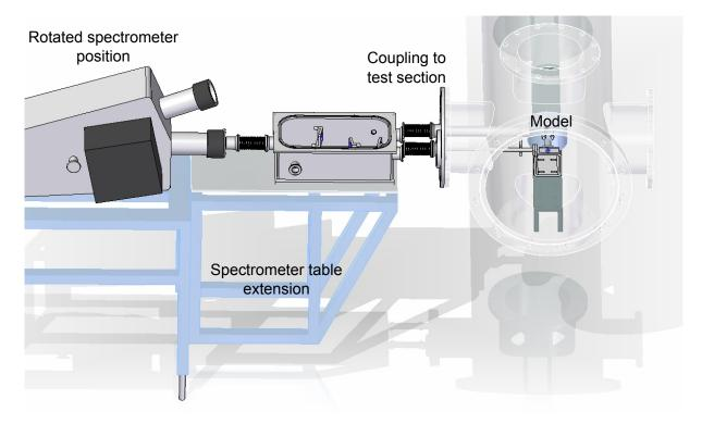
Figure 4.17: Extension of spectrometer table and rotation of spectrometer for enhanced compatibility with test section.
