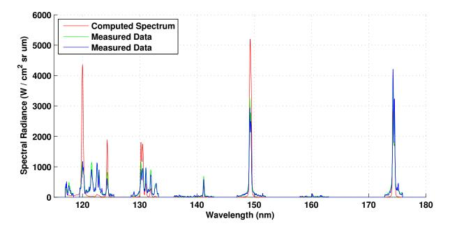
Figure 5.6: Computed and experimentally measured through surface spectra for condition 1.
