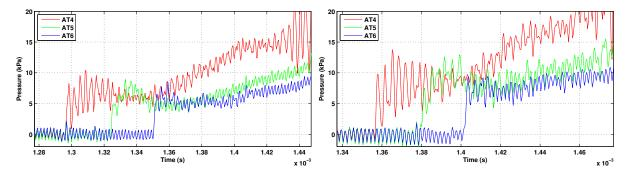
Figure 4.40: Measured static pressure values at the downstream end of the acceleration tube for condition 1 (Left) and condition 2 (Right).
