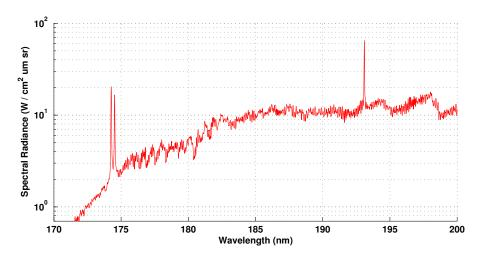
Figure 6.21: Calibrated and spatially averaged spectrum of plasma emission from  $170\,\mathrm{nm}$  to  $200\,\mathrm{nm}.$
