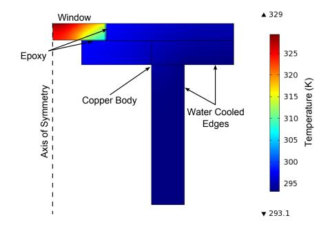
Figure 6.11: Results of the COMSOL Multiphysics simulation showing the steady state temperature of the window within the water cooled copper housing.
