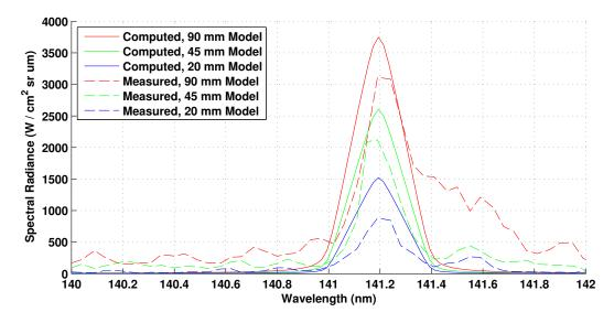
Figure 5.21: Experimentally measured and computed spectral line widths for the 141.2 nm peak at condition 1.
