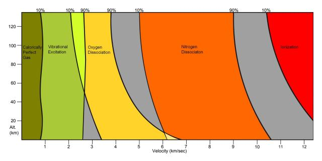
Figure 2.3: Effects of shock heating in air at varying velocities and altitudes. Adapted from Anderson [18]
