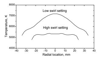
Figure 3.6: Representative temperature profiles for a high swirl and low swirl condition. Adapted from Laux [105].
