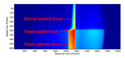
Figure 4.21: Blurred spectral focus at spatial focal point and sharp spectral focus at slit location.
