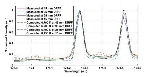
Figure 6.30: Measured and computed normalised spectral lines of the 174.3 nm and 174.5 nm nitrogen doublet at varying depths of radiating flow field.
