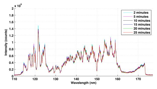
Figure 4.31: Spectra of the deuterium lamp during start up
