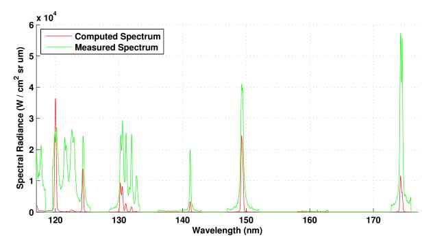
Figure 5.16: Computed and measured spectra across a 20 mm cylindrical model at condition 2.
