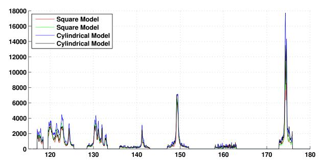
Figure 4.60: Comparison of VUV emission measured across a 90 mm square and cylindrical model for condition 1.
