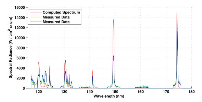
Figure 5.5: Computed and experimentally measured across surface spectra for condition 1.
