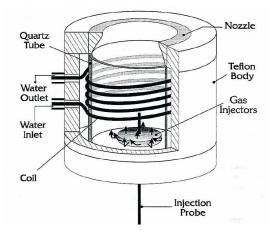
Figure 3.4: Schematic of the plasma torch [25]
