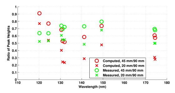
Figure 5.18: Experimentally measured and computed spectral line peak height ratios for condition 2.
