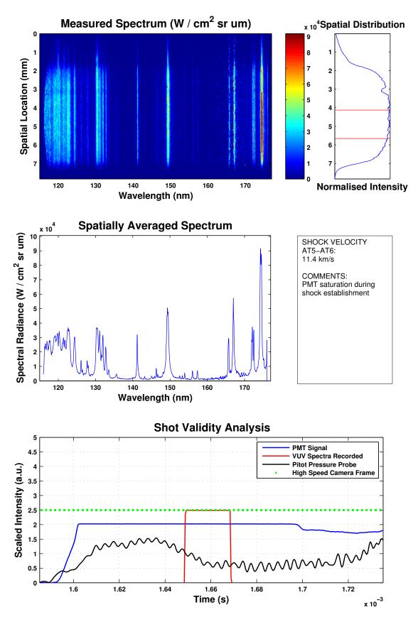
Figure D.5: x2s1940 - Primary shot data for across the surface at condition 2.
