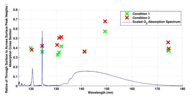
Figure 4.58: Ratios of the selected peak heights when observing through the surface compared to across the surface. Molecular oxygen absorption spectrum superimposed to investigate boundary layer oxygen absorption.
