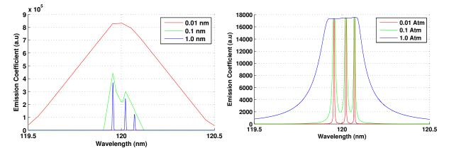
Figure 2.6: Broadening effects on an atomic oxygen triplet calculated using Specair. (Left) - Effect of varying the instrument function on observed spectral lines at 10,000 K using STP air with a 1 cm depth of radiating flow field. (Right) - Effect of broadening at varying pressures of pure nitrogen. Calculated at 7,000 K and 1 cm depth of radiating flow field with no instrument function convolution.
