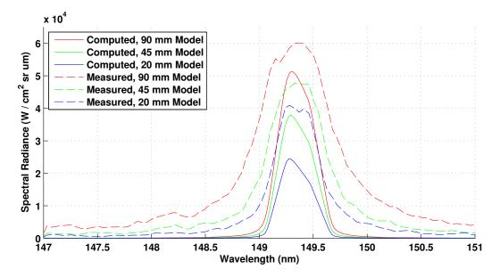
Figure 5.22: Experimentally measured and computed spectral line widths for the 149.3 nm peak at condition 2.
