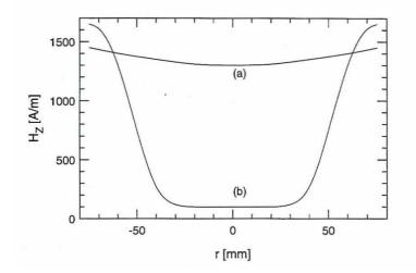
Figure 3.5: Intensity of the magnetic field without a discharge (a) and with a discharge (b). [25]
