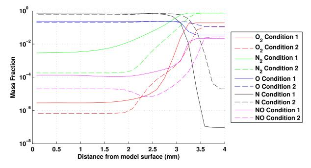
Figure 5.10: Computed stagnation streamline mass fractions using the Park reaction scheme at both conditions.
