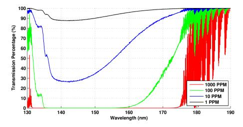
Figure 6.3: Influence of molecular oxygen contaminants on transmitted signal through an optical path of 3 m.
