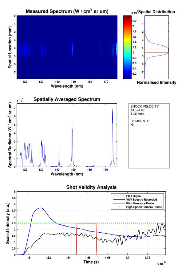
Figure D.19: x2s1944 - Repeat shot data for across the surface of a 20 mm model at condition 2.
