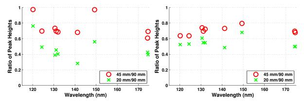
Figure 4.59: (Left) - Ratios of spectral line peaks for condition 1. (Right) - Ratios of spectral line peaks for condition 2. Nitrogen lines selected are 120.0 nm, 124.3 nm, 131.1 nm, 132.0 nm, 141.2 nm, 149.3 nm, 174.3 nm and 174.5 nm. Oxygen line at 130.5 nm.
