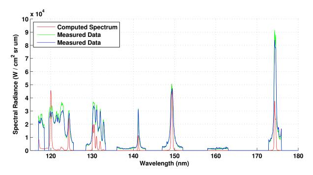
Figure 5.7: Computed and experimentally measured across surface spectra for condition 2.
