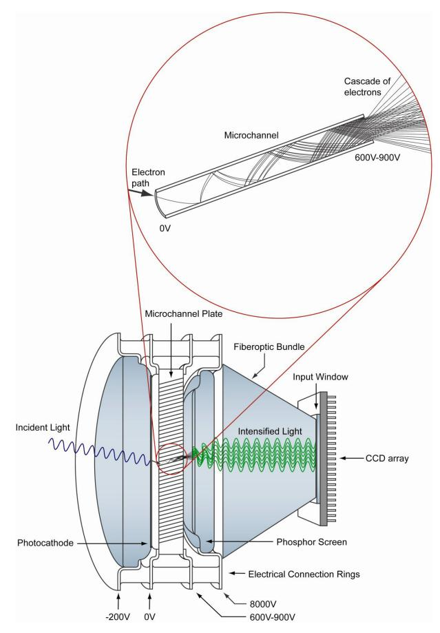
Figure B.1: Cross section of a Princeton Instruments Generation II Image Intensifier and CCD array. [35]
