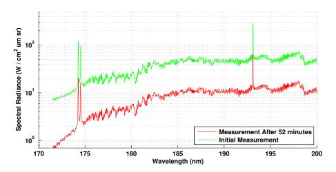
Figure 6.22: Calibrated and spatially averaged spectra at torch start up and after 52 minutes of operation.
