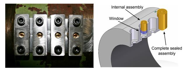
Figure 4.44: Top down view of installed photodiode mount assembly (left). Schematic of photodiode mounts assembly (right).
