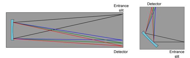
Figure 4.15: Left - Normal incidence concave grating Seya-Namioka monochromator. Right - Turning concave grating design.
