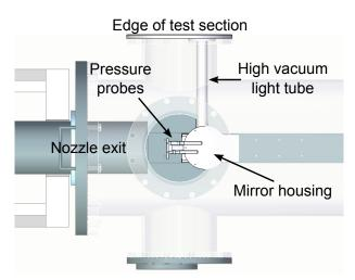
Figure 4.3: Top down view of high vacuum path to model with mirror housing assembly and pressure probes.
