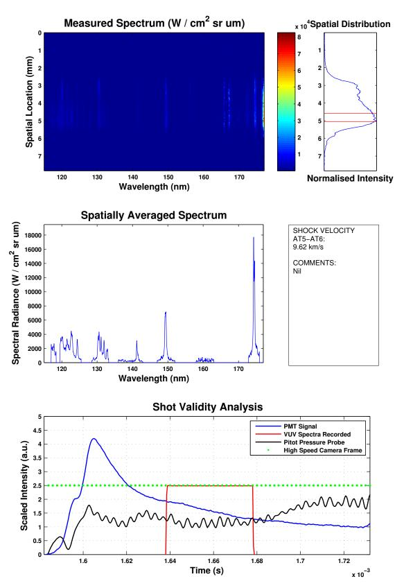
Figure D.9: x2s1926 - Primary shot data for across the surface of a 90 mm model at condition 1.
