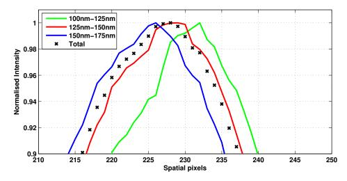
Figure 4.32: Spatial variation in the location of peak radiation output due to a twisting angle between the grating and the camera
