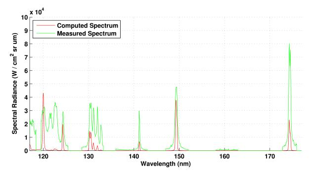
Figure 5.15: Computed and measured spectra across a 45 mm cylindrical model at condition 2.
