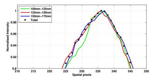
Figure 4.33: Results of a 0.375 degree rotation of the recorded image on the position of the peak spectral radiation output.
