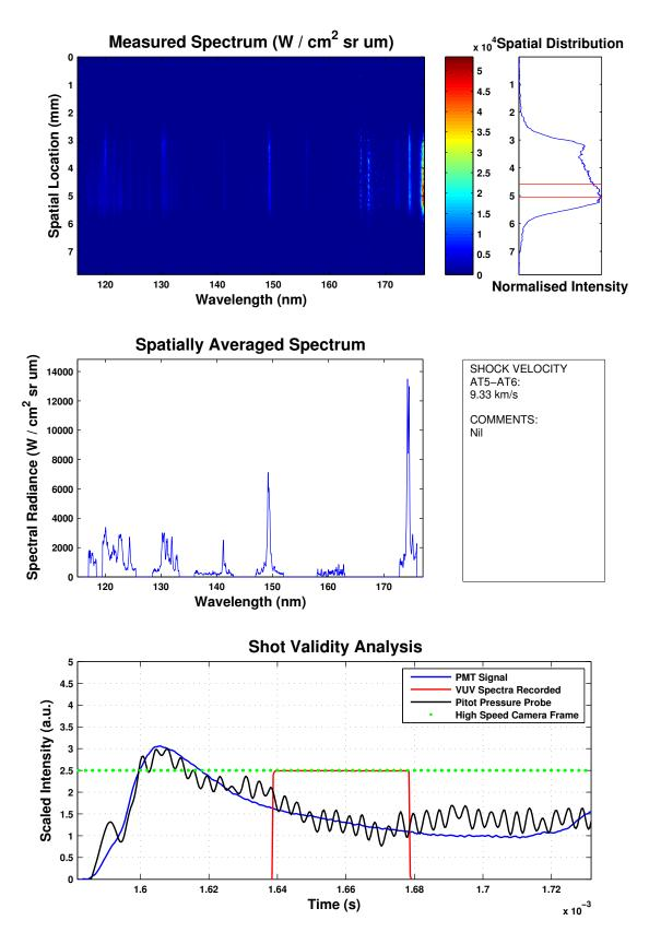
Figure D.10: x2s1927 - Repeat shot data for across the surface of a 90 mm model at condition 1.
