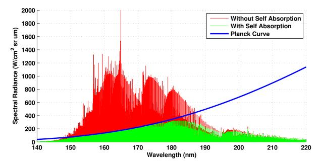
Figure 2.5: Planck's law limiting radiative emission and causing self-absorption to occur. Simulation conducted using Specair for CO(4+) at a temperature of 6,600 K, pressure of 2,000 Pa and 1.0 cm depth of radiating flow field.
