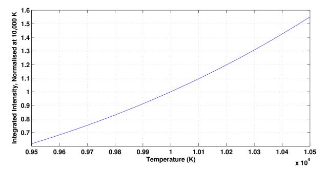
Figure 4.52: Integrated values of the Planck curve between 120 nm and 180 nm at various temperatures, normalised at 10,000 K.
