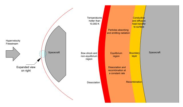
Figure 2.4: Depiction of the varying regions possible within a shock layer. Adapted from [18]
