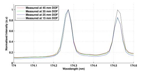
Figure 6.29: Normalised spectral lines of the 174.3 nm and 174.5 nm nitrogen doublet at varying depths of radiating flow field.
