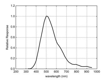
Figure 4.43: Spectral response of the Shimadzu HPV-1 high speed camera [33]
