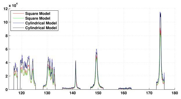
Figure 4.61: Comparison of VUV emission measured across a 90 mm square and cylindrical model for condition 1.
