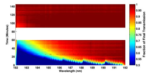
Figure 6.5: Increase in transmission through the optical path during 145 minutes of flushing the spectrometer with nitrogen. Spectra were not recorded in this wavelength range between 60 and 90 minutes.
