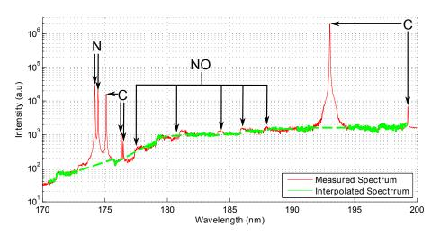
Figure 6.17: Spectral data obtained using the mini-arc with nitrogen and carbon contamination lines.
