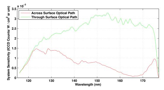
Figure 4.36: Final system sensitivity measured for both optical systems. The across system sensitivity here is calculated for a 10.0 mm aperture.
