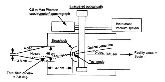
Figure 3.7: Schematic arrangement of the Palumbo arc jet experiment [26]
