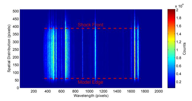
Figure 4.54: Raw image acquired on the ICCD across at flat 90 mm model at condition 2.
