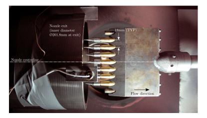
Figure 4.37: Pitot rake arrangement with conical glancing pressure probes for conditions testing. [30]
