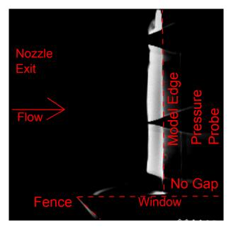
Figure 4.5: Top down view of initial fence and window position with no gap to the blunt model.
