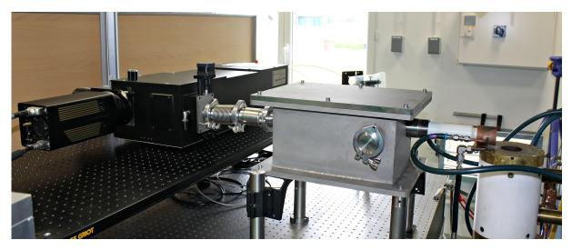
Figure 6.9: Final set up of the spectrometer, optical chamber, water cooled window housing and the plasma torch.
