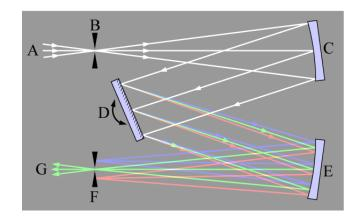
Figure 4.14: Depiction of a Czerny-Turner configuration. Light (A) is focused onto an entrance slit (B) and is collimated by a curved mirror (C). The collimated beam is diffracted from a rotatable grating (D) and the dispersed beam re-focussed by a second mirror (E) at the exit slit (F). Each wavelength of light is focussed to a different position at the slit, and the wavelength which is transmitted through the slit (G) depends on the rotation angle of the grating. [134]
