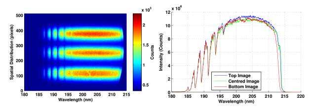
Figure 4.29: Left - Superimposed calibration images depicting ICCD array ranges tested. Right - Results of integrating each image indicate there negligible variation in pixel sensitivity across the ICCD. The slight discrepancy at the longer wavelength cut off is due to the circular shape of the intensifier clipping the signal.
