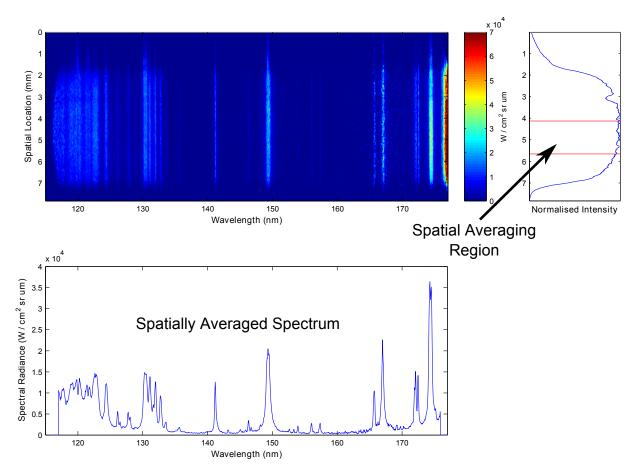
Figure 4.55: (Top Left) - Calibrated image across a 90 mm model at condition 2. (Top Right) - Spatial distribution of recorded emission and spatial region averaged across. (Bottom) - Spatially averaged spectrum produced.
