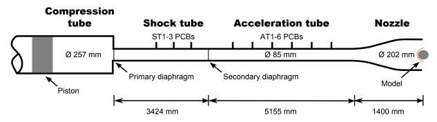
Figure 3.3: Schematic of the X2 expansion tube configuration used for this study. ST1-3 and AT1-6 PCBs are the shock tube and acceleration tube pressure transducers.
