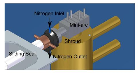
Figure 6.15: Schematic of the in-situ calibration approach with a shroud to contain the nitrogen flush used to remove molecular oxygen between the viewing window and the mini-arc.
