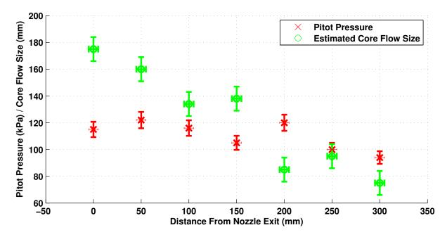
Figure 4.39: Measured core flow size and variation in pitot pressure at distances from the nozzle exit for condition 1
