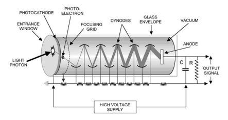
Figure 4.41: Schematic of a photomultiplier tube. [31]
