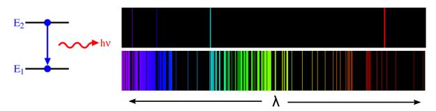
Figure 2.2: (Left) - Photon emission in the visible wavelength range through spontaneous transition to a lower energy state. (Right) - Spectral lines possible as a result of quantum transitions. Hydrogen spectrum (top) with minimal lines due to a small number of possible transitions and iron (bottom) with many different quantum transitions possible resulting in numerous spectral lines. Adapted from [40]
