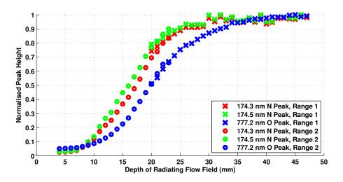
Figure 6.28: Spectral line peak intensities at various depths of radiating flow fields normalised using the measured intensities at a 50 mm depth of radiating flow field. Spectral lines compared are the 174.3 nm and 174.5 nm atomic nitrogen lines and the 777.2 nm atomic oxygen line.
