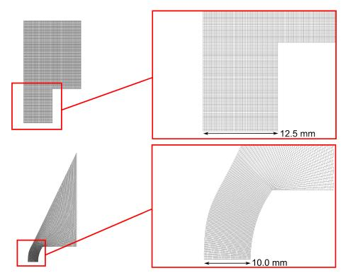
Figure 5.1: Structured grids used in the simulation of both models.
