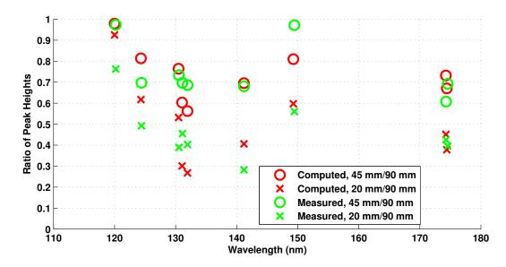
Figure 5.17: Experimentally measured and computed spectral line peak height ratios for condition 1.
