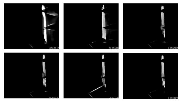
Figure 4.6: Perturbations created by the fence and stagnation region between the fence and the model.
