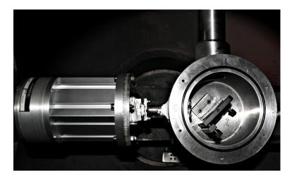
Figure 4.26: Calibration lamp mounted in place of the model.
