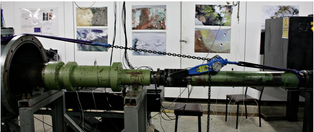
Figure 4.20: A chain block was used to move the test section into firing position. This was required to account for movement of the test section due to vacuum forces.
