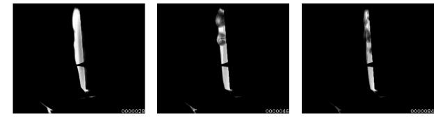
Figure 4.11: Top down view of vaporised aluminium impacting the surface. Flow from left to right.
