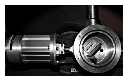
Figure 4.26: Calibration lamp mounted in place of the model.
