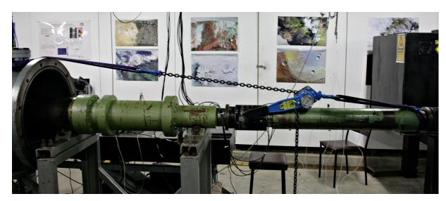
Figure 4.20: A chain block was used to move the test section into firing position. This was required to account for movement of the test section due to vacuum forces.
