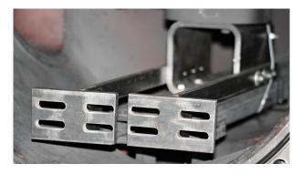
Figure 4.4: Additional bracing installed to ensure model position is maintained.
