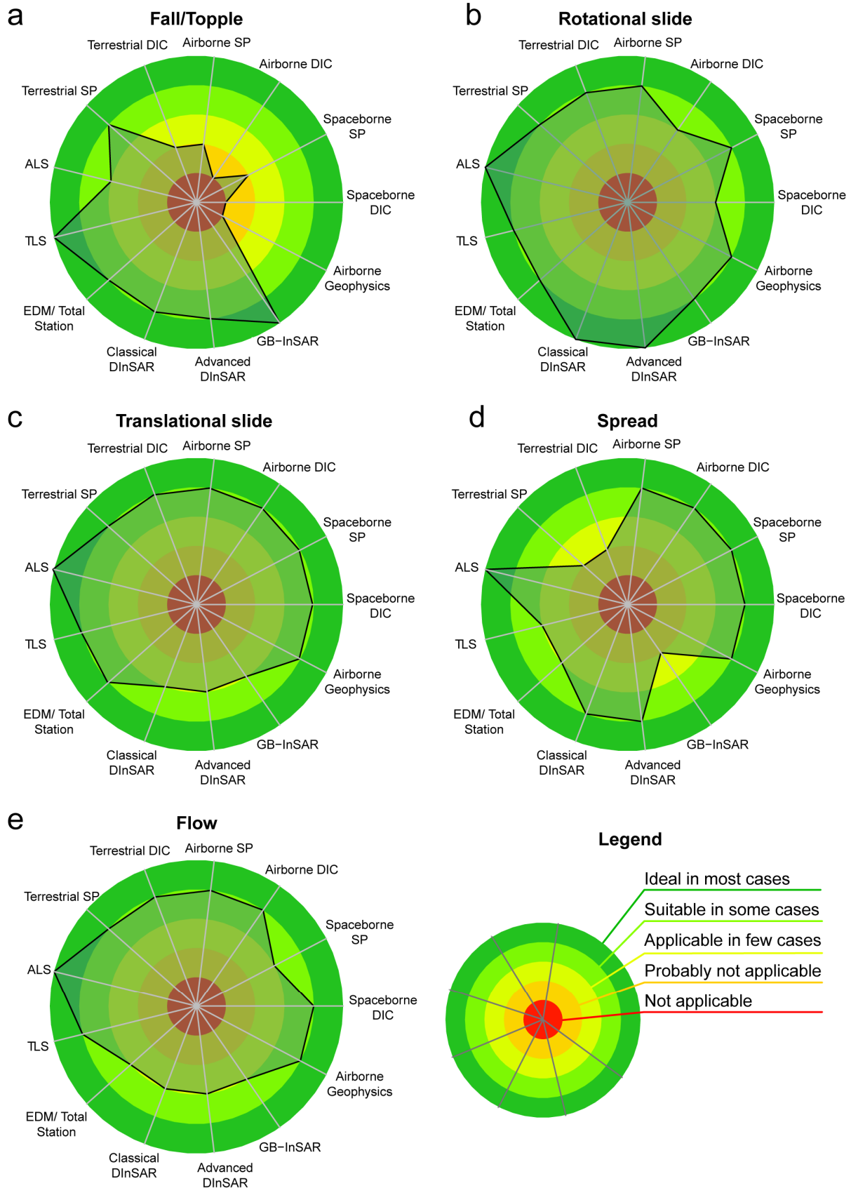
Figure 1-5: Suitability of remote sensing techniques for the monitoring of different landslide types including (a) falls and topples, (b) rotational slides, (c) translational slides, (d) spreads and (e) flows.
