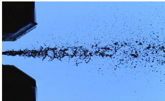
Figure 1.2: Experimental view of a direct liquid injection with various two-phase flow topologies [49].
