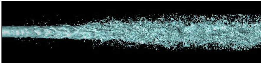
Figure 1.3: DNS simulation of a liquid jet atomization through the hybrid VOF/Level Set sharp interface approach [126].
