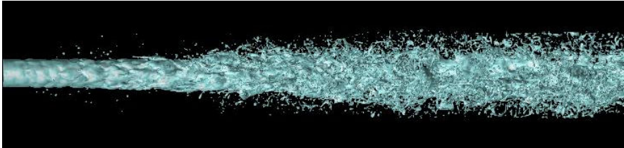
Figure 1.3: DNS simulation of a liquid jet atomization through the hybrid VOF/Level Set sharp interface approach [126].
