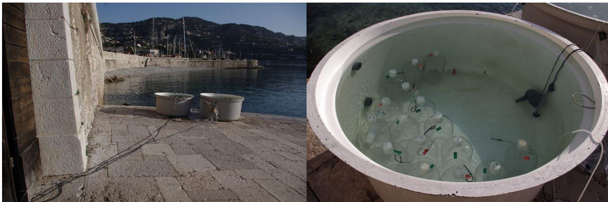
Supplementary Material: Figure SM-IV-1. Picture of the experiment showing the two outdoor tanks on the pontoon in Villefranche-sur Mer (left) and the + 3°C with the 4 L bottles, the heater and pump for water circulation (right).
