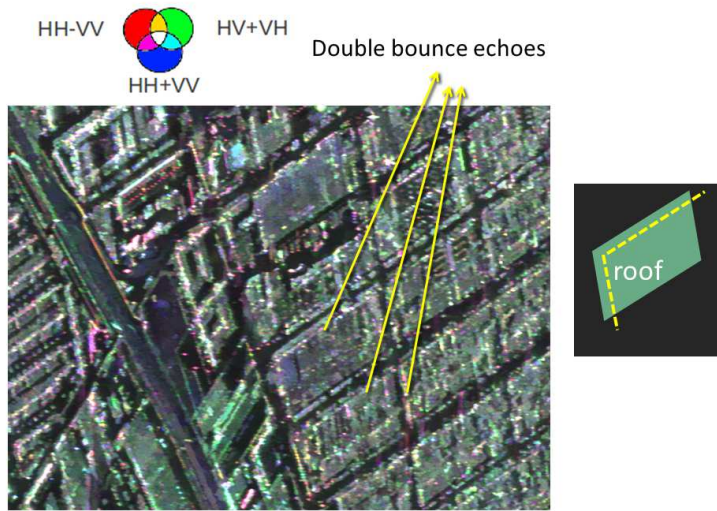
Figure 46: Double bounce echoes visible on UAVSAR polarimetric images
