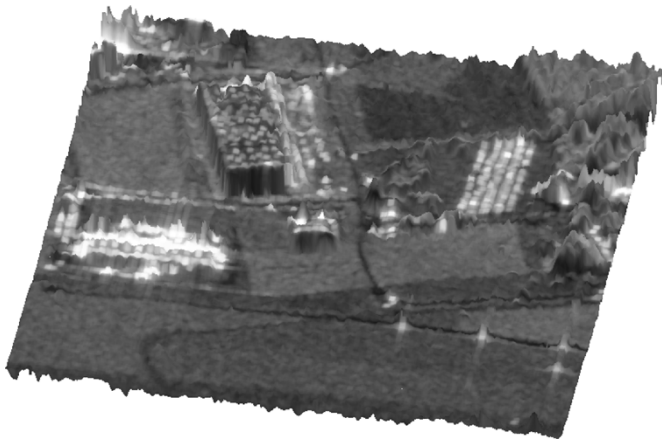
Fig. 8. Digital elevation model after 1MC coherence optimization.
