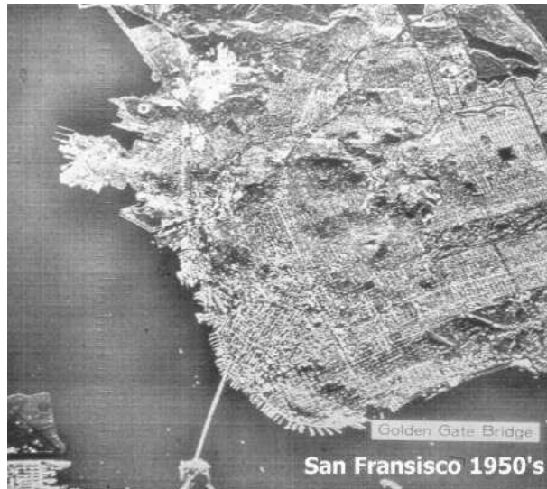
Figure 4: A first Real Aperture Radar image acquired by a Side Looking Airborne System developed by Westinghouse, under sponsorship from the United States Air Force in 1954
