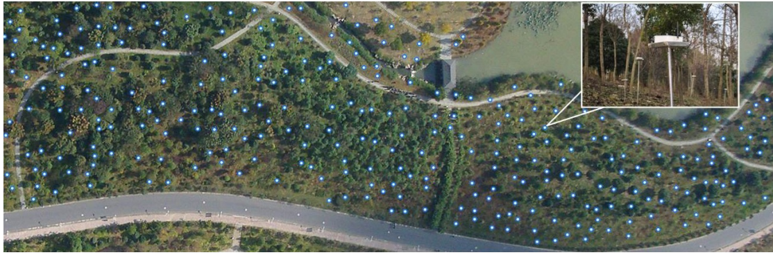
FIGURE 1.1: The GreenOrbs sensor network for ecological surveillance in the forest, collecting data such as temperature, humidity, illumination, and carbon dioxide titer.
