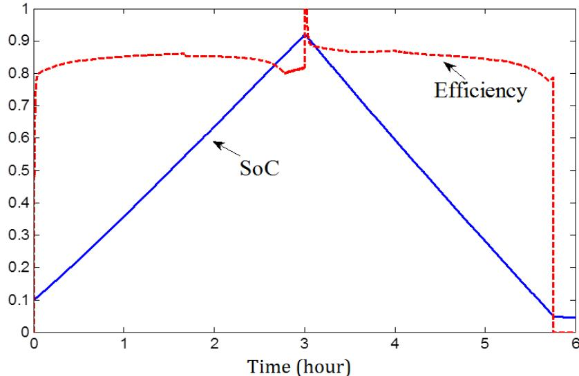
Fig. III.6. SoC and efficiency variation during a charge-discharge cycle.
