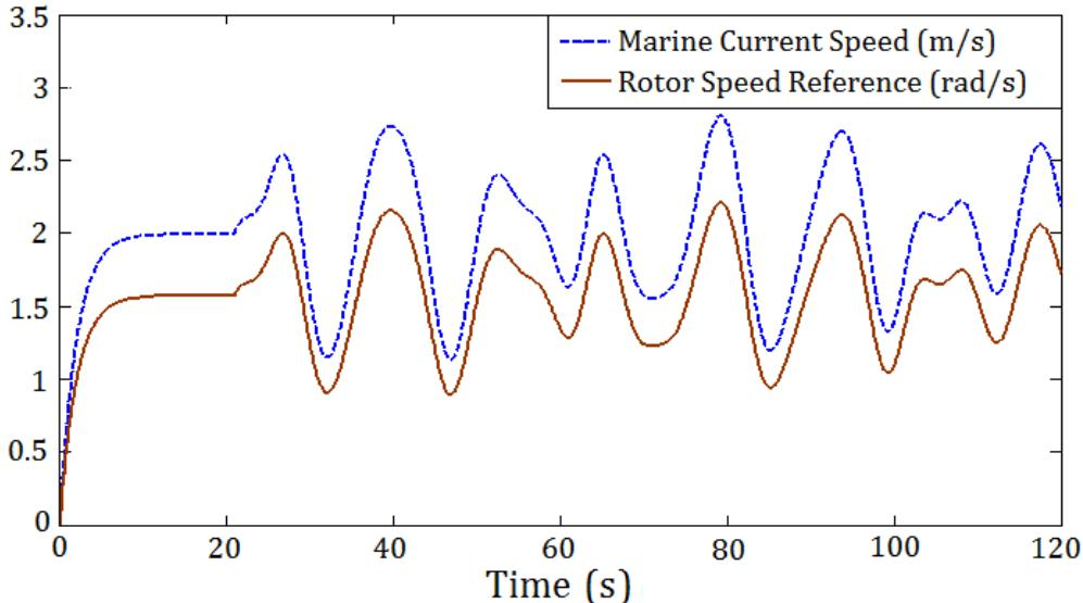
Fig. II.15. Rotor speed reference calculated by conventional MPPT.
