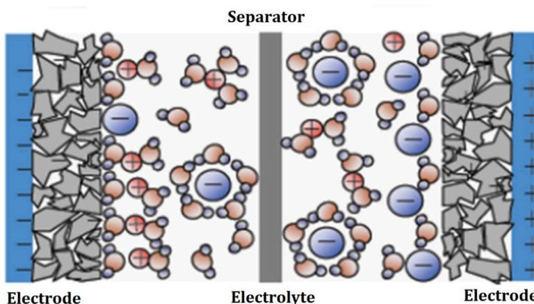
Fig. I.13. Supercapacitor cell [44].
