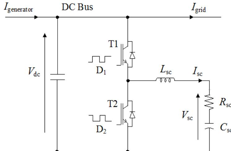
Fig. II.26. Supercapacitor and the bi-directional DC/DC converter.
