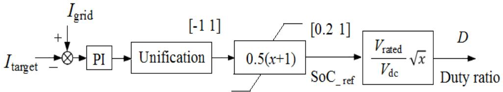
Fig. II.28. Control scheme of the bi-directional DC/DC converter.
