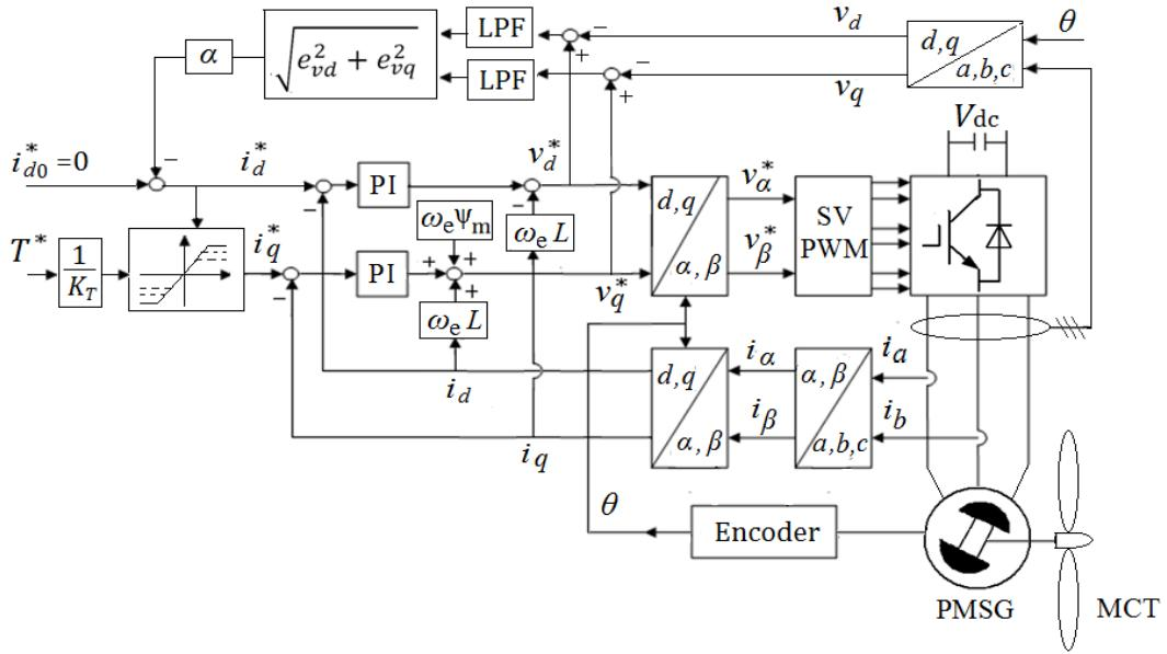
Fig. IV.5. Generator-side control scheme with flux-weakening strategy.
