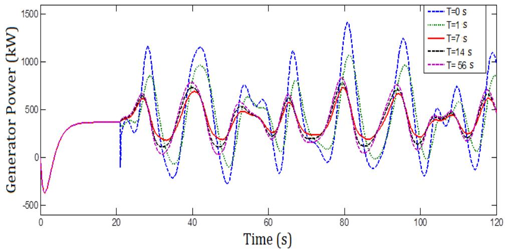
Fig. II.17. Generator powers with different filter time constants.
