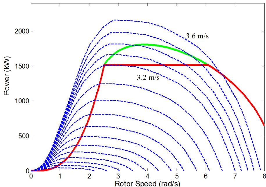
Fig. IV.28. Generator power characteristics with flatter  $C_p$ .
