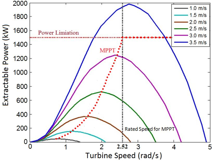
Fig. IV.2. The turbine power characteristics (§ II.3).
