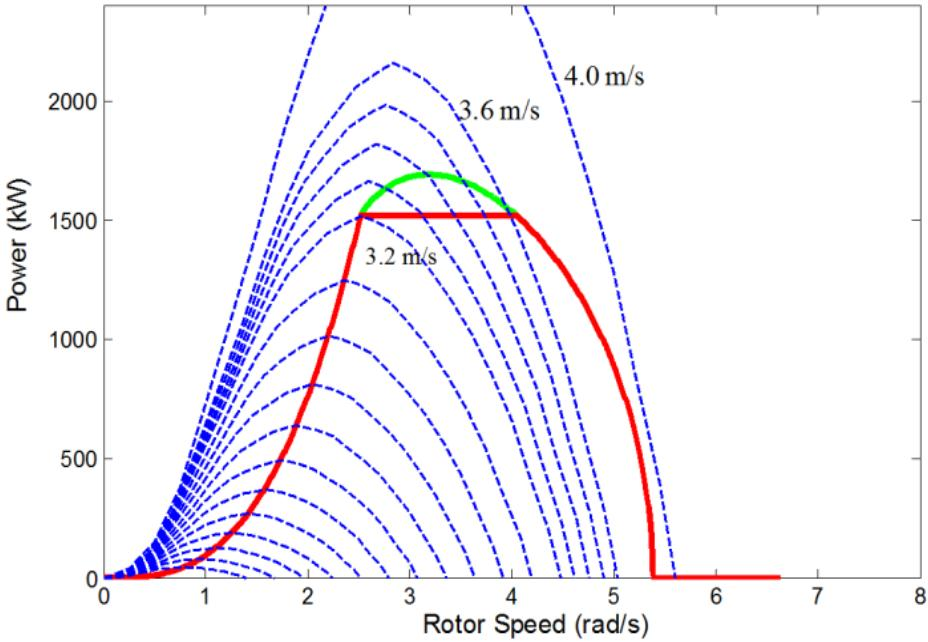
Fig. IV.26. Generator power characteristics with CPSR = 1.6.
