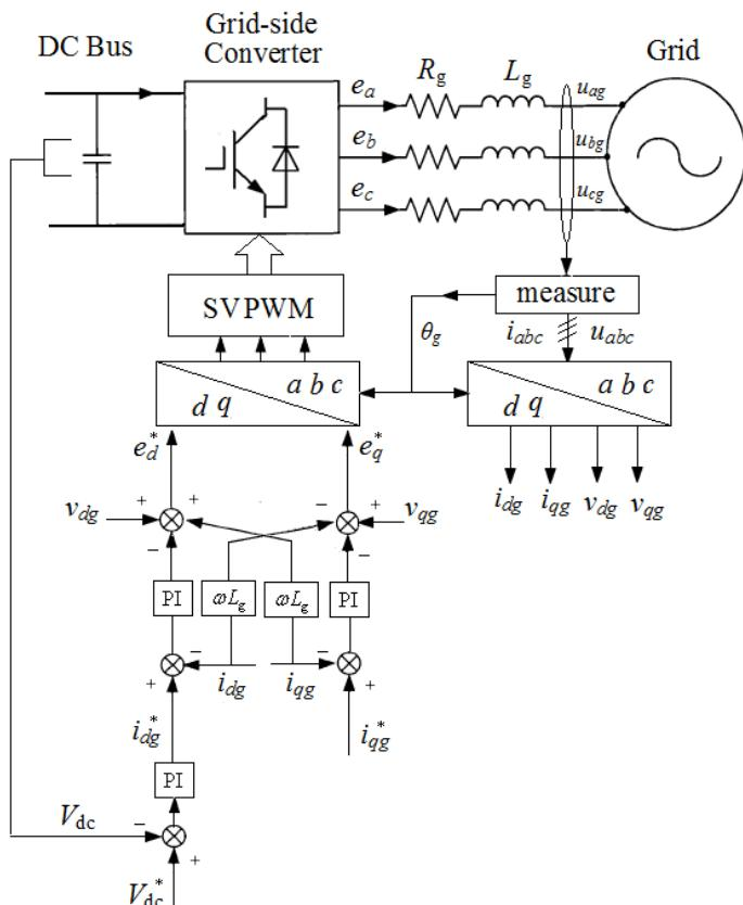
Fig. II.23. Control scheme of the grid-side converter.
