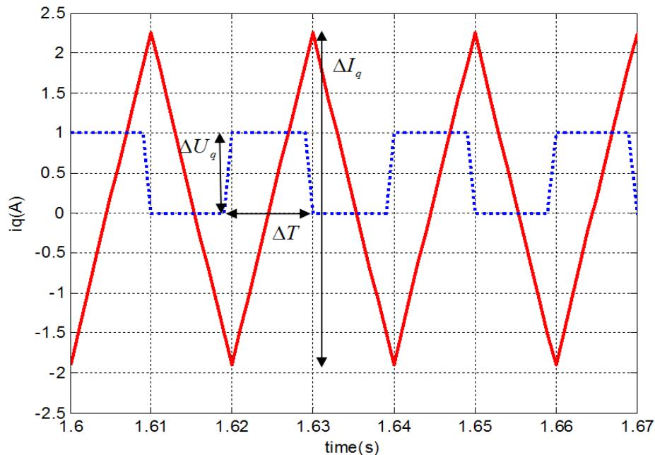
Fig. II.13. Open-loop generator current response in  $q$ -axis.
