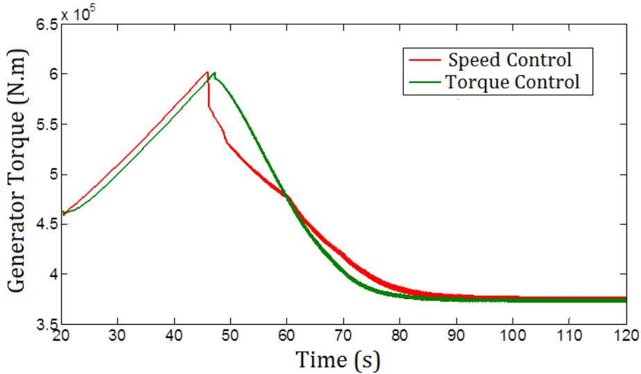
Fig. IV.9. Generator torque responses at high tidal speed.
