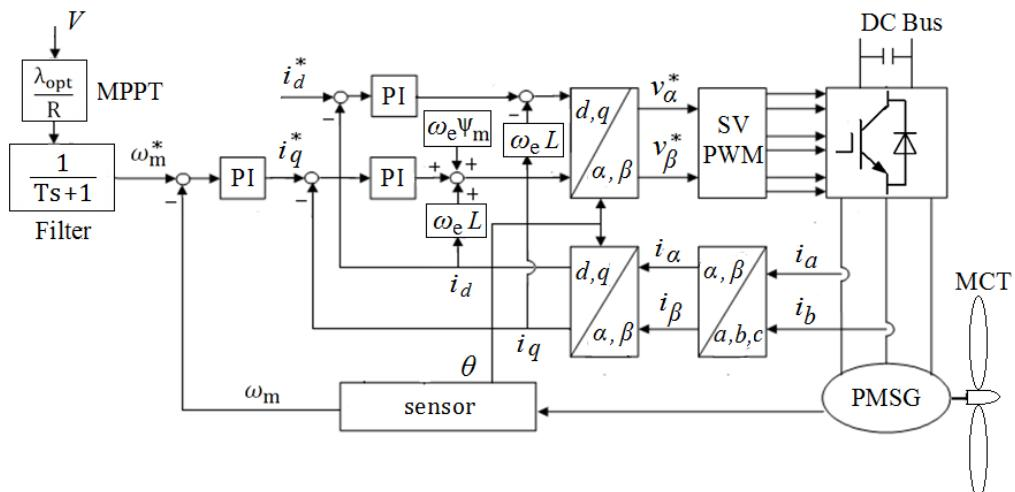
Fig. II.12. Control scheme of the generator-side converter.
