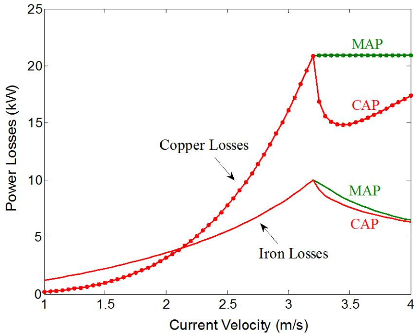
Fig. IV.20. Generator losses under different current velocities.
