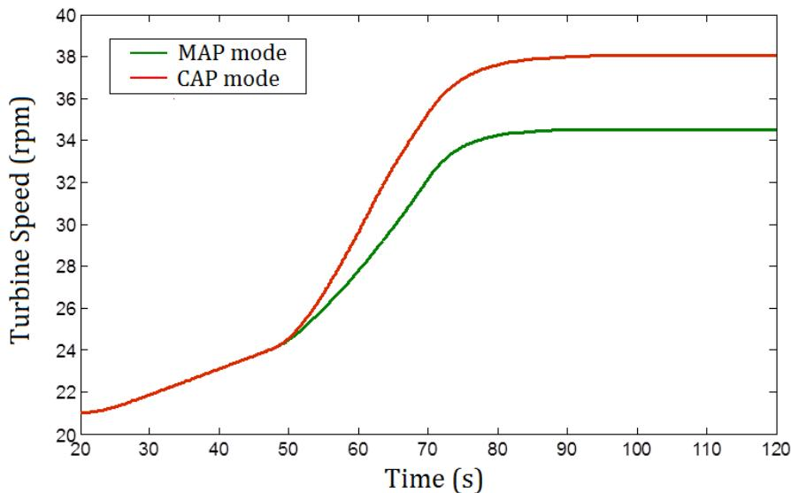
Fig. IV.15. Rotor speed responses at high tidal speed.
