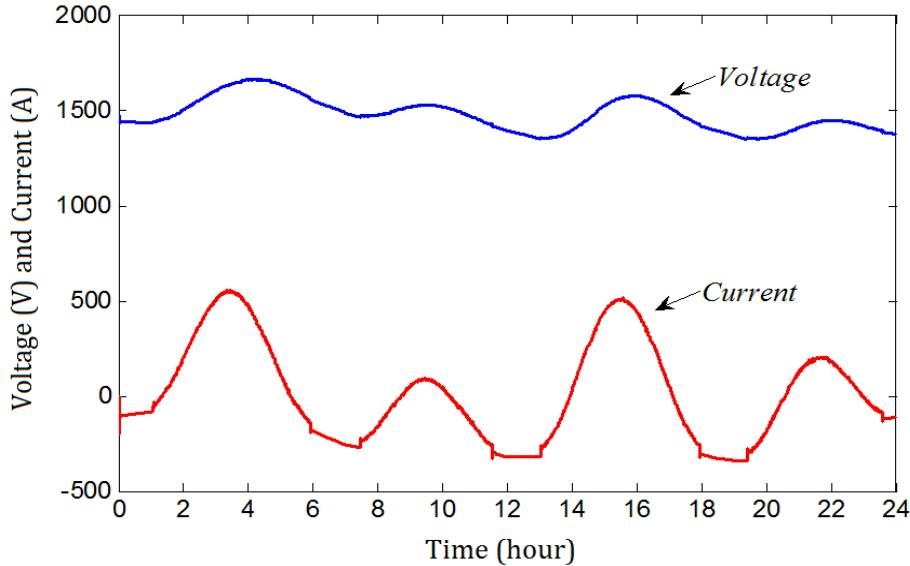
Fig. III.9. Voltage and current of the BESS.
