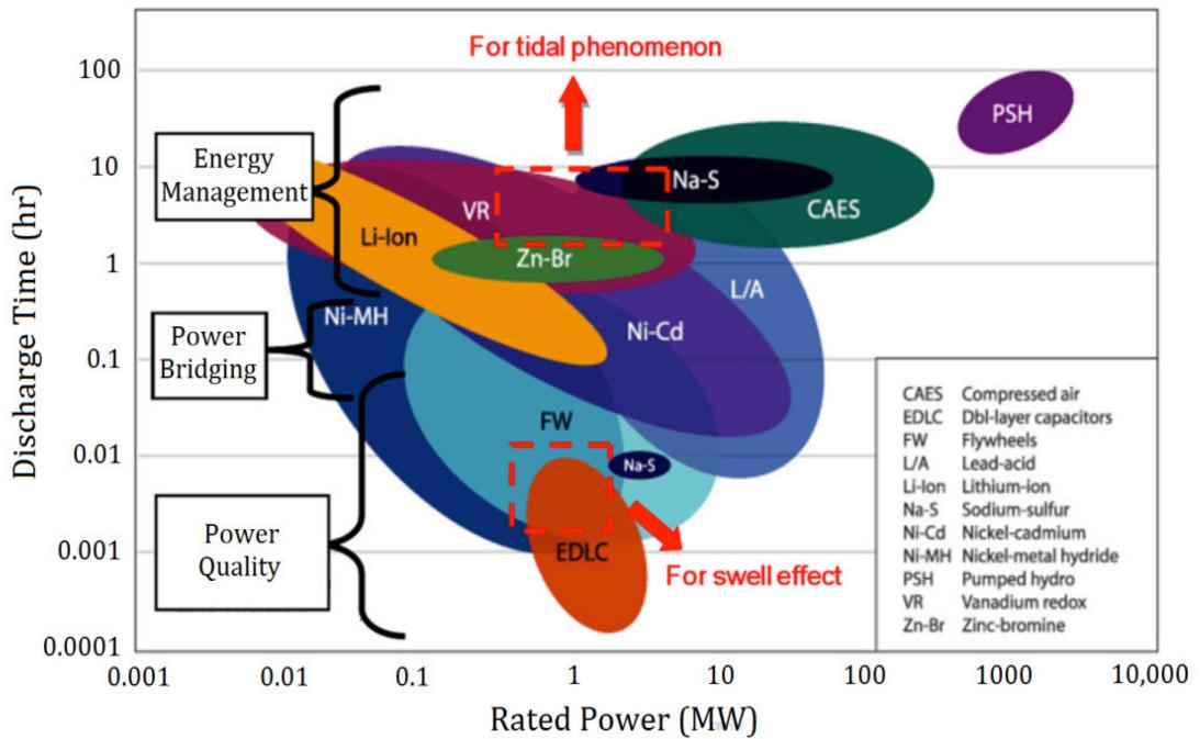
Fig. I.17. System ratings for different energy storage technologies [66].
