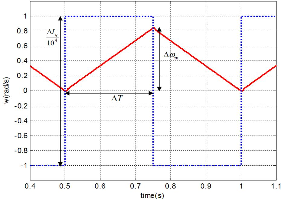
Fig. II.14. Open-loop generator speed response.
