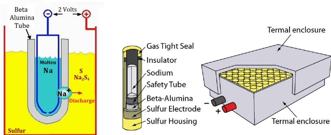
Fig. I.9. NaS battery cell and package [23],[35].
