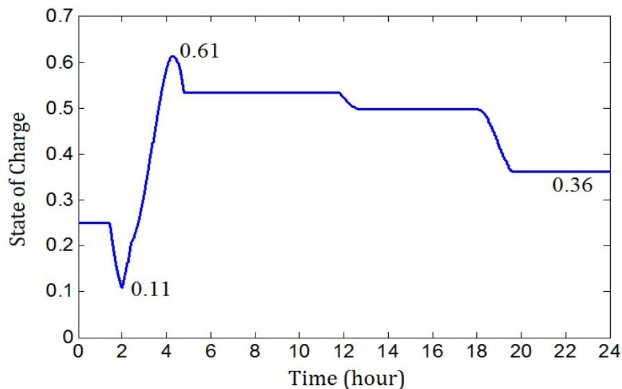
Fig. III.25. SoC of the BESS (initial SoC = 0.25).
