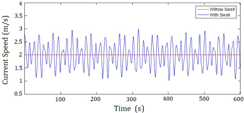
Fig. II.5. Marine current speed under swell effect.
