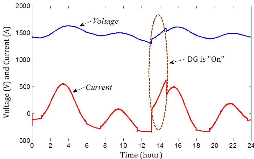
Fig. III.15. Voltage and current of the BESS.
