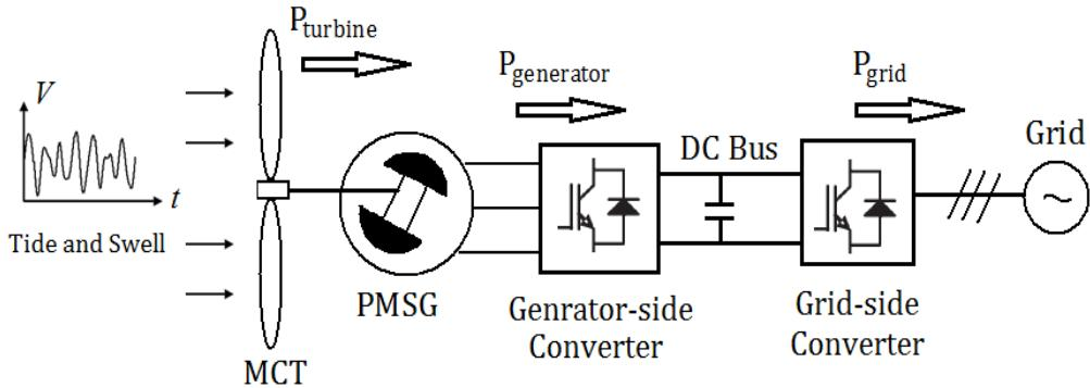
Fig. IV.1. General schema of a PMSG-based direct drive MCT system.
