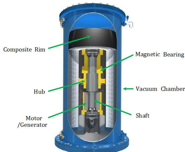
Fig. I.11. Flywheel energy storage device structure [41].
