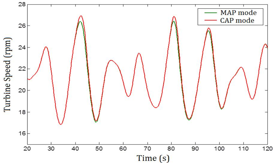
Fig. IV.21. Rotor speed responses under swell effect.
