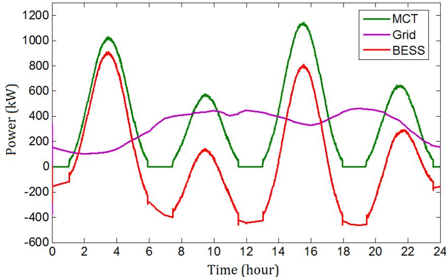
Fig. III.8. Powers of the MCT system with BESS during one day.
