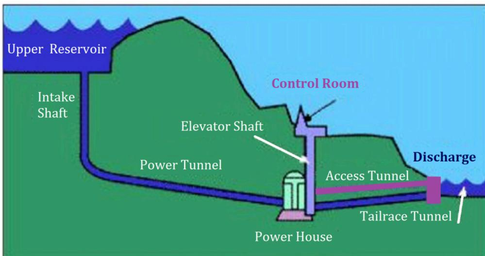
Fig. I.14. Pumped hydro storage plant illustration [64].
