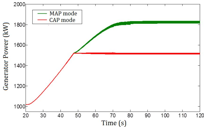
Fig. IV.17. Generator produced power at high tidal speed.
