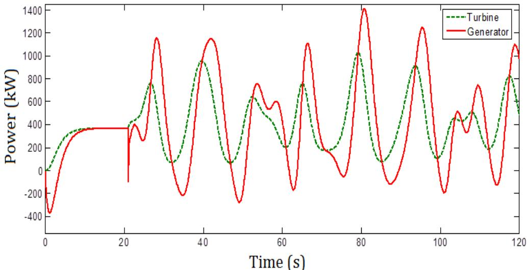
Fig. II.16. Turbine and generator powers with conventional MPPT.
