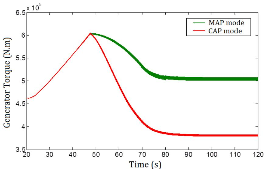
Fig. IV.16. Generator torque responses at high tidal speed.
