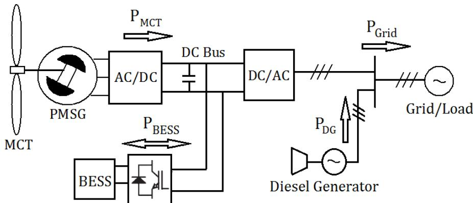
Fig. III.1. General schema for a hybrid MCT/BESS/DG system.
