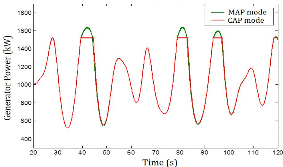
Fig. IV.22. Generator produced power under swell effect.
