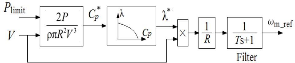
Fig. IV.6. Rotor speed reference at power limitation mode.
