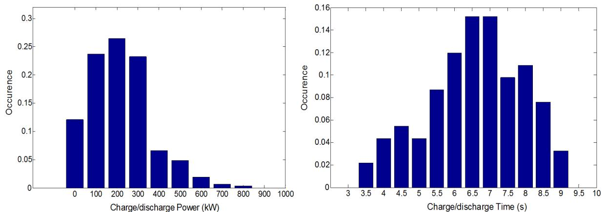
Fig. II.25. Statistical analysis of the ESS charge/discharge characteristics.
