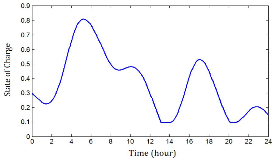
Fig. III.13. SoC of the BESS (initial SoC = 0.3).
