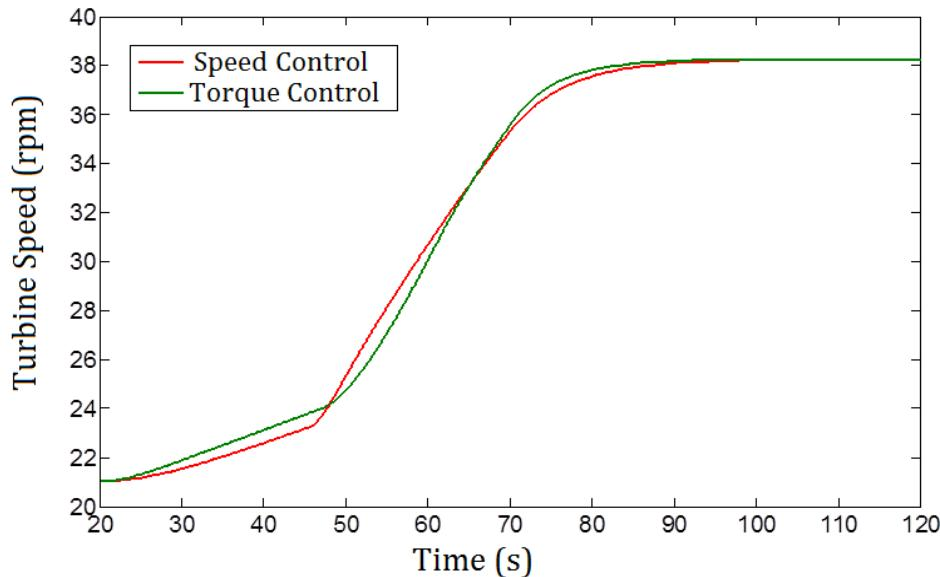
Fig. IV.8. Turbine speed responses at high tidal speed.
