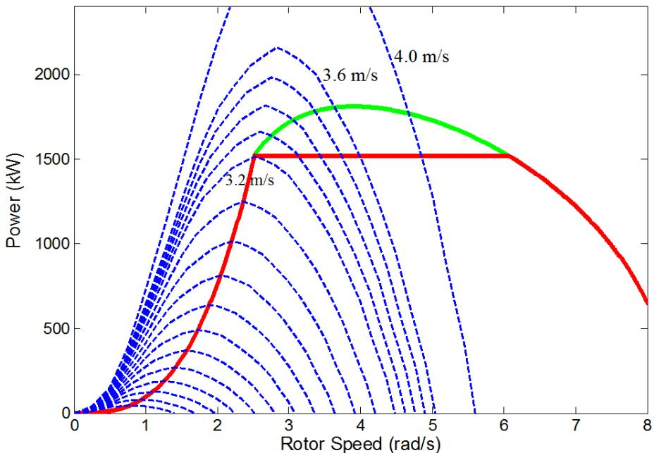
Fig. IV.27. Generator power characteristics with CPSR = 2.4.
