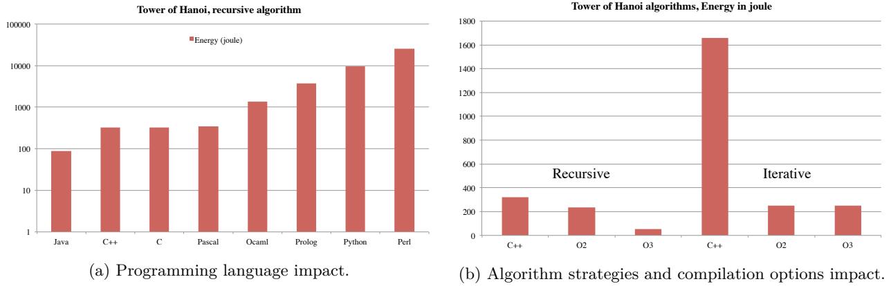
Figure 2.12: Measuring the energy consumption of software.
