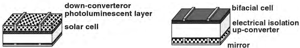
Figure 1.10: (a) solar cell with downconverter added to the front side; (b) solar cell with upconverter on the rear side.
